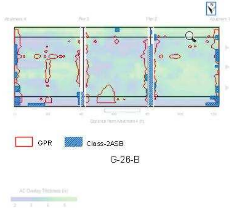
Figure 30: Contour map of asphalt cover overlaid on deck plan with class-2 estimation and as-built data for G-26-B
