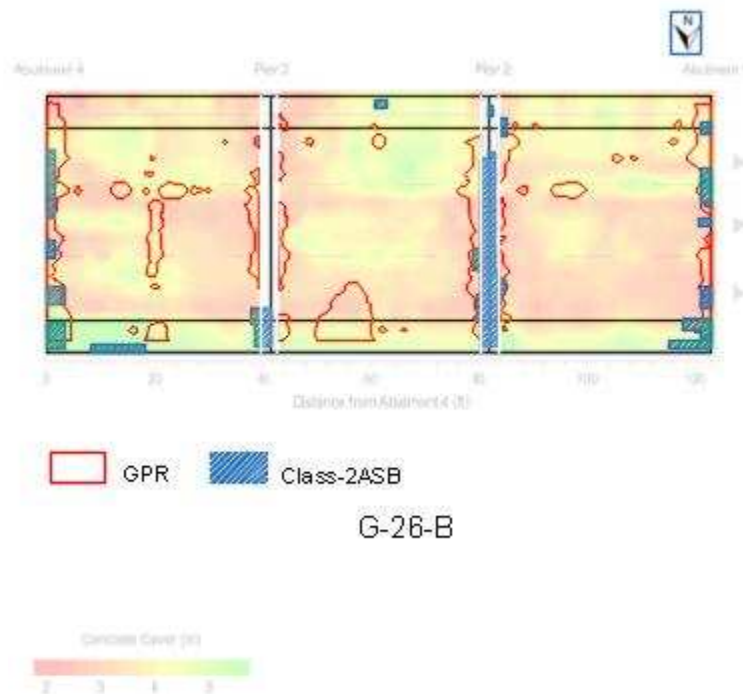
Figure 29: Contour map of concrete cover overlaid on deck plan with class-2 estimation and as-built data for G-26-B
