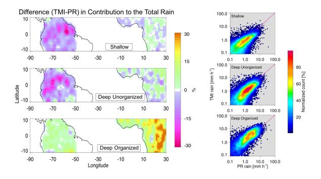
Figure 3.9 Left: The relative difference between PR and PMW total rainfall contribution separated by precipitation regime. Right: Density scatter plots of the PMW and PR rainfall estimates (log-axes) for each of the regimes. In shallow regime (top) PMW sensor underestimates PR by 33%; in deep-unorganized regime (middle) PMW underestimates PR by 10%; in deep-organized regime (bottom) PMW overestimates PR by 41%.
