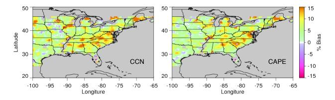
Figure 4.7 Map of improvements in high precipitation rate bias made by using CCN and CAPE environments to complement GPROF algorithm a priori information. Positive values indicate bias improvements.
