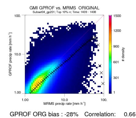
Figure 4.2 Pixel-level comparison of PMW rainfall retrieval (GPROF) and ground reference (MRMS) for the top 10% of rainfall rates over eastern CONUS for period Sep 2014 – Aug 2015. Black crosses represent mean PMW rainfall rate value for corresponding reference rainfall rate bin. The overall bias value for these maximum rain rates is -28%. The correlation coefficient is 0.66.
