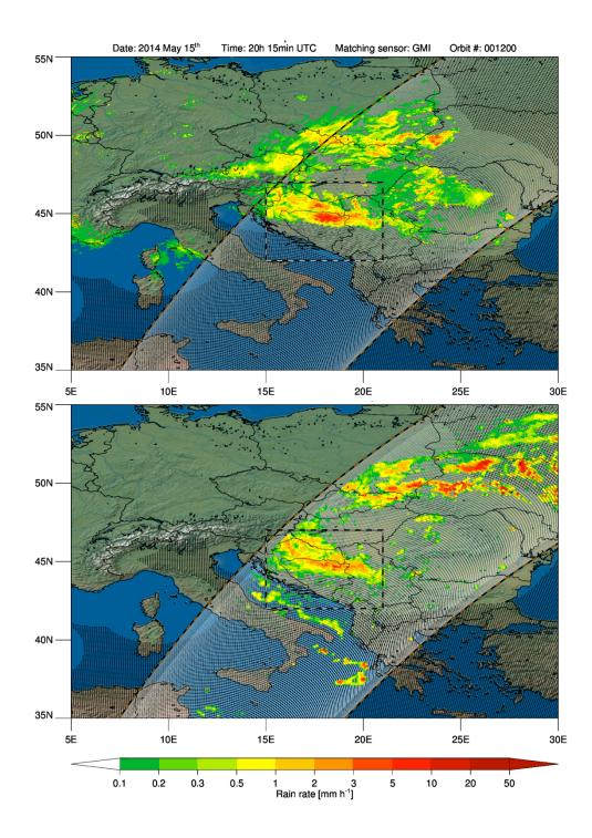
Figure 2.6 *Top:* OPERA composite surface rain rate for 2015 UTC 15 May 2014. Black shading marks radars range; black-white line outlines flood region; white shading with black-yellow limits denote coincided GMI swath. *Bottom:* Corresponding GPROF (GMI orbit 1200) near surface rain rate
