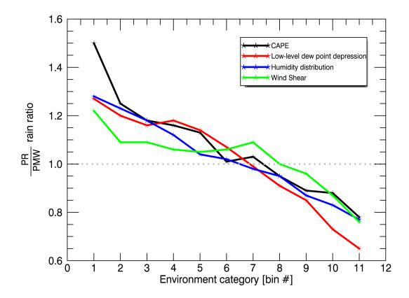
Figure 3.12 PR to PMW rainfall ratio as a function of large-scale environment during the year of 2010. The environmental bins are the same as in Fig. 3.11. The bin limits and exact values of PR to PMW rainfall ratios are listed in Table 3.1.
