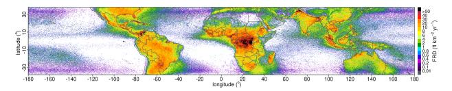
Figure 3.3 The annualized distribution of total (cloud-to-ground plus cloud-to-cloud) lightning activity [flashes km<sup>-2</sup> yr<sup>-1</sup>] detected by the Lightning Imaging Sensor (LIS) Very High Resolution Full Climatology (VHRFC) in period 1998-2013. Source: NASA – Global Hydrological Resource Center (GHRC).
