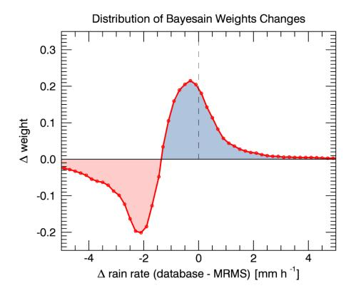
Figure 4.9 Difference in distribution of Bayes mean weights assigned using the original and new, CAPE complemented, a priori information content. The two distributions correspond to the results shown in the first two panels of Fig. 4.6. The differences seen here are associated with 21% reduction of overall rainfall bias (Table 4.4).
