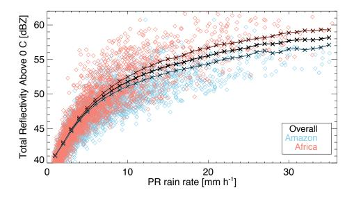
Figure 3.4 Total reflectivity above the freezing level as a function of rain rate. A comparison of the Amazon (blue), African (red) and the overall (black) region (as defined in Fig. 3.1) means. Pixel data are given by diamonds; mean values for each rain rate bin is given by crosses. Note: only 5% randomly chosen pixels are plotted (the means account for full data set) to avoid clutter in the figure.
