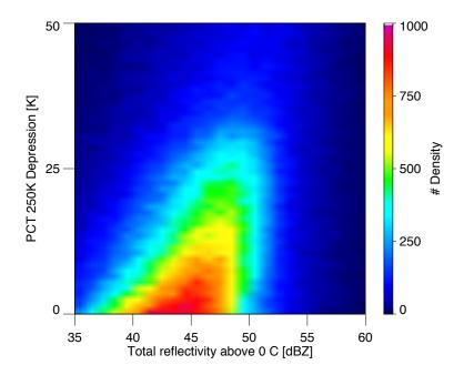
Figure 3.5 Relationship between the total reflectivity above the freezing level (PR) and 85 GHz Tb PCT 250 K depression (TMI).
