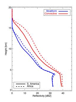
Figure 3.6 Mean PR reflectivity profiles over 4 mm h<sup>-1</sup> 0.5° grid boxes within the two regions marked in Fig. 3.1. Both convective (red) and stratiform (blue) pixels tend to have stronger reflectivity over Africa compared to Amazon.
