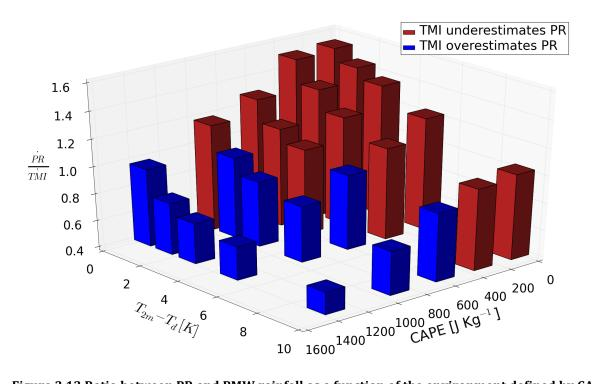
Figure 3.13 Ratio between PR and PMW rainfall as a function of the environment defined by CAPE and the difference between 2m temperature and dew point. Red bars denote bins where PR rainfall is underestimated by PMW retrieval, while blue bars denote the opposite.
