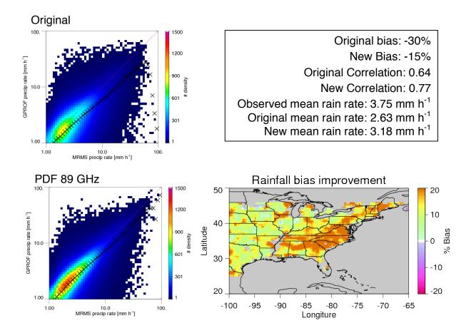
Figure 5.1 Performance of GPROF retrieval when 89 GHz Tb PDF is used to complement the *a priori* information content. Defined using eight 20-degree bins the PDF complements the *a priori* infromation via arbitrarily criterion where scenes of Tb PDFs differencing by more than 20% from that of the observed one are ignored.
