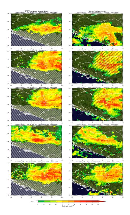
Figure 2.7 *Left column:* OPERA composite surface rain rates over the flood region at the time of the closest overpasses of SSMIS (onboard F16, F17, F18), GMI and AMSR2 sensors, with corresponding orbit numbers: 54532, 38821, 23567, 1200, and 10586, respectively. Shaded in white: region with no valid radar retrieval. *Right column:* corresponding GPROF near surface rain rates.
