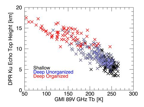
Figure 4.4 Mean cloud top height as a function of mean 89 GHz GMI brightness temperature over 1° x 1° scenes over the CONUS for period Sep 2014 through Aug 2015. The height is estimated using DPR Ku echo top heights. Three colors identify regime type.
