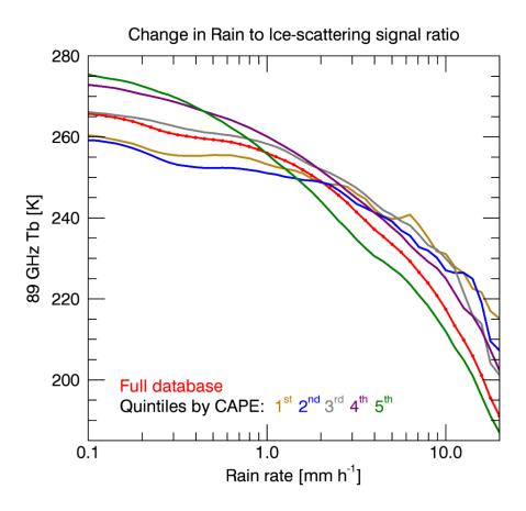
Figure 4.5 Mean relationship between the ice aloft and surface rainfall rate for the full dataset (red line) and five equally populated distinct CAPE environmental subsets (yellow, blue, gray, purple and green). Correlation coefficient for each line is given in Table 4.1.
