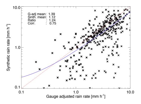
Figure 2.12 Relationship between gauge-adjusted and synthetically retrieved rain rates for six SSMIS-F18 overpasses during the flooding event. Blue line is a linear fit of approximately 2500 rain rates, while red line denotes one to one ratio.
