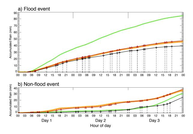
Figure 2.8 Timelines of the area mean rainfall accumulations for the Balkan flood (panel a) and the nonflood (panel b) event. Satellite estimate is given in *black* with symbols marking the individual sensors overpasses; *Red* - OPERA observations at the time of satellite overpass only; *Yellow* - OPERA observations in full temporal and spatial resolution; *Green* - OPERA gauge-adjusted observations in full temporal and spatial resolution (adjusted Z-R relationship is given in Table 2.3).
