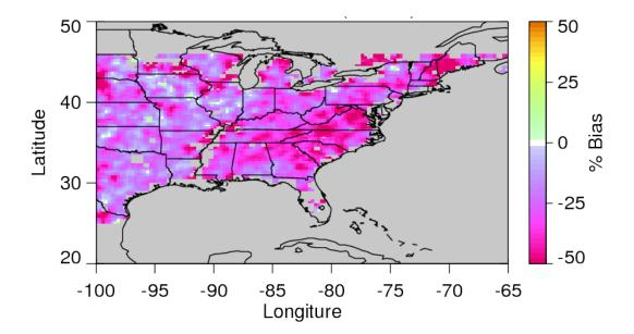
Figure 4.1 Mean rainfall bias between a ground reference (MRMS) and PMW retrieval (GPROF) for the top 10% of rainfall rates over eastern CONUS for period Sep 2014 – Aug 2015 on 0.25° grid. The mean MRMS observed rainfall rate for the period is 3.98 mm h<sup>-1</sup> while the mean PMW retrieved rainfall rate is 2.87 mm h<sup>-1</sup>. The overall bias is -28% (Negative values in the map indicate satellite's retrieval underestimation of the ground reference.).
