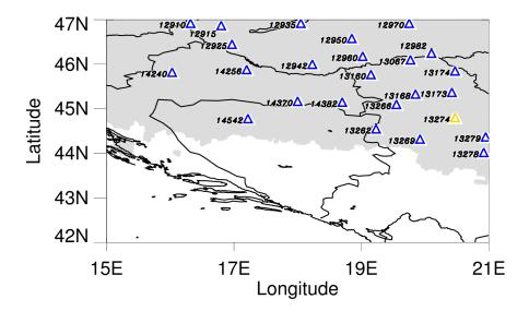
Figure 2.2 Flood region with radar coverage (in gray) and distribution of ground rain gauges (blue triangles labeled by station's WMO IDs) used in the analysis. Yellow marker indicates sounding location.
