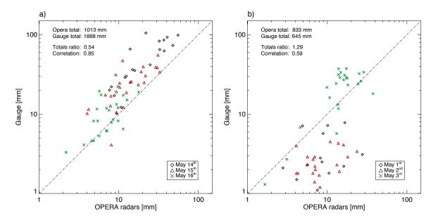
Figure 2.4 Comparison between 25 gauge and OPERA 24-hour rainfall accumulations (diamonds – May 14<sup>th</sup>, triangles – May 15<sup>th</sup>, crosses – May 16<sup>th</sup>) in the Balkan flood event – *panel a*, and in the average (non-flood) 3-day period (May 1<sup>st</sup> – 3<sup>rd</sup>) – *panel b*. Note log-axes on both plots.
