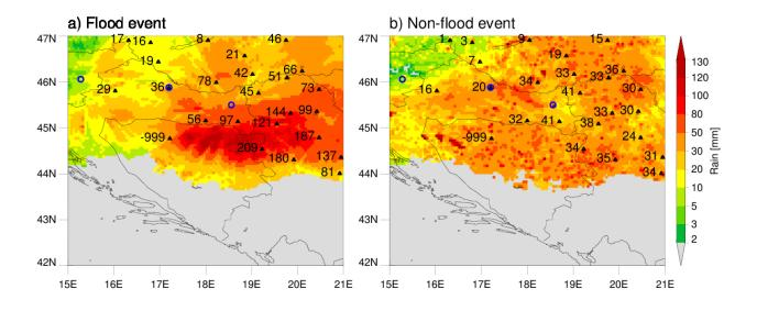
Figure 2.3 A 3-day rainfall accumulations over the flood region for the Balkan flood event (May  $1^{4th} - 16^{th}$ ) – (a), and the average (non-flood) 3-day period (May  $1^{st} - 3^{rd}$ ) – (b). Color bar corresponds to the OPERA measurements; ground rain gauges readings are labeled next to their locations (black triangles) with more details in Table 2.2; blue circles point radar locations.
