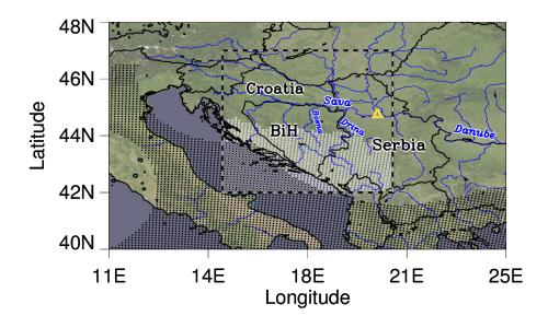
Figure 2.1 Balkan peninsula. Boxed area marks the flood region limits. Shadings denote OPERA network coverage: *shaded in black* - areas beyond radar range, *shaded in white* - no radar coverage due to beam blockage of high terrain. River names are given in blue. Yellow marker indicates sounding location.
