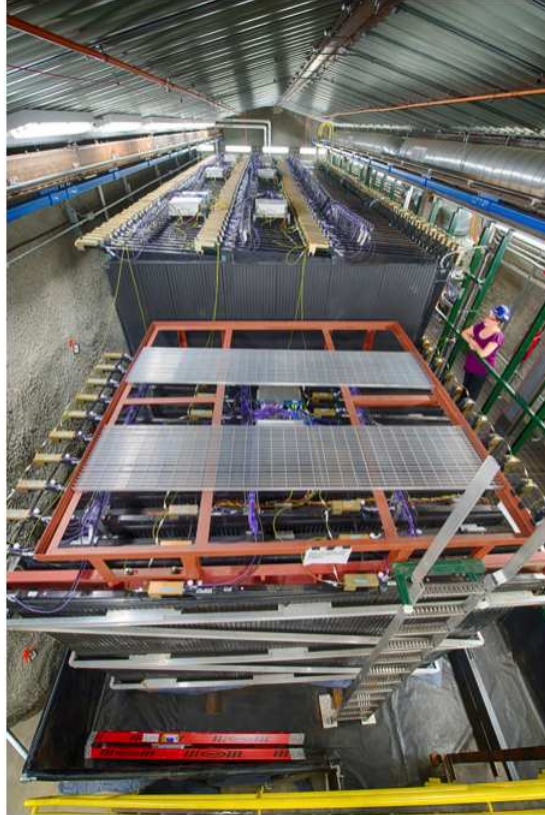
Figure 2.15: A photograph of the muon catcher seated at the downstream end of the NO \nu A near detector. The beam is directed toward the camera in this photo.
