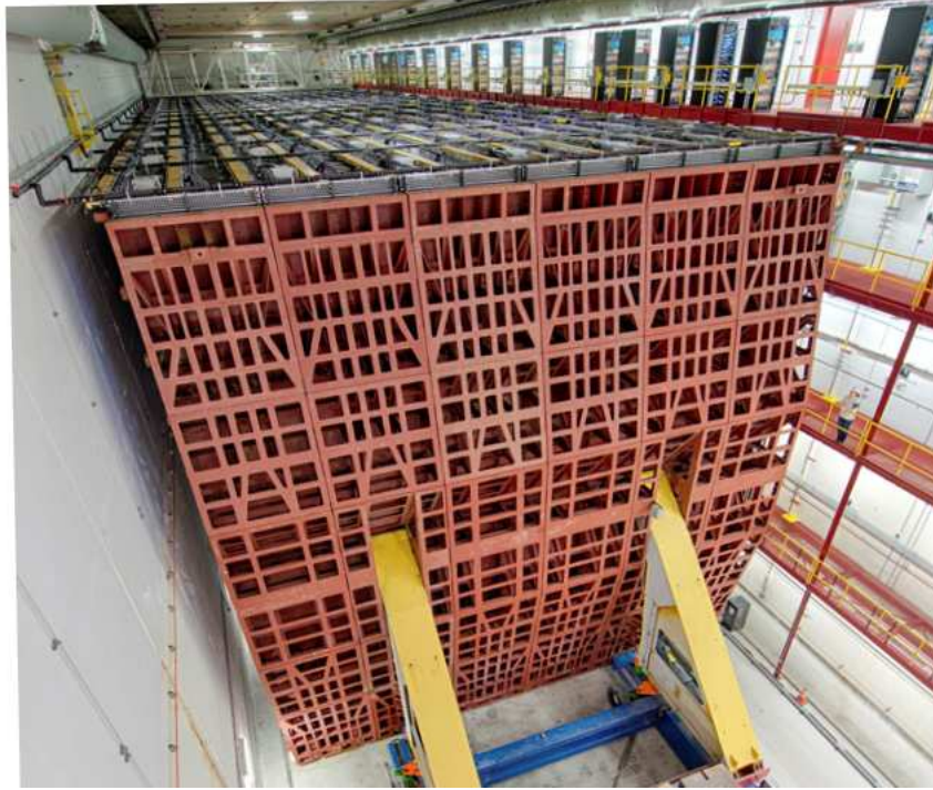
Figure 2.13: A photograph of the NOνA far detector. The far detector height and width are 15.6 m long. The detector is 63.0 m long. The beam direction is away from the camera in this photo.
