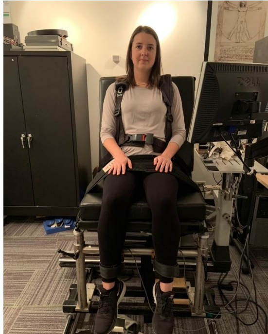
Bilateral knee extension maximal voluntary contraction and rate of force development experimental apparatus.
