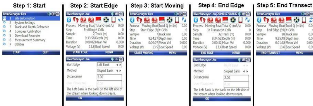
Figure 5. Five steps in completing a discharge measurement
