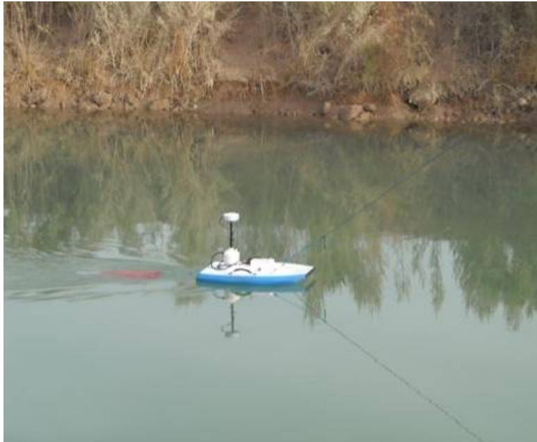
Figure 4. SonTek RiverSurveyor assembled on SonTek Hydroboard
