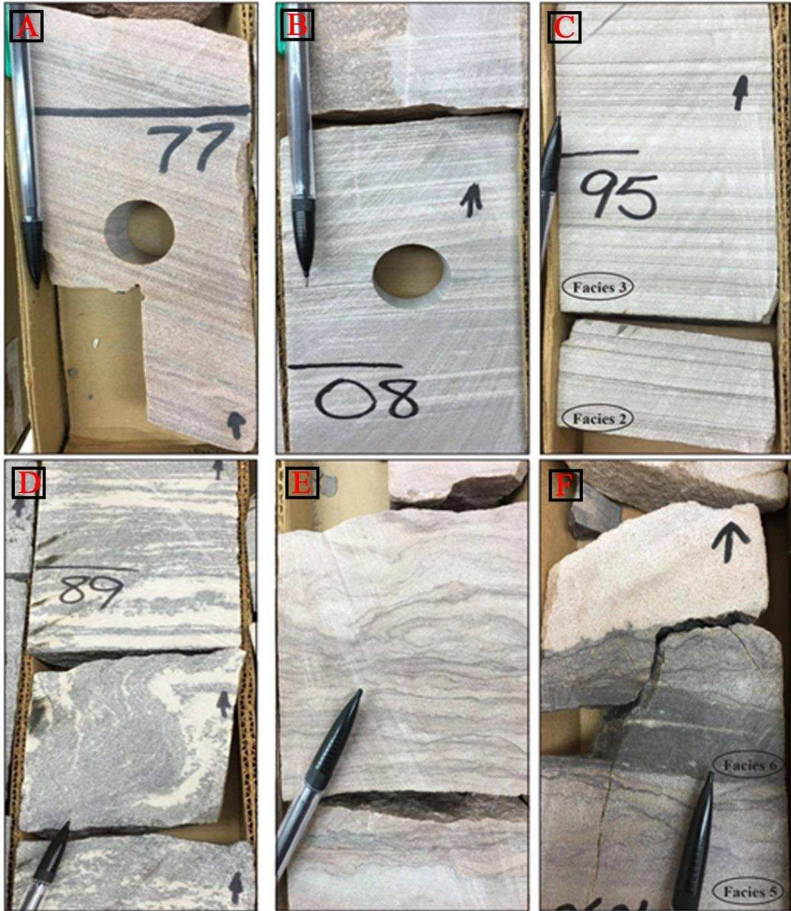
Figure 5. Facies of the Lyons Formation. (A) Core photograph of high-angle cross-laminated sandstone (Facies 1) (Coquina Oil Berthoud State 2, 4977 ft). (B) Core photograph showing low-inclined cross-laminated sandstone (Facies 2) (Tiger Oil Wadleigh 34-21, 7808 ft). (C) Core photograph illustrating horizontally-laminated sandstone facies is overlying low-inclined cross-laminated facies (Facies 3) (Tiger Oil Wadleigh 34-21, 7795 ft). (D) Core photograph of chaotically-bedded to folded sandstone (Facies 4) (Viking Petroleum Cactus Hill 2, 8989 ft) (E) Core photograph showing wavy- to irregularly-laminated silty sandstone (Facies 5) (Coquina Oil Berthoud State 2, 4992 ft). (F) Core photograph illustrating massive to wavy-laminated silt-rich mudstone (Facies 6) is overlying wavy to irregularly-laminated silty sandstone (Facies 5) (Amoco Production Champlin 410, 8526 ft).
