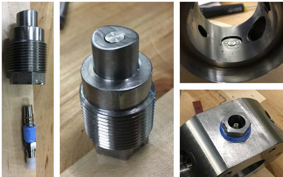
Figure 5. Kistler 601CAA piezoelectric pressure transducer and adapter plug. Pictured outside of its adapter housing (left), fully assembled (center), and mounted to combustion chamber (right).
