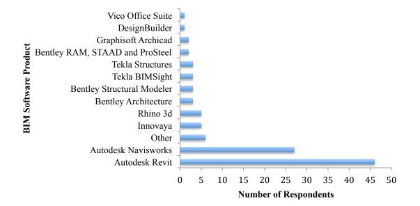
Figure 6: Most common BIM software programs used by respondent companies
