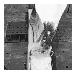
Figure 1.3 Yield and Buckling pattern in a Reduced Beam Section
