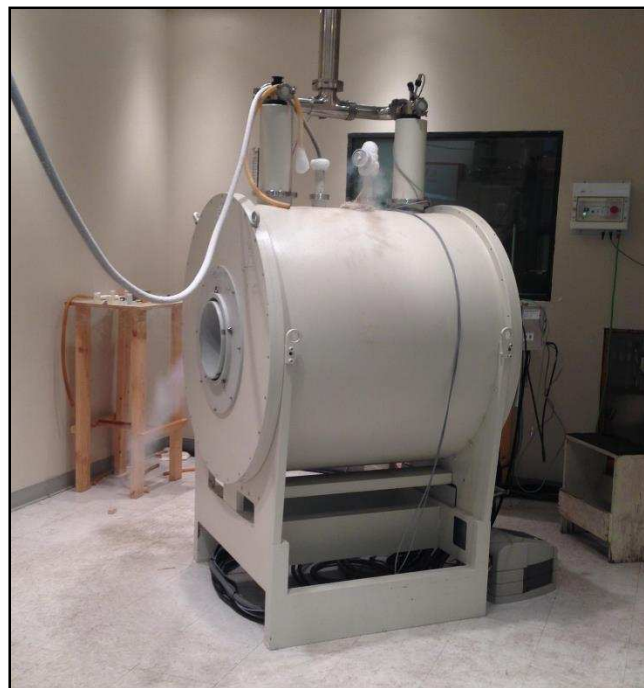
Figure 4.11. Bruker small-animal MRI scanner with 2.3 Tesla (100 MHz) at RMMRC, CSU.
