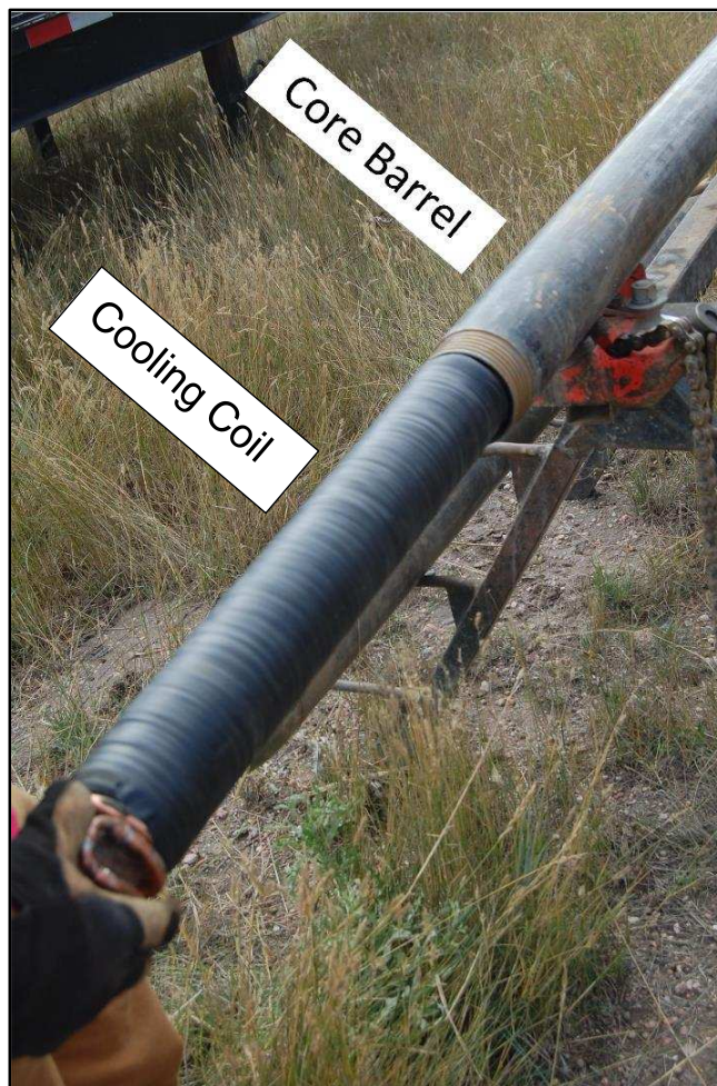
Figure A-2. Photo showing the insulated cooling coil being inserted into the core barrel.
