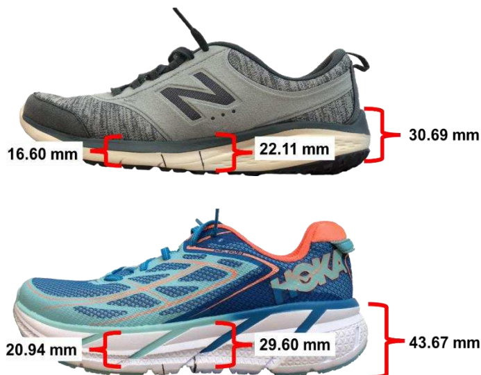
Figure 2. Measurements of the midsole were taken at the heel, midfoot, and forefoot. The New Balance 85v1 ( TOP ) serves as the standard cushioned midsole. Weight = 216 grams. IMEVA foam midsole. The Hoka One One Clifton 3 ( BOTTOM ) serves as the high cushioned midsole. Weight = 204 grams. ProFly EVA midsole.
