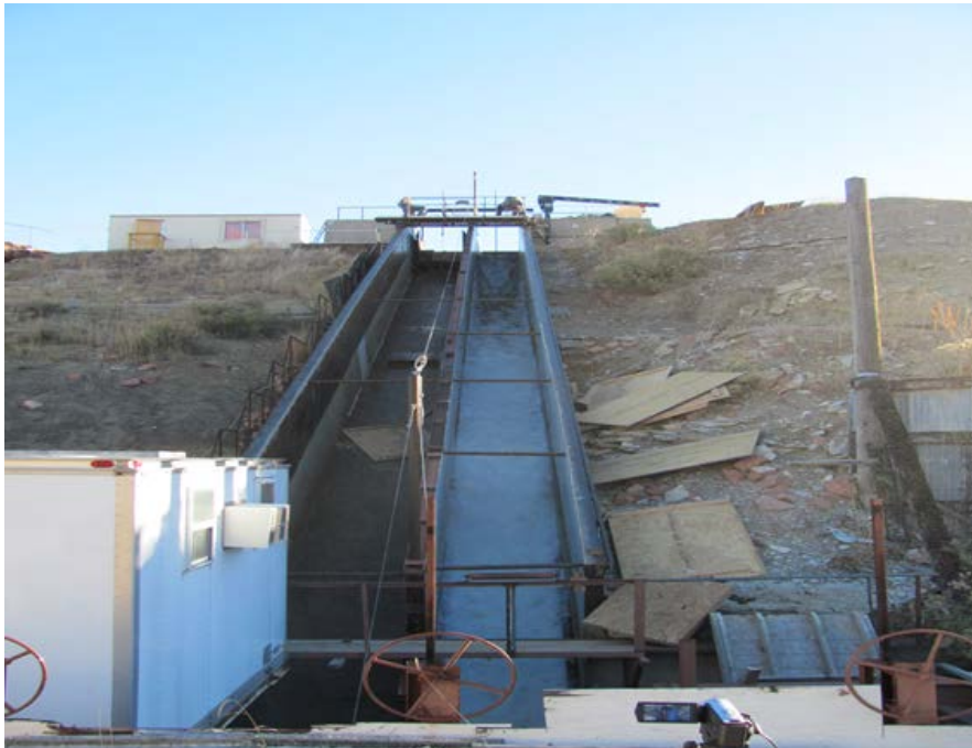
Figure 1. Fixed Slope Test Flume at Colorado State University
