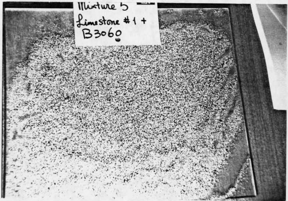
Picture B-13. No clear segregation of mixture #5 from above
