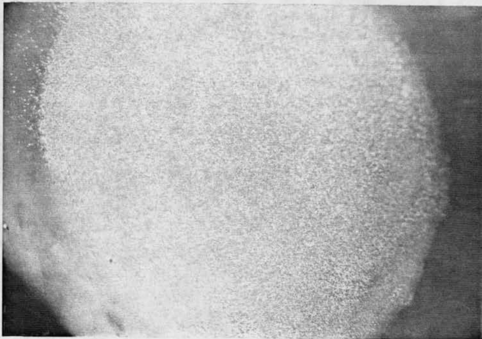
Picture B-20. White particles on bottom from mixture #9 (view underneath)
