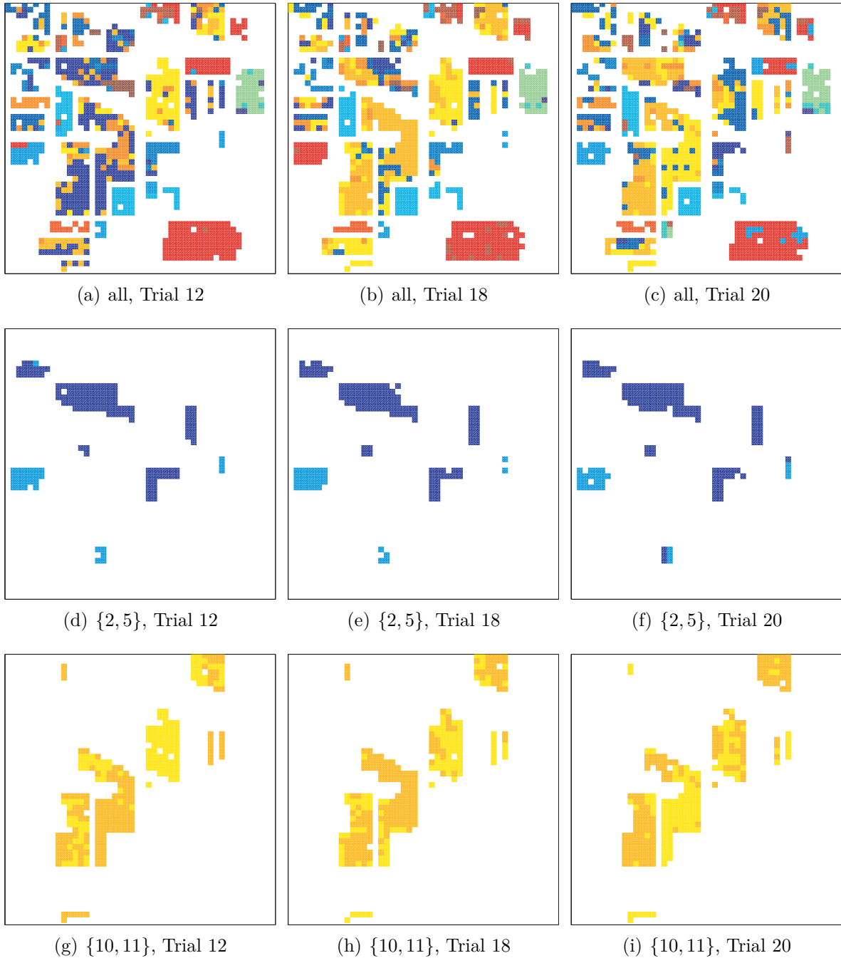
FIGURE 4.3. Example Indian Pines classifications using PCA-generated subspace models ( a = 1 ). Tiles are color coded by the best class (detector) using the same scale as in Figure 4.2(a).
