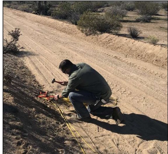
Figure 9-2. John Boyle installing an electrode into the ground for Survey A, along the road. 11/26/18.
