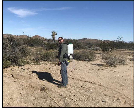
Figure 9-6. John Boyle utilizing the 5-Gallon backpack sprayer with salt-water solution to saturate electrodes in order to improve contact resistance. 11/26/18.
