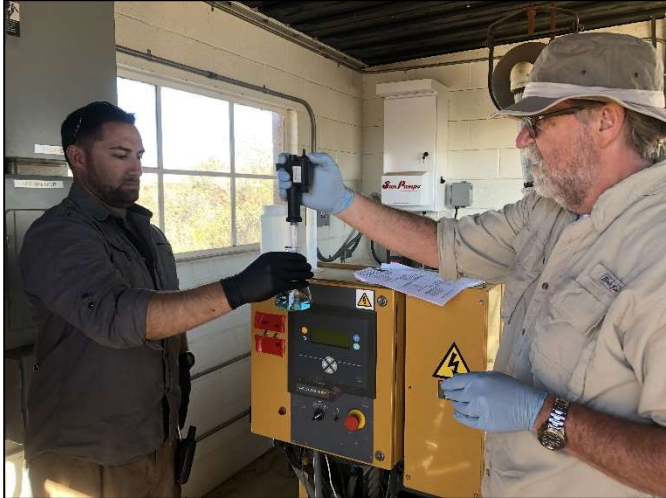
Figure 9-19. John Boyle (left) and Dr. William Sanford (right) using Hach Method 8203 to determine alkalinity of LUB-23 well water. 11/28/18.
