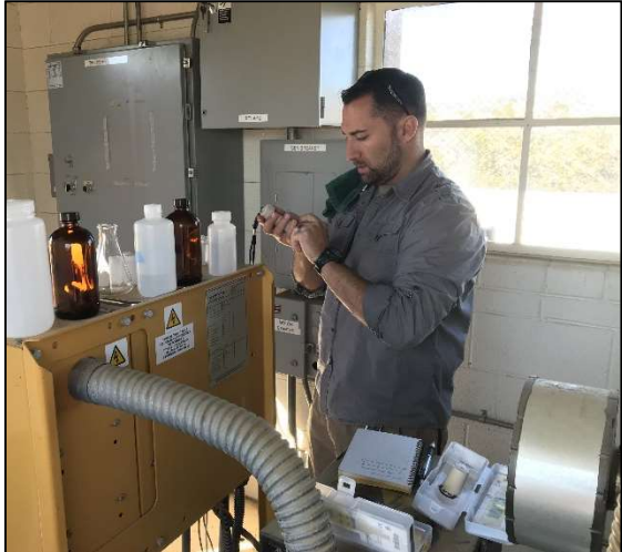
Figure 9-20. John Boyle using the Oakton multi-parameter PC Testr-35 to measure pH, conductance, water temperature, and dissolved oxygen of LUB-23 well water. 11/28/18.
