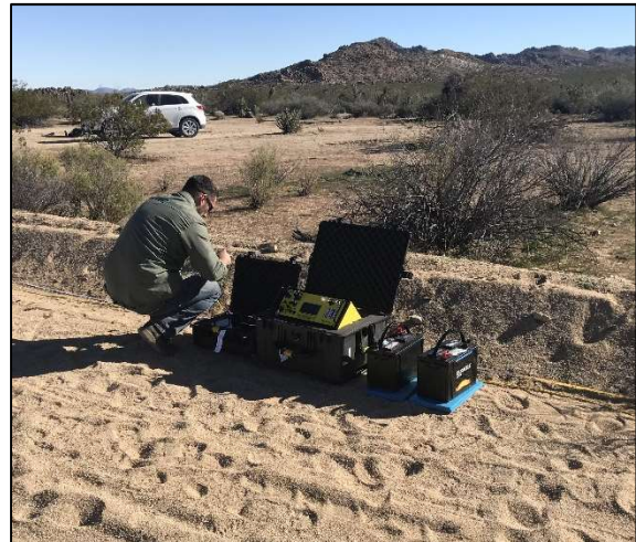
Figure 9-4. John Boyle setting up the AGI Supersting™ at the center point of Array 1 of Survey A along the road. 11/26/18.
