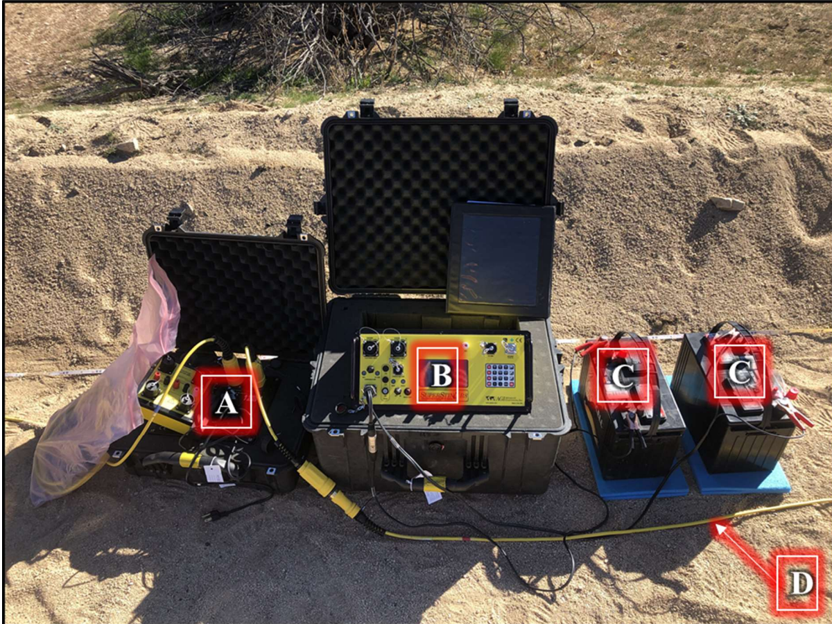
Figure 3-1a. Equipment Layout. (A) ERT Switch Box, (B) ERT Supersting™ R8, (C) 2x Deep Cycle Marine Batteries, (D) 4x ERT Electrode (10m spacing) Land Cables.
