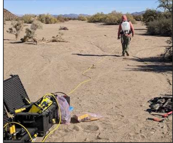
Figure 9-9. Tyler Gilkerson using the 5-gallon backpack sprayer to saturate the electrodes to help improve contact resistance for Survey B.
