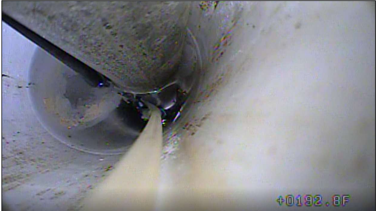
Figure 9-16. Camera screenshot inside LUB-23 at a spool length of 192.8 ft. Notice the water level just below the camera. The precise reading at that water level is 193.18 ft from spool or 190.78 ft bgs.
