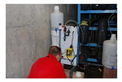
Figure 10 - Injection Pump Connected to Tracer Solution
