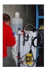
Figure 5 - Pump Attached to DI Water for Calibration
