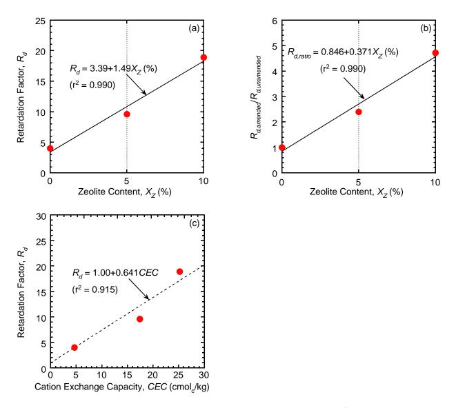
Figure 5.60. Effect of amount of zeolite on retardation of potassium (K<sup>+</sup>) for backfills with 0 (unamended), 5 and 10 % chabazite-LB permeated with 35 mM KCl: (a) retardation factor ( $R_d$ ); (b) ratio of  $R_d$  for the zeolite-amended backfill relative to  $R_d$  for the unamended backfill ( $R_{d,amended}/R_{d,unamended}$ ); (c) cation exchange capacity (*CEC*) of backfill and  $R_d$  of K<sup>+</sup>.
