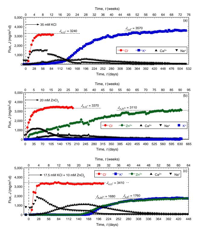
Figure 5.20. Temporal trends in effluent solute flux for columns of backfills amended with 5 % chabazite-UB and permeated with different salt solutions: (a) 35 mM KCl (Test No. 3); (b) 20 mM ZnCl<sub>2</sub> (Test No. 4); (c) 17.5 mM KCl plus 10 mM ZnCl<sub>2</sub> (Test No. 5).
