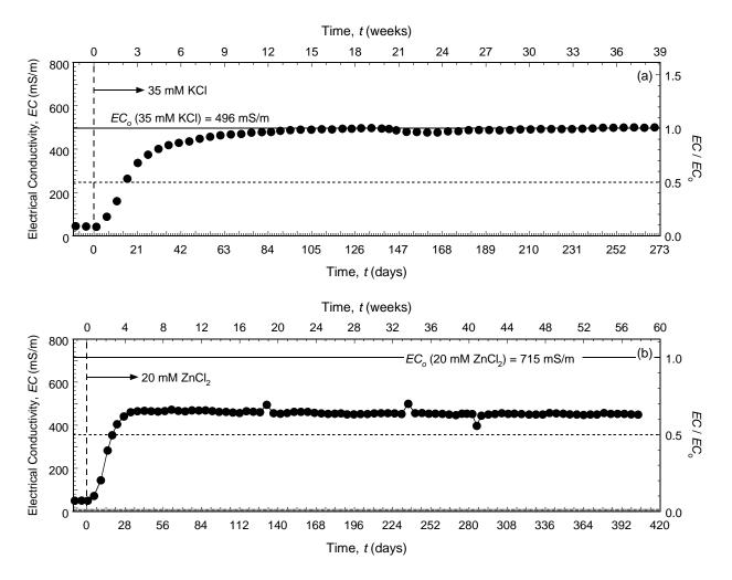
Figure 5.27. Temporal trends in the electrical conductivity of the effluent for columns with unamended backfills permeated with different salt solutions: (a) 35 mM KCl (Test No. 1); (b)  $20 \text{ mM ZnCl}_2$  (Test No. 2).
