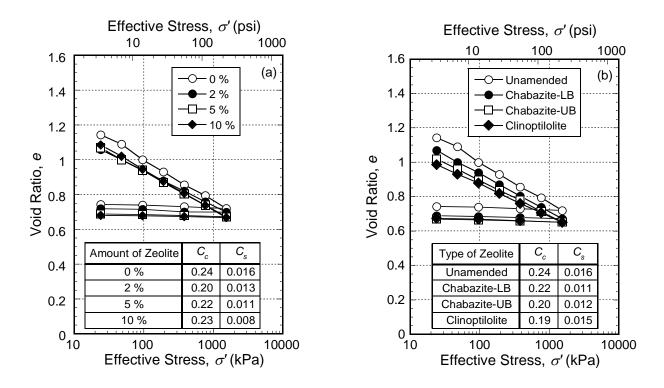
Figure 2.3. Stress-strain curves for confined compression of unamended and zeolite-amended backfills: (a) effect of different amounts of the same zeolite (chabazite-LB); (b) effect of same amount (5 %) of different types of zeolite.  $C_c$  = compression index;  $C_s$  = swell index.
