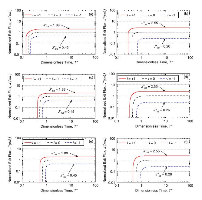
Figure E.15. Effect of Péclet number,  $P_L$ , on flux breakthrough curves with a constant source concentration,  $C_o = 10,000 \text{ mg/L}$  for: (a) unamended with potassium (K); (b) unamended with zinc (Zn); (c) amended with 5 % clinoptilolite with potassium (K); (d) amended with 5 % clinoptilolite with zinc (Zn); (e) amended with 10 % clinoptilolite with potassium (K); (f) amended with 10 % clinoptilolite with zinc (Zn), all based on the Freundlich adsorption model.
