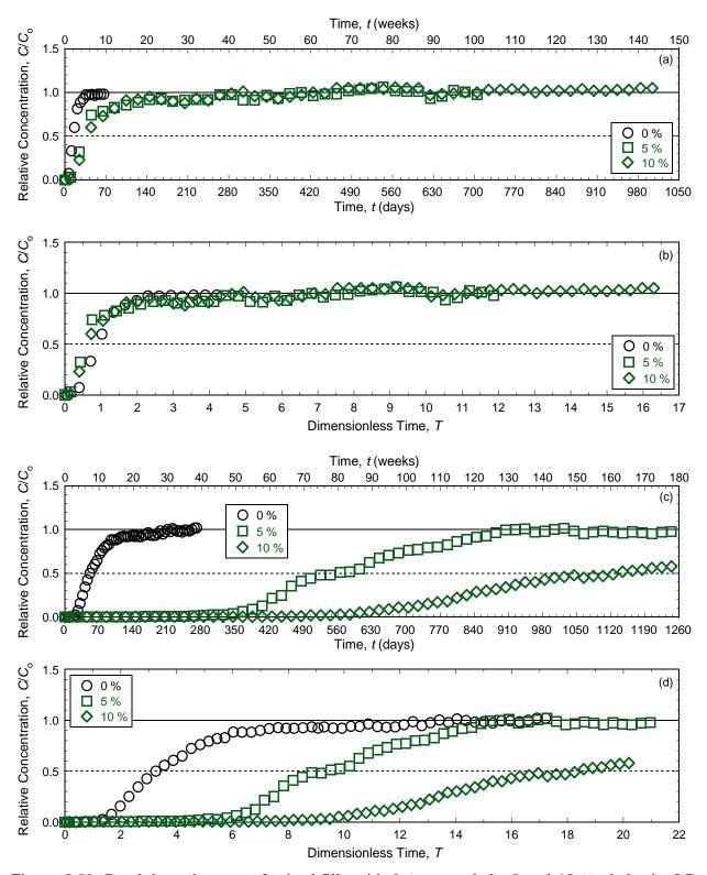
Figure 5.59. Breakthrough curves for backfills with 0 (unamended), 5 and 10 % chabazite-LB permeated with 35 mM KCl: (a) chloride (Cl<sup>-</sup>) versus time (*t*); (b) Cl<sup>-</sup> versus dimensionless time (*T*); (c) potassium (K<sup>+</sup>) versus *t*; (d) K<sup>+</sup> versus *T*.
