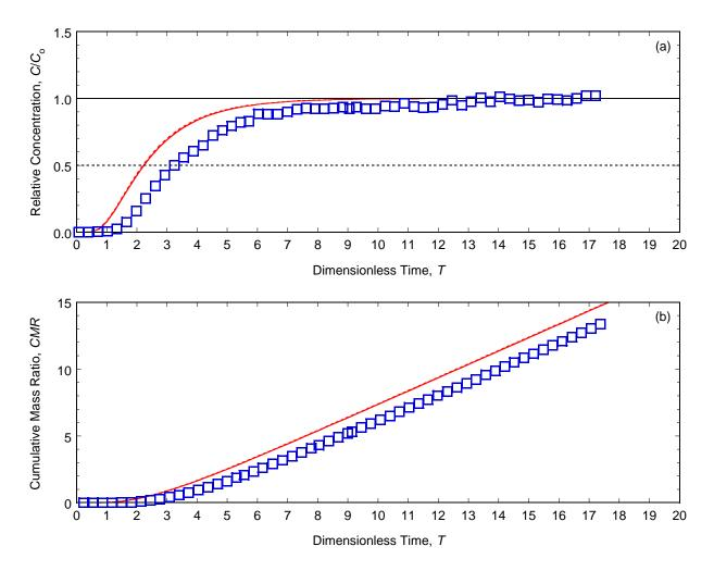
Figure F.1. Comparison of the measured column effluent data for potassium (K<sup>+</sup>) versus the model simulation using  $R_d$  based on the BEAT results and  $P_L$  from regression of the measured column effluent data for the unamended backfill permeated with 35 mM KCl (Test No. 1): (a) relative concentration (*RC*) data; (b) cumulative mass ratio (*CMR*) data. Note: dashed line =  $R_d$  based on Freundlich adsorption model; solid line =  $R_d$  based on Langmuir adsorption model.
