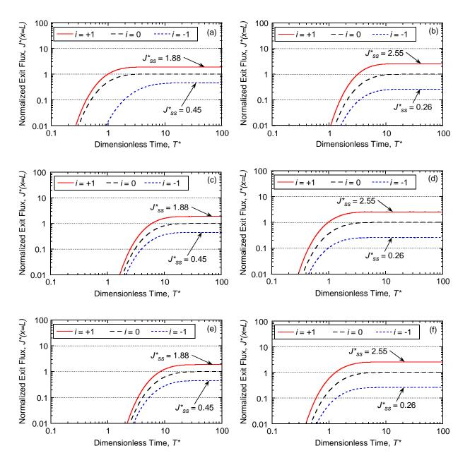
Figure E.10. Effect of Péclet number,  $P_L$ , on flux breakthrough curves with a constant source concentration,  $C_o = 100 \text{ mg/L}$  for: (a) unamended with potassium (K); (b) unamended with zinc (Zn); (c) amended with 5 % chabazite-UB with potassium (K); (d) amended with 5 % chabazite-UB with zinc (Zn); (e) amended with 10 % chabazite-UB with potassium (K); (f) amended with 10 % chabazite-UB with zinc (Zn), all based on the Langmuir adsorption model.
