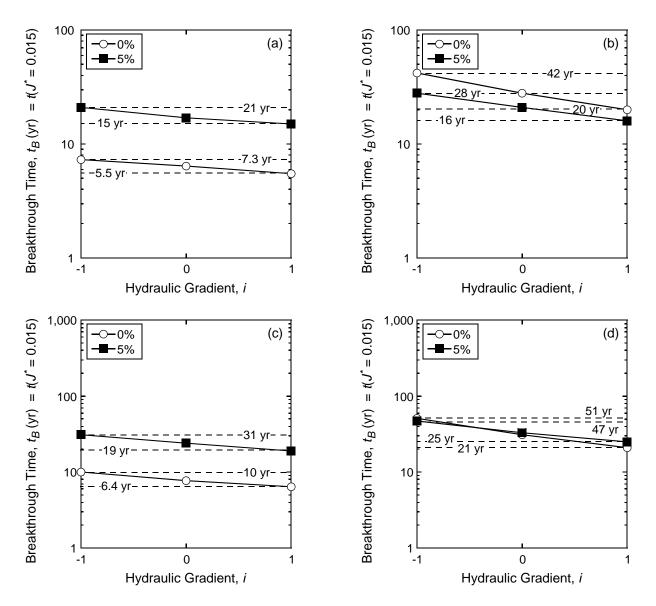
Figure E.27. Relationship between Péclet number,  $P_L$ , and predicted flux breakthrough times corresponding to  $J^*(x = L) = 0.015$  with a constant source concentration ( $C_o$ ) of 10,000 mg/L for the unamended and zeolite-amended cutoff wall with 5 % clinoptilolite: (a) potassium (K), Langmuir; (b) zinc (Zn), Langmuir; (c) potassium (K), Freundlich; (d) zinc (Zn), Freundlich.
