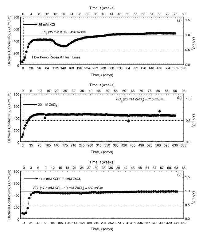
Figure 5.28. Temporal trends in the electrical conductivity of the effluent from columns of backfills amended with 5 % chabazite-UB permeated with different salt solutions: (a) 35 mM KCl (Test No. 3); (b) 20 mM ZnCl<sub>2</sub> (Test No. 4); (c) 17.5 mM KCl plus 10 mM ZnCl<sub>2</sub> (Test No. 5).
