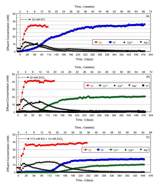
Figure 5.17. Temporal trends in effluent solute concentrations for columns of backfills amended with 5 % clinoptilolite and permeated with different salt solutions: (a) 35 mM KCl (Test No. 6); (b) 20 mM ZnCl<sub>2</sub> (Test No. 7); (c) 17.5 mM KCl plus 10 mM ZnCl<sub>2</sub> (Test No. 8).
