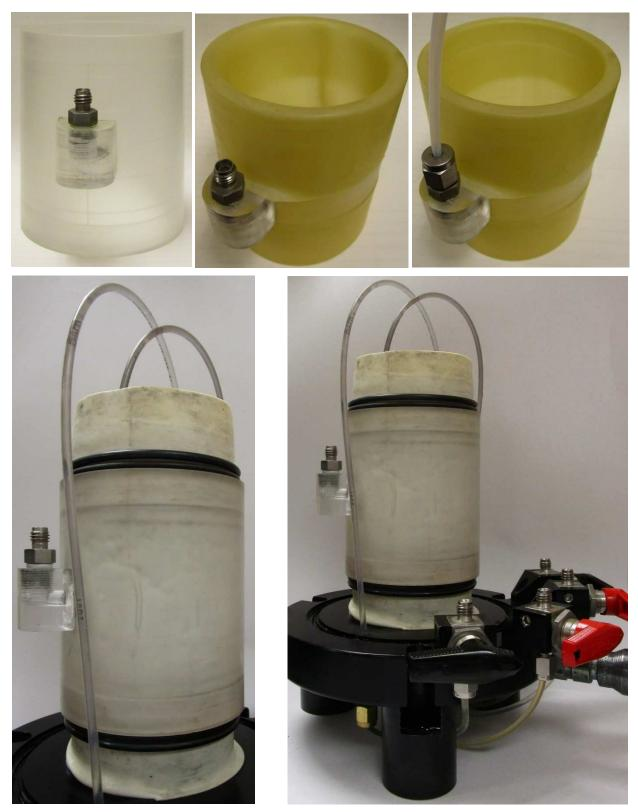
Figure A.2. Pictorial view of the acrylic cylinder used for the flexible-wall setup.
