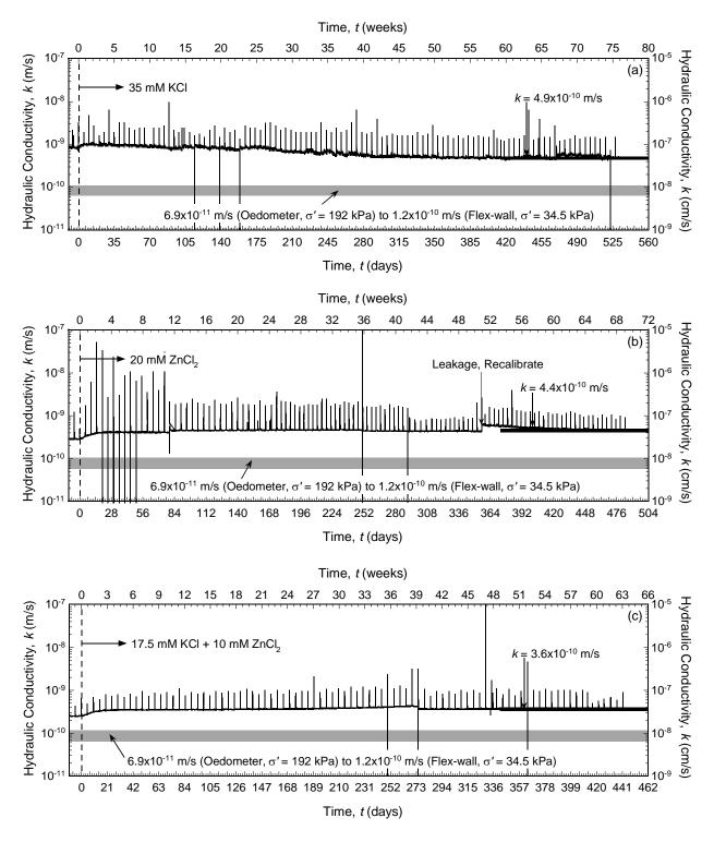
Figure 5.12. Temporal trends in hydraulic conductivity for columns of backfills amended with 5 % clinoptilolite and permeated with different salt solutions: (a) 35 mM KCl (Test No. 6); (b) 20 mM ZnCl<sub>2</sub> (Test No. 7); (c) 17.5 mM KCl plus 10 mM ZnCl<sub>2</sub> (Test No. 8).
