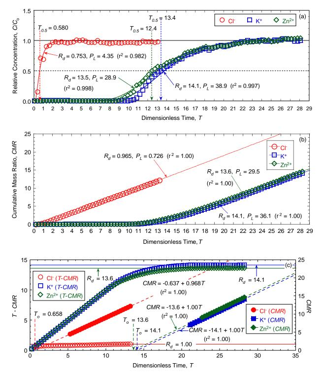
Figure 5.40. Chemical transport analyses for determination of column Péclet number ( $P_L$ ) and/or retardation factor ( $R_d$ ) for backfill amended with 5 % chabazite-UB and permeated with 17.5 mM KCl plus 10 mM ZnCl<sub>2</sub> (Test No. 5): (a) regression of relative concentration (RC) data; (b) regression of cumulative mass ratio (CMR) data; (c)  $T_o$  (=  $R_d$ ) and T - CMR analyses for  $R_d$ .
