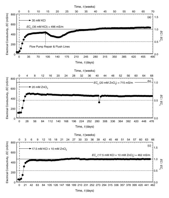
Figure 5.29. Temporal trends in the electrical conductivity of the effluent for columns of backfills amended with 5 % clinoptilolite permeated with different salt solutions: (a) 35 mM KCl (Test No. 6); (b) 20 mM ZnCl<sub>2</sub> (Test No. 7); (c) 17.5 mM KCl plus 10 mM ZnCl<sub>2</sub> (Test No. 8).
