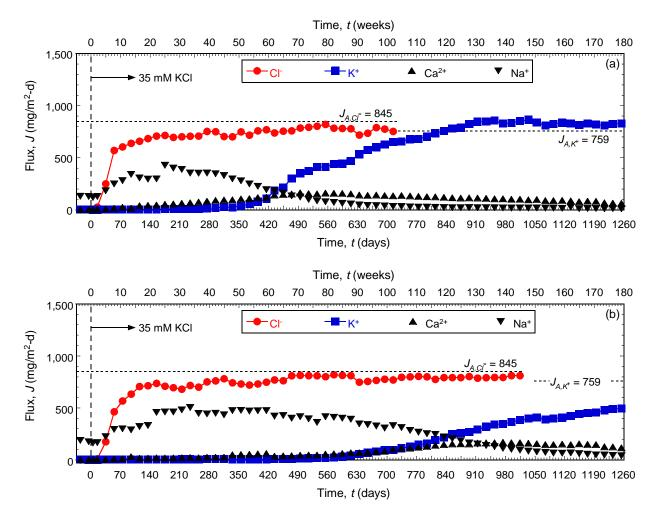
Figure 5.22. Temporal trends in effluent solute flux for columns of backfills amended with different amounts of chabazite-LB and permeated with a solution of 35 mM KCl: (a) 5 % chabazite-LB (Test No. 9); (b) 10 % chabazite-LB (Test No. 10).
