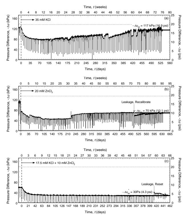
Figure 5.7. Temporal trends in pressure differences across columns of backfills amended with 5 % chabazite-UB and permeated with different salt solutions: (a) 35 mM KCl (Test No. 3); (b) 20 mM ZnCl<sub>2</sub> (Test No. 4); (c) 17.5 mM KCl plus 10 mM ZnCl<sub>2</sub> (Test No. 5).
