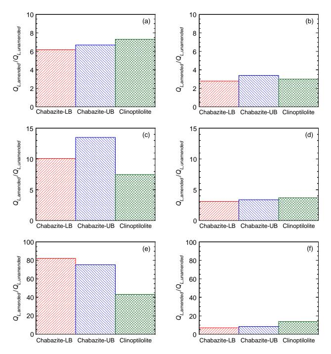
Figure 3.13. Comparison of the ratio of the maximum adsorption capacity  $(Q_L)$  of the zeoliteamended backfill sorbents  $(Q_{L,amended})$  relative to the  $Q_L$  of the unamended backfill sorbent  $(Q_{L,unamended})$  for different types of zeolite: (a) K with 5 % zeolite; (b) Zn with 5 % zeolite; (c) K with 10 % zeolite; (d) Zn with 10 % zeolite; (e) K with 100 % zeolite; (f) Zn with 100 % zeolite.
