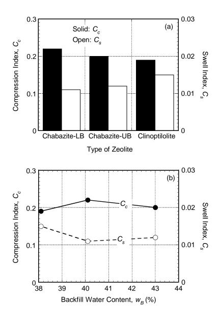
Figure 2.9. Compression and swell indices for zeolite-amended backfills amended with the same amount (5 %) of different types of zeolites: (a) effect of type of zeolite; (b) effect of backfill water content.
