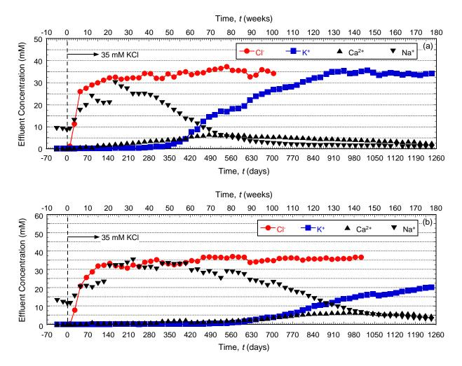
Figure 5.18. Temporal trends in effluent solute concentrations for columns of backfills amended with different amounts of chabazite-LB and permeated with a solution of 35 mM KCl: (a) 5 % chabazite-LB (Test No. 9); (b) 10 % chabazite-LB (Test No. 10).
