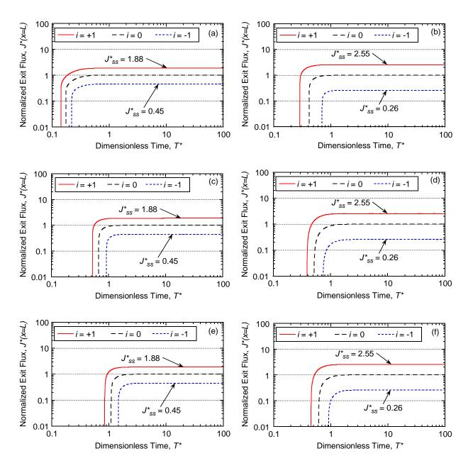
Figure E.9. Effect of Péclet number,  $P_L$ , on flux breakthrough curves with a constant source concentration,  $C_o = 10,000 \text{ mg/L}$  for: (a) unamended with potassium (K); (b) unamended with zinc (Zn); (c) amended with 5 % chabazite-UB with potassium (K); (d) amended with 5 % chabazite-UB with zinc (Zn); (e) amended with 10 % chabazite-UB with potassium (K); (f) amended with 10 % chabazite-UB with zinc (Zn), all based on the Freundlich adsorption model.
