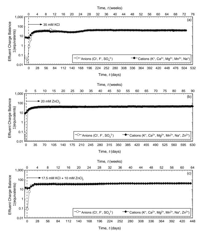
Figure 5.24. Temporal trends in effluent charge balance for columns of backfills amended with 5 % chabazite-UB and permeated with different salt solutions: (a) 35 mM KCl (Test No. 3); (b) 20 mM ZnCl<sub>2</sub> (Test No. 4); (c) 17.5 mM KCl plus 10 mM ZnCl<sub>2</sub> (Test No. 5). [Note: absolute values for the  $\Sigma$ anion equivalents are shown].
