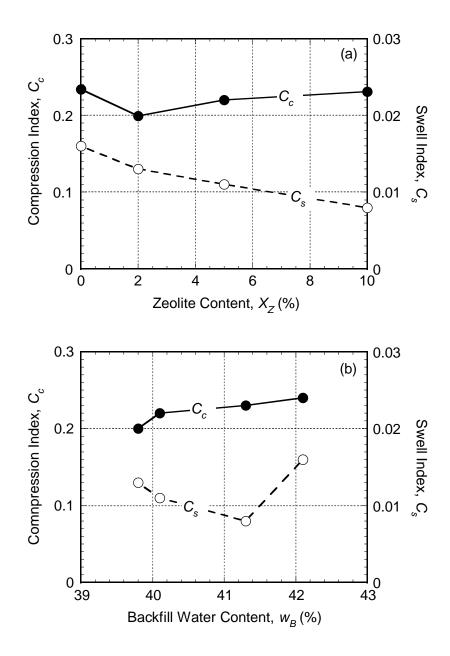
Figure 2.8. Compression and swell indices for unamended backfill and zeolite-amended backfills amended with the same zeolite (chabazite-LB): (a) effect of amount of zeolite; (b) effect of backfill water content.
