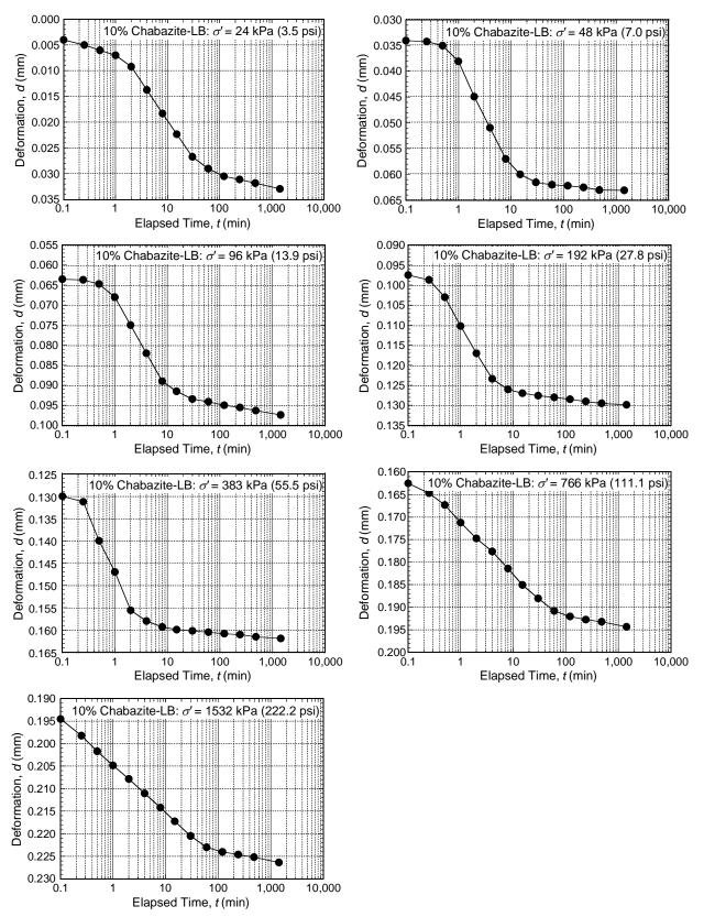
Figure A.11. Results of settlement as a function of log time for SB backfill amended with 10 % chabazite-LB.
