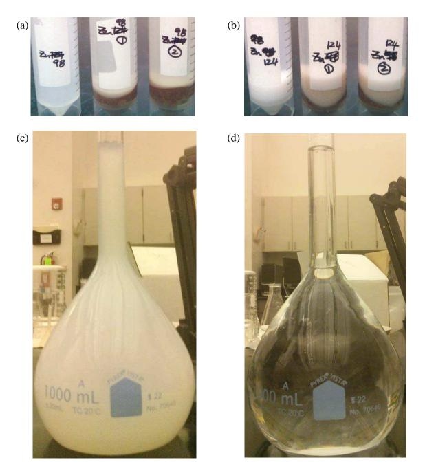
Figure 3.1. Formation of precipitation in zinc chloride solution: (a) after batch test for source concentration of 98 mM without acid addition; (b) after batch test for source concentration of 124 mM without acid addition; (c) stock solution with target concentration of 200 mM before acid addition (pH 5.27); (d) stock solution with target concentration of 200 mM after addition of 1 mL of 37 % HCl (pH 2.76).
