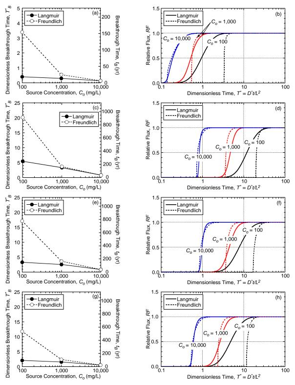
Figure 4.17. Effect of constant potassium source concentration ( $C_o$ ) on the dimensionless barrier breakthrough times,  $T_B^*$  (a, c, e) for f = 0.05 and flux breakthrough curves (b, d, f) for unamended and zeolite-amended backfills: (a) & (b) unamended; (c) & (d) 10 % chabazite-LB-amended; (e) & (f) 10 % chabazite-UB-amended; (g) & (h) 10 % clinoptilolite-amended.
