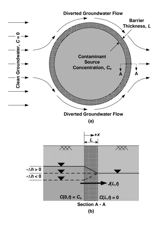
Figure 4.1. Schematic of soil-bentonite vertical cutoff wall scenarios for model simulations: (a) plan view showing divergent groundwater flow; (b) cross-sectional view of cutoff wall illustrating boundary conditions.
