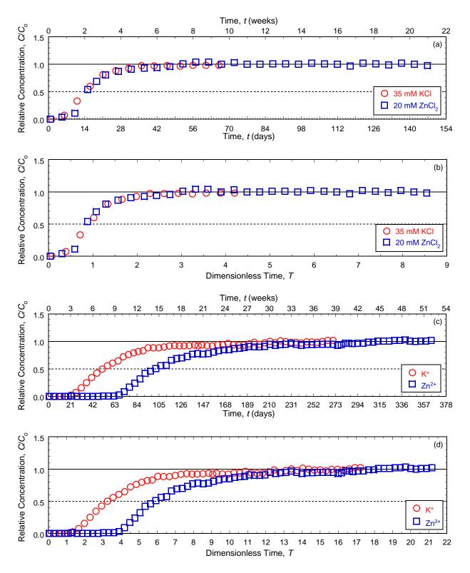
Figure 5.62. Breakthrough curves for unamended backfill permeated with 35 mM KCl or 20 mM ZnCl<sub>2</sub>: (a) chloride (Cl<sup>-</sup>) versus time (*t*); (b) Cl<sup>-</sup> versus dimensionless time (*T*); (c) potassium (K<sup>+</sup>) and zinc (Zn<sup>2+</sup>) versus *t*; (d) K<sup>+</sup> and Zn<sup>2+</sup> versus *T*.
