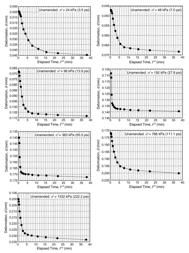
Figure A.6. Results of settlement as a function of square root elapsed time for the unamended SB backfill.
