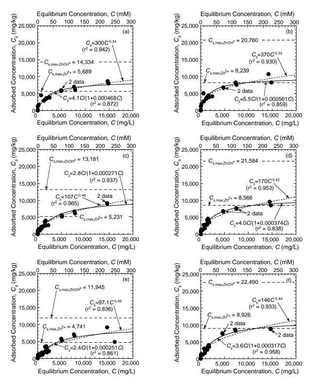
Figure 3.5. Fitted Freundlich (dashed line) and Langmuir (solid line) adsorption models for zinc (Zn) adsorption to zeolite-amended backfill sorbents: (a) 5 % chabazite-LB; (b) 10 % chabazite-LB; (c) 5 % chabazite-UB; (d) 10 % chabazite-UB; (e) 5 % clinoptilolite; (f) 10 % clinoptilolite.
