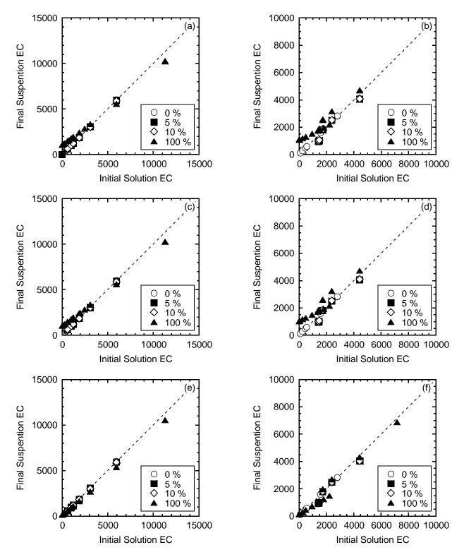
Figure B.2. Change in initial solution EC after the experiments for the unamended, zeoliteamended and 100 % zeolite: (a) chabazite-LB for  $K^+$ ; (b) chabazite-LB for  $Zn^{2+}$ ; (c) chabazite-UB for  $K^+$ ; (d) chabazite-UB for  $Zn^{2+}$ ; (e) clinoptilolite for  $K^+$ ; (f) clinoptilolite for  $Zn^{2+}$ .
