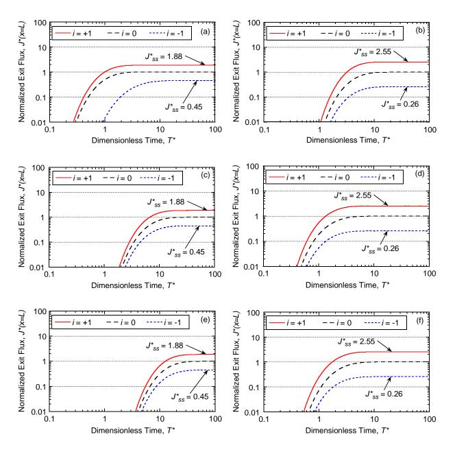
Figure E.4. Effect of Péclet number,  $P_L$ , on flux breakthrough curves with a constant source concentration,  $C_o = 100 \text{ mg/L}$  for: (a) unamended with potassium (K); (b) unamended with zinc (Zn); (c) amended with 5 % chabazite-LB with potassium (K); (d) amended with 5 % chabazite-LB with zinc (Zn); (e) amended with 10 % chabazite-LB with potassium (K); (f) amended with 10 % chabazite-LB with zinc (Zn), all based on the Langmuir adsorption model.
