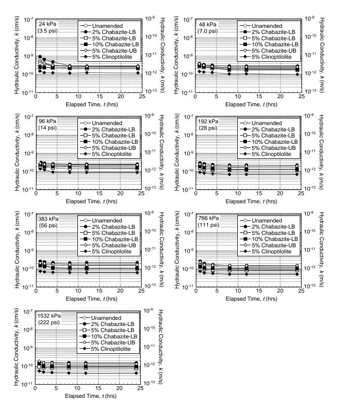
Figure A.4 Measured hydraulic conductivity in fixed-ring oedometer cells as a function of elapsed time for each unamended and zeolite-amended soil-bentonite backfills prepared at 125-mm slumps at different consolidation effective stress ( $\sigma$ ).
