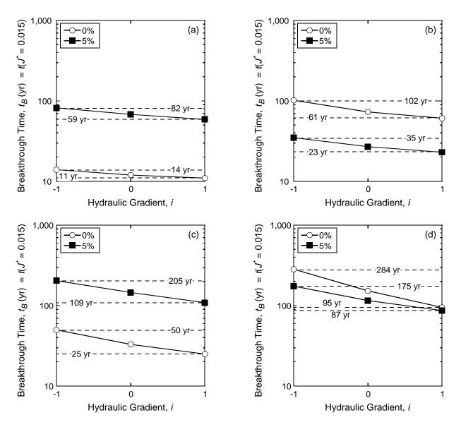
Figure E.23. Relationship between Péclet number,  $P_L$ , and predicted flux breakthrough times corresponding to  $J^*(x = L) = 0.015$  with a constant source concentration ( $C_o$ ) of 1,000 mg/L for the unamended and zeolite-amended cutoff wall with 5 % chabazite-UB: (a) potassium (K), Langmuir; (b) zinc (Zn), Langmuir; (c) potassium (K), Freundlich; (d) zinc (Zn), Freundlich.
