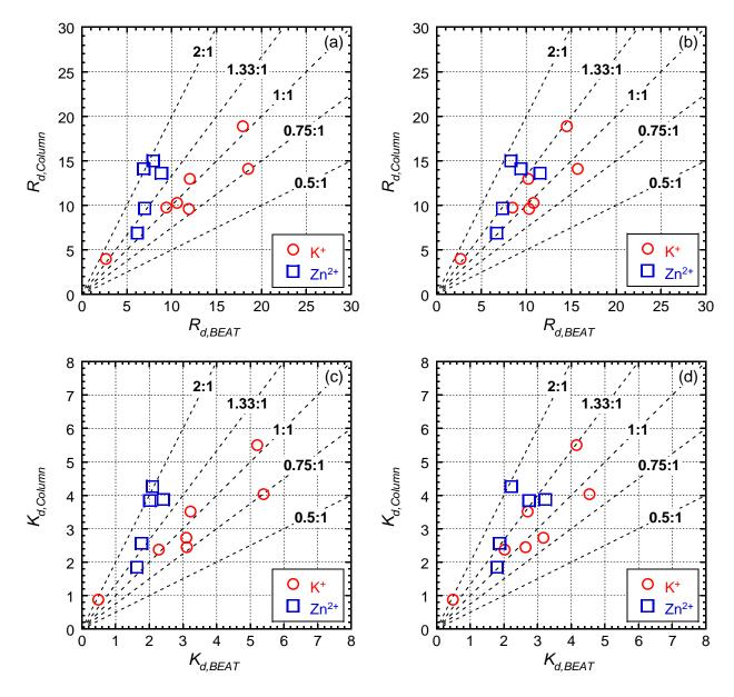
Figure 5.50. Comparison of the retardation factor  $(R_d)$  and distribution coefficient  $(K_d)$  based on the *CMR* regression to the column test and batch equilibrium adsorption tests (BEATs): (a)  $R_{d,BEAT}$  (Langmuir model) versus  $R_{d,Column}$ ; (b)  $R_{d,BEAT}$  (Freundlich model) versus  $R_{d,Column}$ ; (c)  $K_{d,BEAT}$  (Langmuir model) versus  $K_{d,Column}$ ; (d)  $K_{d,BEAT}$  (Freundlich model) versus  $K_{d,Column}$ .
