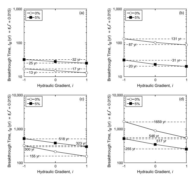
Figure E.25. Relationship between Péclet number,  $P_L$ , and predicted flux breakthrough times corresponding to  $J^*(x = L) = 0.015$  with a constant source concentration ( $C_o$ ) of 100 mg/L for the unamended and zeolite-amended cutoff wall with 5 % clinoptilolite: (a) potassium (K), Langmuir; (b) zinc (Zn), Langmuir; (c) potassium (K), Freundlich; (d) zinc (Zn), Freundlich.
