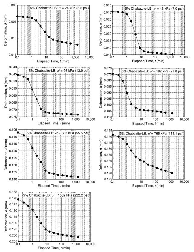
Figure A.9. Results of settlement as a function of log time for SB backfill amended with 5 % chabazite-LB.
