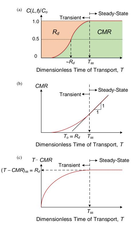
Figure 5.4. Comparison of the chemical analysis methods: (a) relative concentration (*RC*); (b) cumulative mass ratio (*CMR*) and the x-intercept from the *CMR*-to-*T* plot; (c) T-*CMR*.
