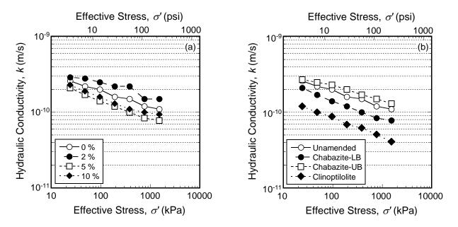
Figure 2.4. Hydraulic conductivity measured in fixed-ring oedometer cells as a function of consolidation effective stress for unamended and zeolite-amended backfills: (a) effect of different amounts of the same zeolite (chabazite-LB); (b) effect of same amount (5 %) of different types of zeolite.
