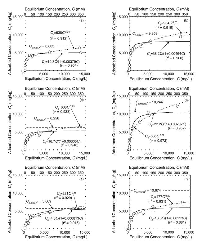
Figure 3.4. Fitted Freundlich (dashed line) and Langmuir (solid line) adsorption models for potassium (K) adsorption to zeolite-amended backfill sorbents: (a) 5 % chabazite-LB; (b) 10 % chabazite-LB; (c) 5 % chabazite-UB; (d) 10 % chabazite-UB; (e) 5 % clinoptilolite; (f) 10 % clinoptilolite.
