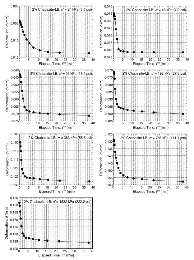
Figure A.8. Results of settlement as a function of square root time for SB backfill amended with 2 % chabazite-LB.
