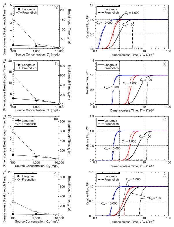
Figure 4.16. Effect of constant potassium source concentration ( $C_o$ ) on the dimensionless barrier breakthrough times,  $T_B^*$  (a, c, e) for f = 0.05 and flux breakthrough curves (b, d, f) for unamended and zeolite-amended backfills: (a) & (b) unamended; (c) & (d) 5 % chabazite-LBamended; (e) & (f) 5 % chabazite-UB-amended; (g) & (h) 5 % clinoptilolite-amended.
