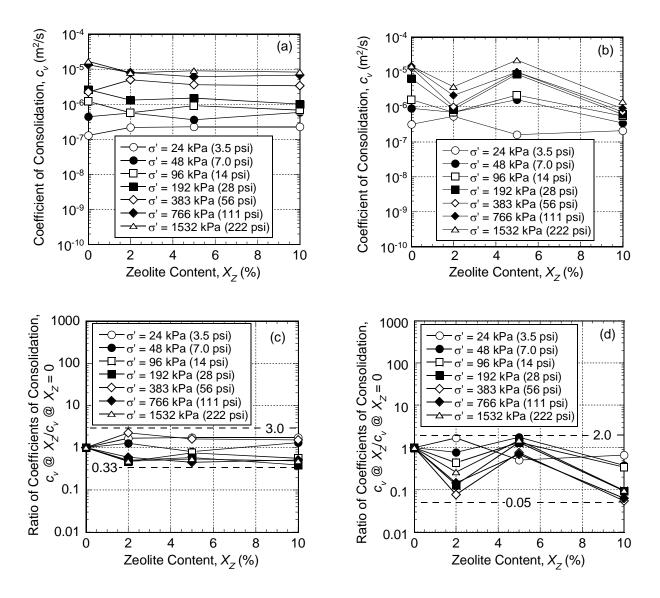
Figure 2.13. Effect of the amount of the same zeolite (chabazite-LB) on the coefficient of consolidation,  $c_{\nu}$ , of zeolite-amended backfills as a function of consolidation effective stress,  $\sigma'$ : (a)  $c_{\nu}$  based on Casagrande method; (b)  $c_{\nu}$  based on Taylor method; (c) ratio of  $c_{\nu}$  based on Casagrande method; (d) ratio of  $c_{\nu}$  based on Taylor method.
