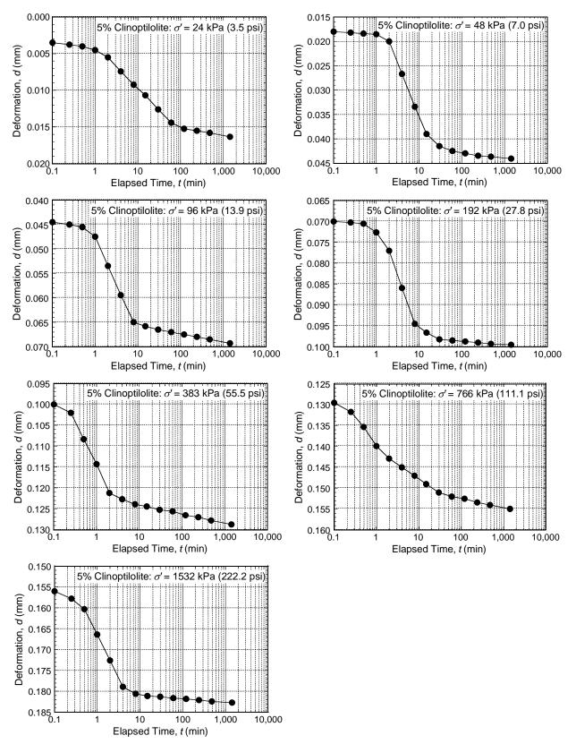
Figure A.15. Results of settlement as a function of log time for SB backfill amended with 5 % clinoptilolite.
