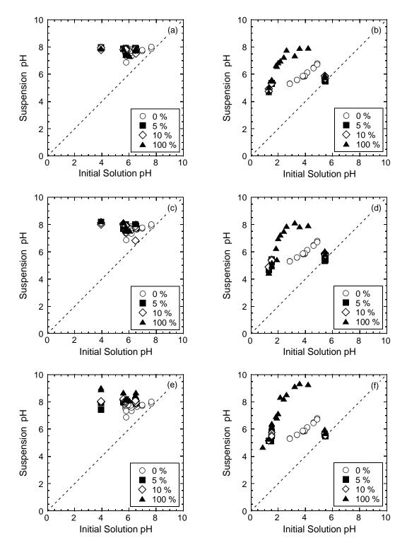
Figure 3.6. Initial salt solution pH versus the equilibrium (final) pH of the sorbate-sorbent suspension for sorbents with different percentages of zeolite amendment: (a) K with chabazite-LB; (b) Zn with chabazite-LB; (c) K with chabazite-UB; (d) Zn with chabazite-UB; (e) K with clinoptilolite; (f) Zn with clinoptilolite.
