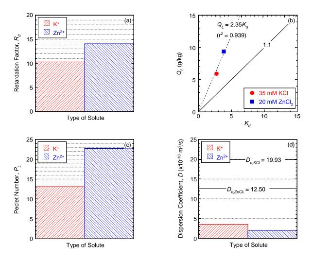
Figure 5.69. Effect of cation competition on transport parameters for backfill amended with 5 % clinoptilolite and permeated with 17.5 mM KCl plus 10 mM ZnCl<sub>2</sub> solution: (a) retardation factor ( $R_d$ ) for potassium (K<sup>+</sup>) and zinc (Zn<sup>2+</sup>); (b)  $Q_L$  versus  $K_d$ ; (c) Péclet number ( $P_L$ ) for K<sup>+</sup> and Zn<sup>2+</sup>; (d) *D* for K<sup>+</sup> and Zn<sup>2+</sup>.
