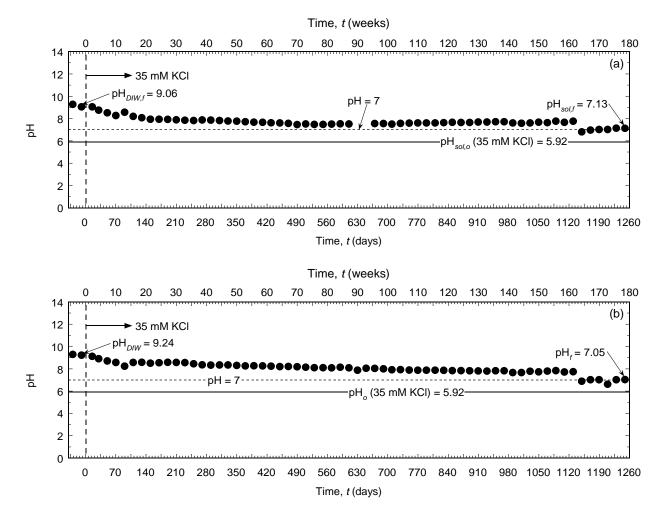
Figure 5.34. Temporal trends in the pH of the effluent for columns of backfills amended with different amounts of chabazite-LB and permeated with a solution of 35 mM KCl: (a) 5 % chabazite-LB (Test No. 9); (b) 10 % chabazite-LB (Test No. 10).
