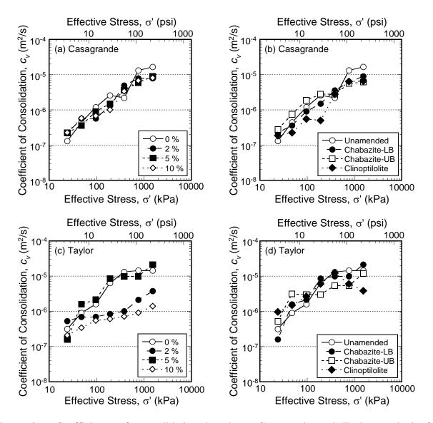
Figure 2.6. Coefficients of consolidation based on Casagrande and Taylor methods for unamended and zeolite-amended backfills as a function of consolidation effective stress: (a), (c) effect of different amounts of the same zeolite (chabazite-LB); (b), (d) effect of same amount (5%) of different types of zeolite.
