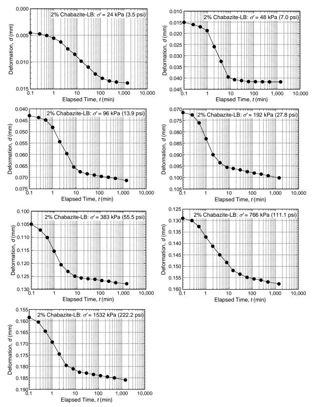
Figure A.7. Results of settlement as a function of log time for SB backfill amended with 2 % chabazite-LB.
