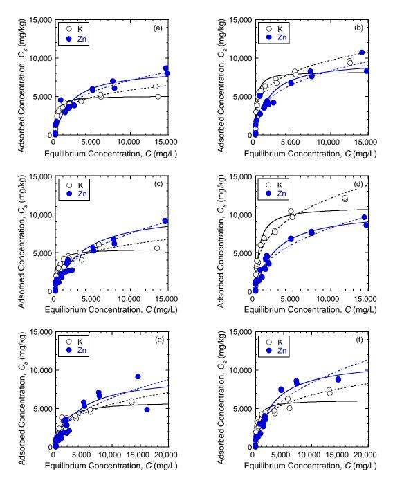
Figure 3.15. Comparison of potassium (K) versus zinc (Zn) adsorption including fitted Freundlich (dash lines) and Langmuir (solid lines) adsorption models for zeolite-amended backfill sorbents: (a) 5 % chabazite-LB; (b) 10 % chabazite-LB; (c) 5 % chabazite-UB; (d) 10 % chabazite-UB; (e) 5 % clinoptilolite; (f) 10 % clinoptilolite.
