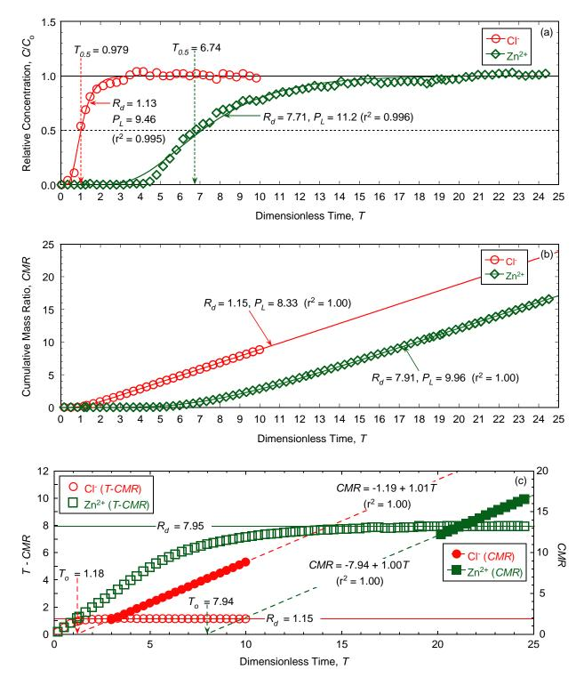
Figure 5.36. Chemical transport analyses for determination of column Péclet number ( $P_L$ ) and/or retardation factor ( $R_d$ ) for unamended backfill permeated with 20 mM ZnCl<sub>2</sub> (Test No. 2): (a) regression of relative concentration (RC) data; (b) regression of cumulative mass ratio (CMR) data; (c)  $T_o$  (=  $R_d$ ) and T - CMR analyses for  $R_d$ .
