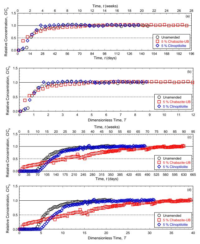
Figure 5.56. Breakthrough curves for unamended and zeolite-amended backfills permeated with 20 mM ZnCl<sub>2</sub>: (a) chloride (Cl<sup>-</sup>) versus time (*t*); (b) Cl<sup>-</sup> versus dimensionless time (*T*); (c) zinc (Zn<sup>2+</sup>) versus *t*; (d) Zn<sup>2+</sup> versus *T*.
