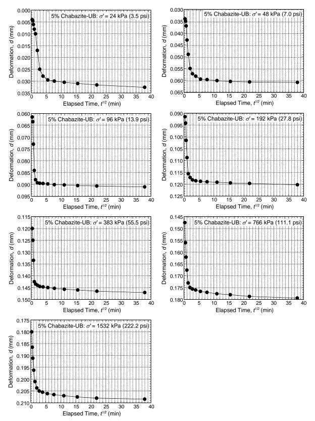
Figure A.14. Results of settlement as a function of square root time for SB backfill amended with 5 % chabazite-UB.
