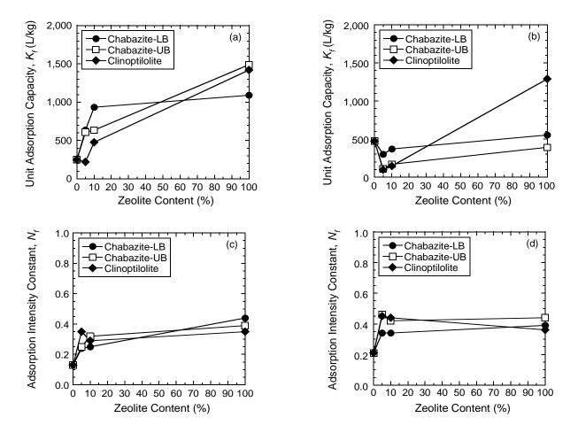
Figure 3.9. Best-fit values of the Freundlich unit adsorption capacity  $(K_f)$  and exponent  $(N_f)$  for different types and amounts of zeolite: (a)  $K_f$  for K; (b)  $K_f$  for Zn; (c)  $N_f$  for K; (d)  $N_f$  for Zn.
