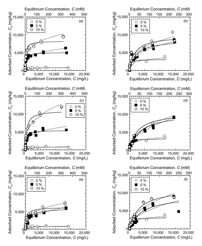
Figure 3.10. Adsorption test results fitted to the Freundlich (dashed line) and Langmuir (solid line) adsorption models for different amounts of added zeolite: (a) K with chabazite-LB; (b) Zn with chabazite-LB; (c) K with chabazite-UB; (d) Zn with chabazite-UB; (e) K with clinoptilolite; (f) Zn with clinoptilolite.
