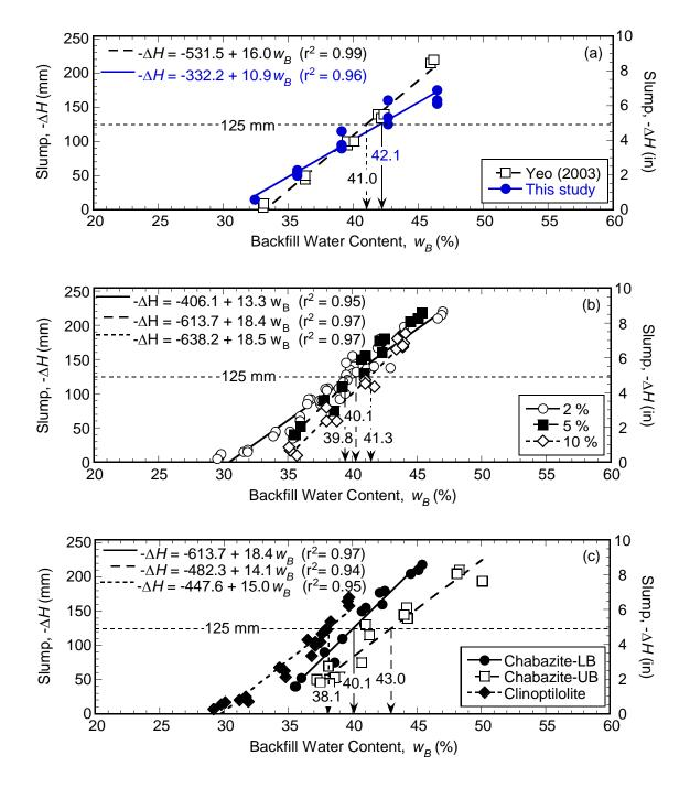
Figure 2.2. Backfill slump versus backfill gravimetric water content: (a) unamended backfill compared with the results of Yeo (2003); (b) backfills amended with different percentages of the same zeolites (chabazite-LB); (c) backfills amended with same amount (5 %) of different types of zeolites.
