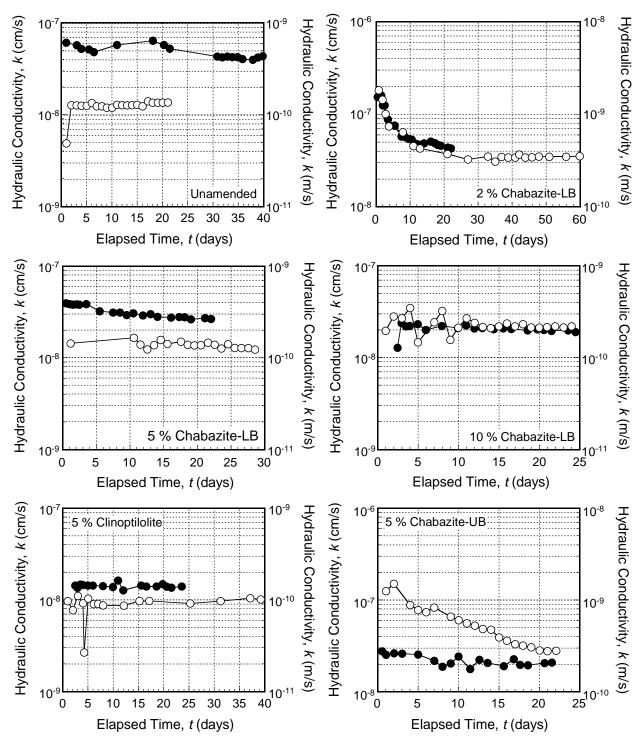
Figure A.3 Measured hydraulic conductivity for duplicate specimens in flexible-wall permeameters as a function of elapsed time for each unamended and zeolite-amended soil-bentonite backfills prepared at  $125\pm12.5$  mm slump.
