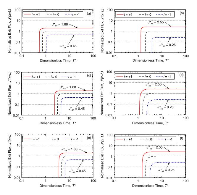
Figure E.8. Effect of Péclet number,  $P_L$ , on flux breakthrough curves with a constant source concentration,  $C_o = 1,000$  mg/L for: (a) unamended with potassium (K); (b) unamended with zinc (Zn); (c) amended with 5 % chabazite-UB with potassium (K); (d) amended with 5 % chabazite-UB with zinc (Zn); (e) amended with 10 % chabazite-UB with potassium (K); (f) amended with 10 % chabazite-UB with zinc (Zn), all based on the Freundlich adsorption model.
