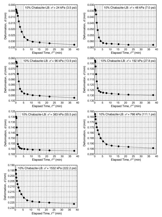
Figure A.12. Results of settlement as a function of square root time for SB backfill amended with 10 % chabazite-LB.
