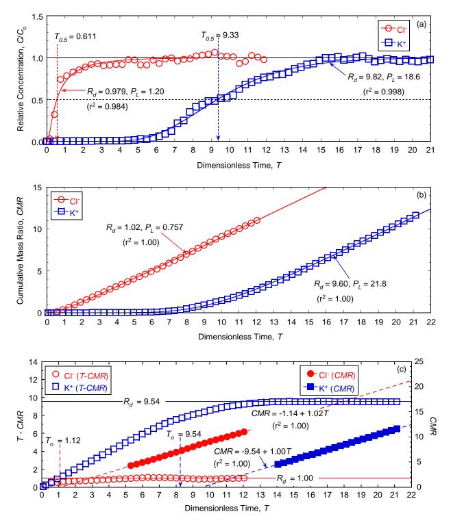
Figure 5.44. Chemical transport analyses for determination of column Péclet number ( $P_L$ ) and/or retardation factor ( $R_d$ ) for backfill amended with 5 % chabazite-LB and permeated with 35 mM KCl (Test No. 9): (a) regression of relative concentration (RC) data; (b) regression of cumulative mass ratio (*CMR*) data; (c)  $T_o$  (=  $R_d$ ) and T - CMR analyses for  $R_d$ .
