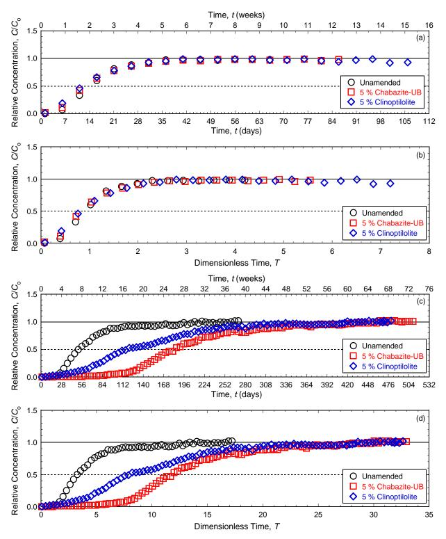
Figure 5.53. Breakthrough curves for unamended and zeolite-amended backfills permeated with 35 mM KCl: (a) chloride (Cl<sup>-</sup>) versus time (*t*); (b) Cl<sup>-</sup> versus dimensionless time (*T*); (c) potassium (K<sup>+</sup>) versus *t*; (d) K<sup>+</sup> versus *T*.
