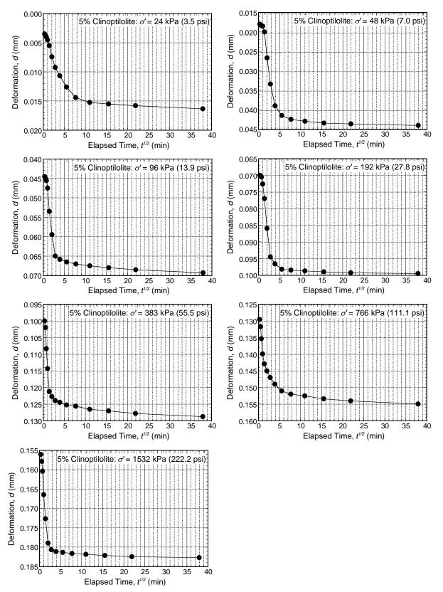
Figure A.16. Results of settlement as a function of square root time for SB backfill amended with 5 % clinoptilolite.
