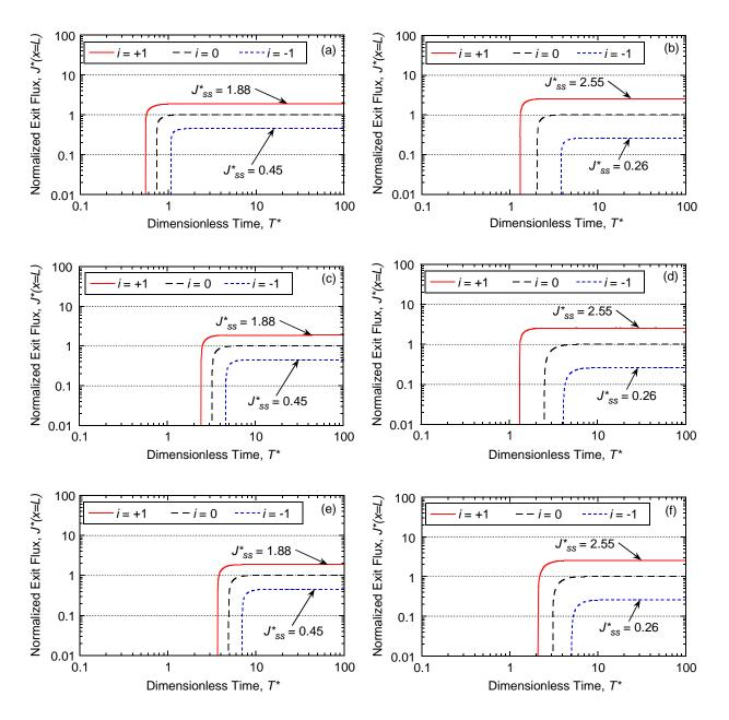
Figure E.2. Effect of Péclet number,  $P_L$ , on flux breakthrough curves with a constant source concentration,  $C_o = 1,000$  mg/L for: (a) unamended with potassium (K); (b) unamended with zinc (Zn); (c) amended with 5 % chabazite-LB with potassium (K); (d) amended with 5 % chabazite-LB with zinc (Zn); (e) amended with 10 % chabazite-LB with potassium (K); (f) amended with 10 % chabazite-LB with zinc (Zn), all based on the Freundlich adsorption model.
