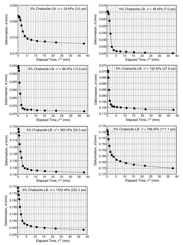
Figure A.10. Results of settlement as a function of square root time for SB backfill amended with 5 % chabazite-LB.
