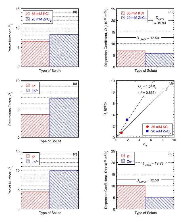
Figure 5.63. Effect of type of metal on transport parameters for columns of unamended backfill permeated with 35 mM KCl or 20 mM ZnCl<sub>2</sub>: (a) Péclet number ( $P_L$ ) for chloride (Cl<sup>-</sup>); (b) hydrodynamic dispersion coefficient (D) for Cl<sup>-</sup>; (c) retardation factor ( $R_d$ ) for potassium (K<sup>+</sup>) and zinc (Zn<sup>2+</sup>); (d)  $Q_L$  versus  $K_d$ ; (e)  $P_L$  for K<sup>+</sup> and Zn<sup>2+</sup>; (f) D for K<sup>+</sup> and Zn<sup>2+</sup>.
