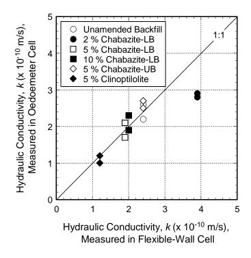
Figure 2.5. Correlation between geometric mean of hydraulic conductivity, k, measured in flexible-wall cell at an average effective stress,  $\sigma$ , of 34.5 kPa (5.0 psi) versus k measured in fixed-ring oedometer cell for 24 kPa (3.5 psi) and 48 kPa (7.0 psi).
