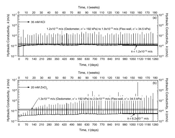
Figure 5.13. Temporal trends in hydraulic conductivity for columns of backfills amended with different amounts of chabazite-LB and permeated with a solution of 35 mM KCl: (a) 5 % chabazite-LB (Test No. 9); (b) 10 % chabazite-LB (Test No. 10).
