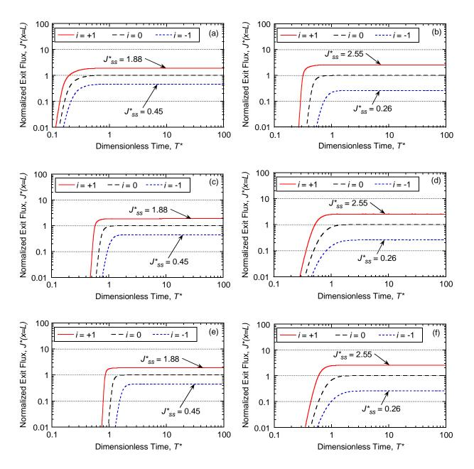
Figure E.6. Effect of Péclet number,  $P_L$ , on flux breakthrough curves with a constant source concentration,  $C_o = 10,000 \text{ mg/L}$  for: (a) unamended with potassium (K); (b) unamended with zinc (Zn); (c) amended with 5 % chabazite-LB with potassium (K); (d) amended with 5 % chabazite-LB with zinc (Zn); (e) amended with 10 % chabazite-LB with potassium (K); (f) amended with 10 % chabazite-LB with zinc (Zn), all based on the Langmuir adsorption model.
