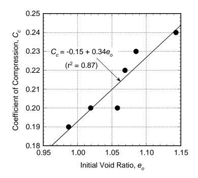
Figure 2.10. Correlation between initial void ratio and compression index zeolite-amended backfills with different amounts and/or types of zeolites.
