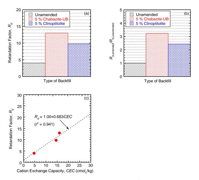
Figure 5.54. Effect of type of zeolite on retardation of potassium (K<sup>+</sup>) for columns of unamended and zeolite-amended backfills permeated with 35 mM KCl: (a) retardation factor ( $R_d$ ); (b) ratio of  $R_d$  for the zeolite-amended backfill relative to  $R_d$  for the unamended backfill ( $R_{d,amended}/R_{d,unamended}$ ); (c) cation exchange capacity (*CEC*) of backfill and  $R_d$  of K<sup>+</sup>.
