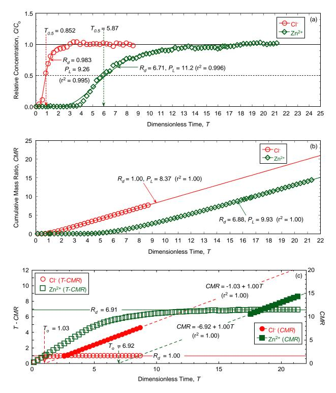
Figure 5.37. Chemical transport analyses for determination of column Péclet number ( $P_L$ ) and/or retardation factor ( $R_d$ ) for unamended backfill permeated with 20 mM ZnCl<sub>2</sub> (Test No. 2): (a) regression of relative concentration (RC) data; (b) regression of cumulative mass ratio (CMR) data; (c)  $T_o$  (=  $R_d$ ) and T - CMR analyses for  $R_d$ .
