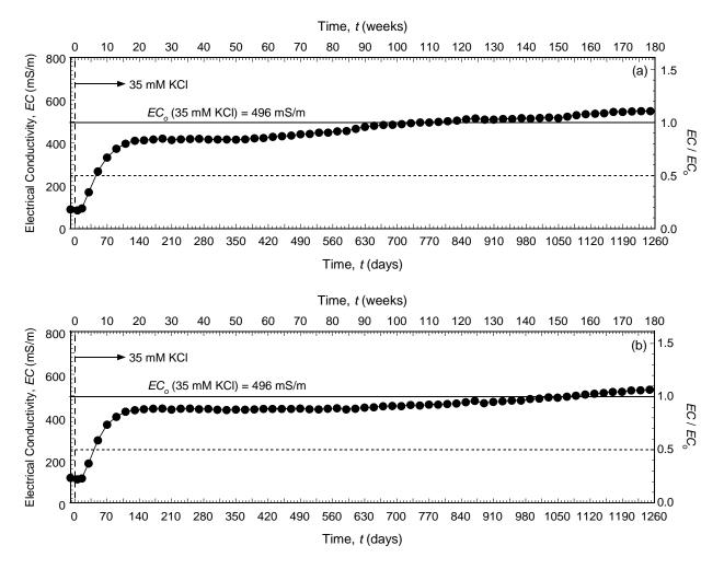
Figure 5.30. Temporal trends in the electrical conductivity of the effluent for columns of backfills amended with different amounts of chabazite-LB and permeated with a solution of 35 mM KCl: (a) 5 % chabazite-LB (Test No. 9); (b) 10 % chabazite-LB (Test No. 10).
