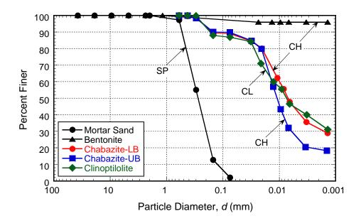
Figure 2.1. Measured particle-size distributions (ASTM D422-ASTM 2007) for constituent materials used in study. Letter designations associated with curves represent classifications based on the Unified Soil Classification System (ASTM D2487-ASTM 2008).
