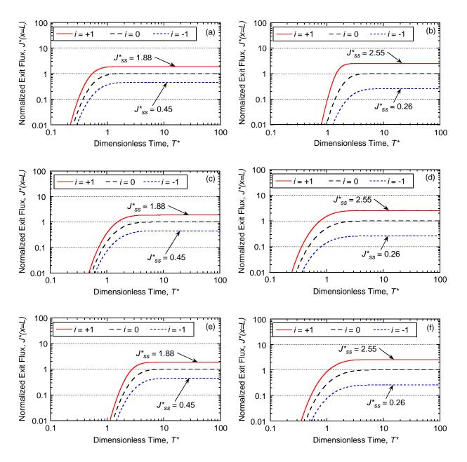
Figure E.17. Effect of Péclet number,  $P_L$ , on flux breakthrough curves with a constant source concentration,  $C_o = 1,000$  mg/L for: (a) unamended with potassium (K); (b) unamended with zinc (Zn); (c) amended with 5 % clinoptilolite with potassium (K); (d) amended with 5 % clinoptilolite with zinc (Zn); (e) amended with 10 % clinoptilolite with potassium (K); (f) amended with 10 % clinoptilolite with zinc (Zn), all based on the Langmuir adsorption model.
