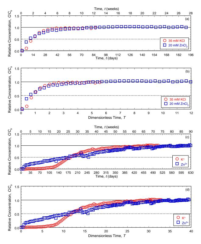
Figure 5.64. Breakthrough curves for backfill amended with 5 % chabazite-UB and permeated with 35 mM KCl or 20 mM ZnCl<sub>2</sub>: (a) chloride (Cl<sup>-</sup>) versus time (*t*); (b) Cl<sup>-</sup> versus dimensionless time (*T*); (c) potassium (K<sup>+</sup>) and zinc (Zn<sup>2+</sup>) versus *t*; (d) K<sup>+</sup> and Zn<sup>2+</sup> versus *T*.
