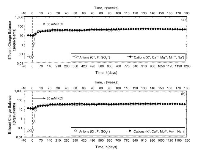
Figure 5.26. Temporal trends in effluent charge balance for columns of backfills amended with different amounts of chabazite-LB and permeated with a solution of 35 mM KCl (Test No. 9): (a) 5 % chabazite-LB; (b) 10 % chabazite-LB (Test No. 10). [Note: absolute values for the  $\sum$ anion equivalents are shown].
