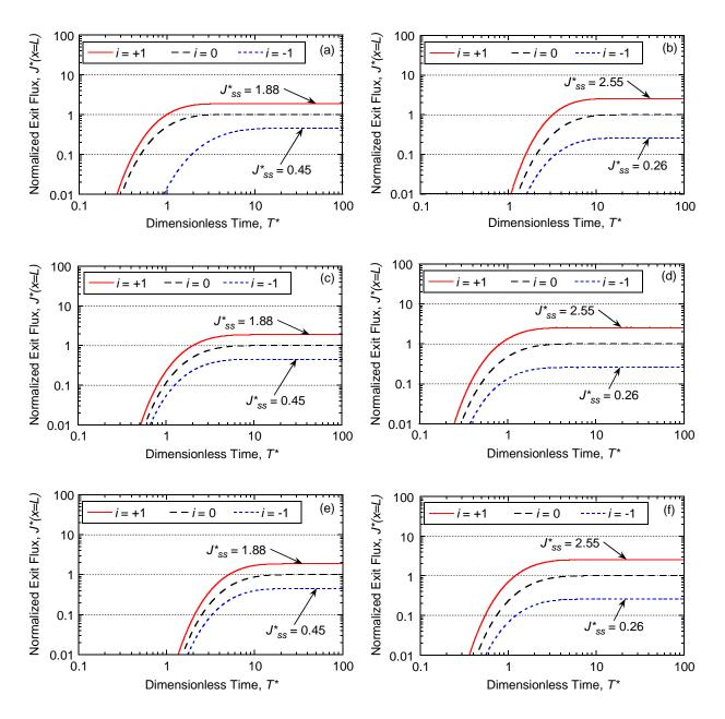
Figure E.16. Effect of Péclet number,  $P_L$ , on flux breakthrough curves with a constant source concentration,  $C_o = 100 \text{ mg/L}$  for: (a) unamended with potassium (K); (b) unamended with zinc (Zn); (c) amended with 5 % clinoptilolite with potassium (K); (d) amended with 5 % clinoptilolite with zinc (Zn); (e) amended with 10 % clinoptilolite with potassium (K); (f) amended with 10 % clinoptilolite with zinc (Zn), all based on the Langmuir adsorption model.
