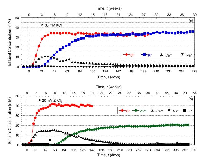
Figure 5.15. Temporal trends in effluent solute concentrations for columns of unamended backfills permeated with different salt solutions: (a) 35 mM KCl (Test No. 1); (b) 20 mM  $ZnCl_2$  (Test No. 2).
