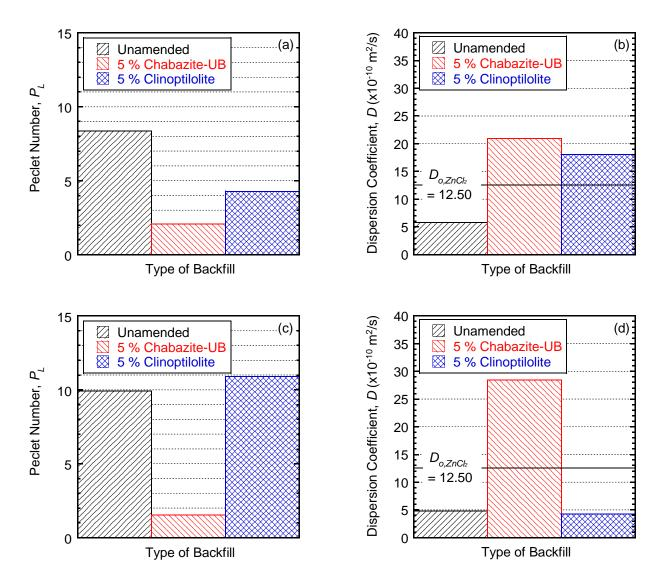
Figure 5.58. Effect of type of zeolite on transport parameters for columns of unamended and zeolite-amended backfills permeated with 20 mM ZnCl<sub>2</sub>: (a) Péclet number ( $P_L$ ) for chloride (Cl<sup>-</sup>); (b) hydrodynamic dispersion coefficient (D) for Cl<sup>-</sup>; (c)  $P_L$  for zinc (Zn<sup>2+</sup>); (d) D for Zn<sup>2+</sup>.
