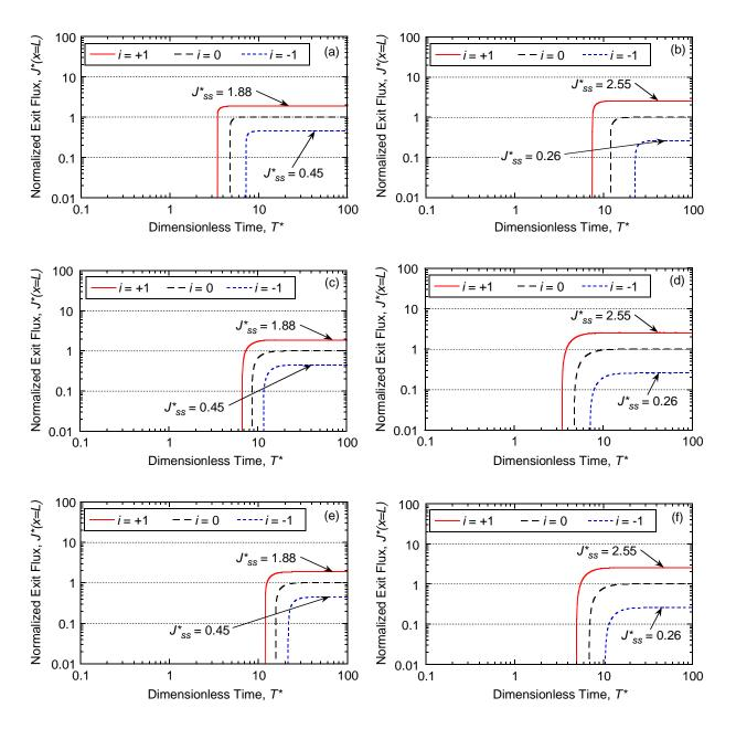
Figure E.13. Effect of Péclet number,  $P_L$ , on flux breakthrough curves with a constant source concentration,  $C_o = 100 \text{ mg/L}$  for: (a) unamended with potassium (K); (b) unamended with zinc (Zn); (c) amended with 5 % clinoptilolite with potassium (K); (d) amended with 5 % clinoptilolite with zinc (Zn); (e) amended with 10 % clinoptilolite with potassium (K); (f) amended with 10 % clinoptilolite with zinc (Zn), all based on the Freundlich adsorption model.
