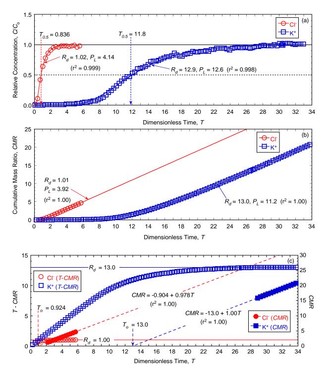
Figure 5.38. Chemical transport analyses for determination of column Péclet number ( $P_L$ ) and/or retardation factor ( $R_d$ ) for backfill amended with 5 % chabazite-UB and permeated with 35 mM KCl (Test No. 3): (a) regression of relative concentration (RC) data; (b) regression of cumulative mass ratio (CMR) data; (c)  $T_o$  (=  $R_d$ ) and T - CMR analyses for  $R_d$ .
