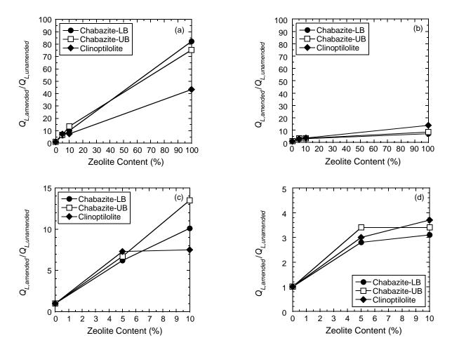
Figure 3.11. Comparison of the ratio of the maximum adsorption capacity  $(Q_L)$  of the zeoliteamended backfill sorbents  $(Q_{L,amended})$  relative to the  $Q_L$  of the unamended backfill sorbent  $(Q_{L,unamended})$  for different types and amounts of zeolite: (a) K including 100 % zeolite; (b) Zn including 100 % zeolite; (c) K for zeolite content  $\leq 10$  %; (d) Zn for zeolite content  $\leq 10$  %.
