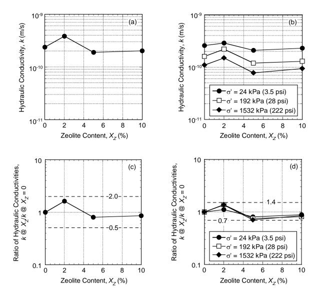
Figure 2.11. Effect of the amount of the same zeolite (chabazite-LB) on the hydraulic conductivity, k, of zeolite-amended backfills: (a) geometric mean of k values measured using flexible-wall cells; (b) k values measured in fixed-ring oedometer cells as a function of consolidation effective stress,  $\sigma'$ ; (c) ratio of geometric mean k values measured using flexible-wall cells; (d) ratio of k values measured in fixed-ring oedometer cells as a function of  $\sigma'$ .
