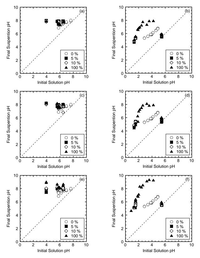
Figure B.1. Change in initial solution pH after the experiments for the unamended, zeoliteamended and 100 % zeolite: (a) chabazite-LB for  $K^+$ ; (b) chabazite-LB for  $Zn^{2+}$ ; (c) chabazite-UB for  $K^+$ ; (d) chabazite-UB for  $Zn^{2+}$ ; (e) clinoptilolite for  $K^+$ ; (f) clinoptilolite for  $Zn^{2+}$ .
