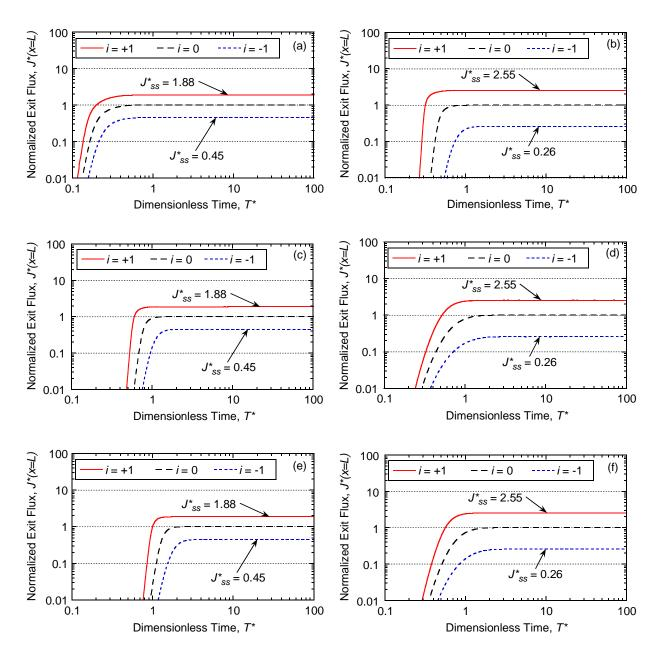
Figure E.12. Effect of Péclet number,  $P_L$ , on flux breakthrough curves with a constant source concentration,  $C_o = 10,000 \text{ mg/L}$  for: (a) unamended with potassium (K); (b) unamended with zinc (Zn); (c) amended with 5 % chabazite-UB with potassium (K); (d) amended with 5 % chabazite-UB with zinc (Zn); (e) amended with 10 % chabazite-UB with potassium (K); (f) amended with 10 % chabazite-UB with zinc (Zn), all based on the Langmuir adsorption model.
