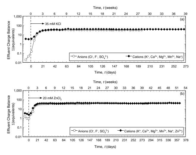
Figure 5.23. Temporal trends in effluent charge balance for columns of unamended backfills permeated with different salt solutions: (a) 35 mM KCl (Test No. 1); (b) 20 mM ZnCl<sub>2</sub> (Test No. 2). [Note: absolute values for the  $\sum$ anion equivalents are shown].
