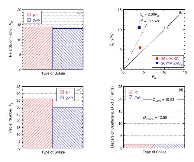
Figure 5.68. Effect of cation competition on transport parameters for backfill amended with 5 % chabazite-UB and permeated with 17.5 mM KCl plus 10 mM ZnCl<sub>2</sub> solution: (a) retardation factor ( $R_d$ ) for potassium (K<sup>+</sup>) and zinc (Zn<sup>2+</sup>); (b)  $Q_L$  versus  $K_d$ ; (c) Péclet number ( $P_L$ ) for K<sup>+</sup> and Zn<sup>2+</sup>; (d) *D* for K<sup>+</sup> and Zn<sup>2+</sup>.
