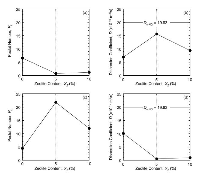
Figure 5.61. Effect of amount of zeolite on the Péclet number ( $P_L$ ) and hydrodynamic dispersion coefficient (D) of chloride (Cl<sup>-</sup>) and potassium (K<sup>+</sup>) for backfills with 0 (unamended), 5 and 10 % chabazite-LB permeated with 35 mM KCl: (a)  $P_L$  for Cl<sup>-</sup>; (b) D for Cl<sup>-</sup>; (c)  $P_L$  for K<sup>+</sup>; (d) D for K<sup>+</sup>.
