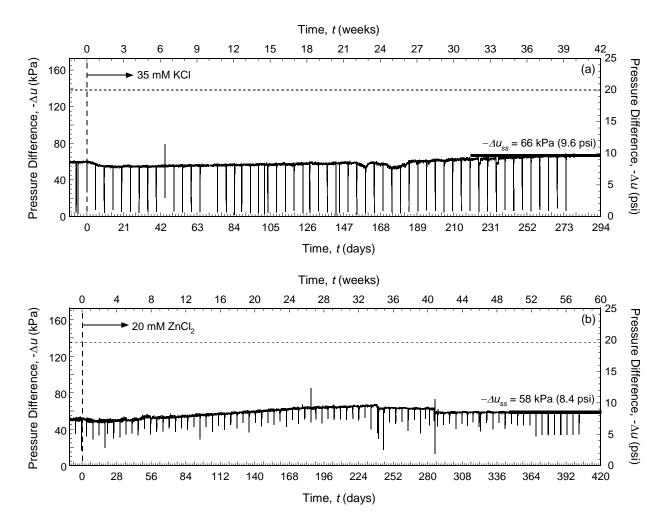
Figure 5.6. Temporal trends in pressure differences across columns of unamended backfills permeated with different salt solutions: (a) 35 mM KCl (Test No. 1); (b) 20 mM  $ZnCl_2$  (Test No. 2).
