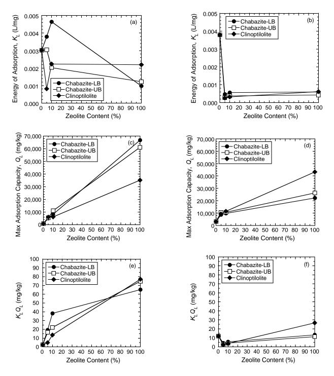
Figure 3.8. Best-fit values of the Langmuir energy of adsorption ( $K_L$ ), maximum adsorption capacity ( $Q_L$ ), and  $K_LQ_L$  for different types and amounts of zeolite: (a)  $K_L$  for K; (b)  $K_L$  for Zn; (c)  $Q_L$  for K; (d)  $Q_L$  for Zn; (e)  $K_LQ_L$  for K; (f)  $K_LQ_L$  for Zn.
