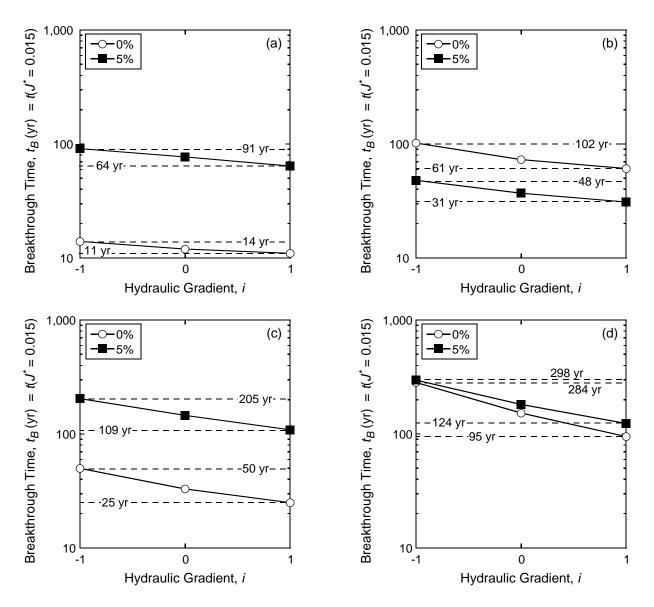
Figure E.20. Relationship between Péclet number,  $P_L$ , and predicted flux breakthrough times corresponding to  $J^*(x = L) = 0.015$  with a constant source concentration ( $C_o$ ) of 1,000 mg/L for the unamended and zeolite-amended cutoff wall with 5 % chabazite-LB: (a) potassium (K), Langmuir; (b) zinc (Zn), Langmuir; (c) potassium (K), Freundlich; (d) zinc (Zn), Freundlich.
