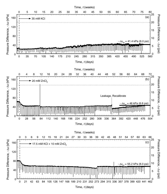
Figure 5.8. Temporal trends in pressure differences across columns of backfills amended with 5 % clinoptilolite and permeated with different salt solutions: (a) 35 mM KCl (Test No. 6); (b) 20 mM ZnCl<sub>2</sub> (Test No. 7); (c) 17.5 mM KCl plus 10 mM ZnCl<sub>2</sub> (Test No. 8).
