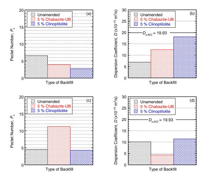
Figure 5.55. Effect of type of zeolite on transport parameters for columns of unamended and zeolite-amended backfills permeated with 35 mM KCl: (a) Péclet number ( $P_L$ ) for chloride (Cl<sup>-</sup>); (b) hydrodynamic dispersion coefficient (D) for Cl<sup>-</sup>; (c)  $P_L$  for potassium (K<sup>+</sup>); (d) D for K<sup>+</sup>.
