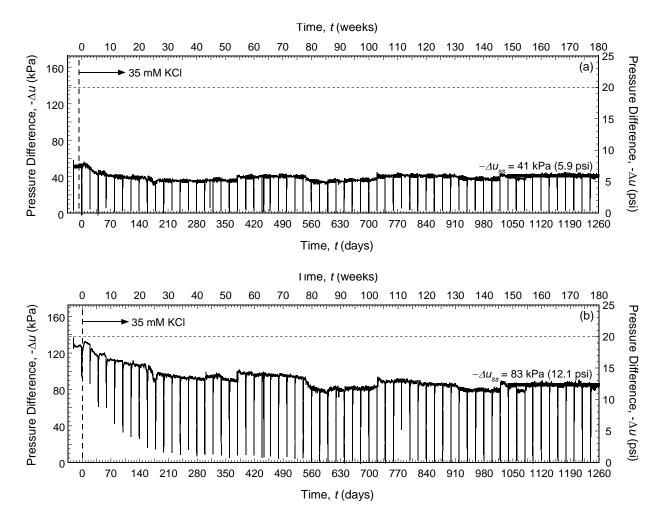
Figure 5.9. Temporal trends in pressure differences across columns of backfills amended with different amounts of chabazite-LB and permeated with a solution of 35 mM KCl: (a) 5 % chabazite-LB (Test No. 9); (b) 10 % chabazite-LB (Test No. 10).
