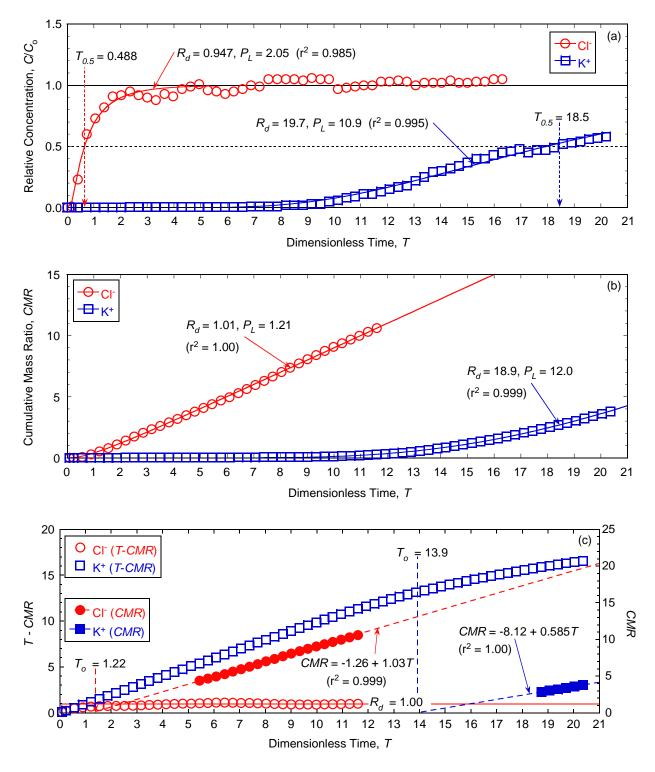
Figure 5.45. Chemical transport analyses for determination of column Péclet number ( $P_L$ ) and/or retardation factor ( $R_d$ ) for backfill amended with 10 % chabazite-LB and permeated with 35 mM KCl (Test No. 10): (a) regression of relative concentration (RC) data; (b) regression of cumulative mass ratio (CMR) data; (c)  $T_o$  (=  $R_d$ ) and T - CMR analyses for  $R_d$ .
