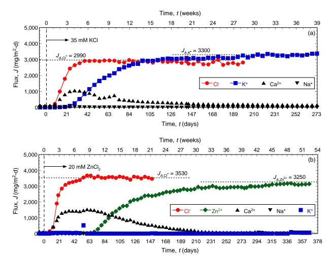
Figure 5.19. Temporal trends in effluent solute flux for columns of unamended backfills permeated with different salt solutions: (a) 35 mM KCl (Test No. 1); (b) 20 mM  $ZnCl_2$  (Test No. 2).
