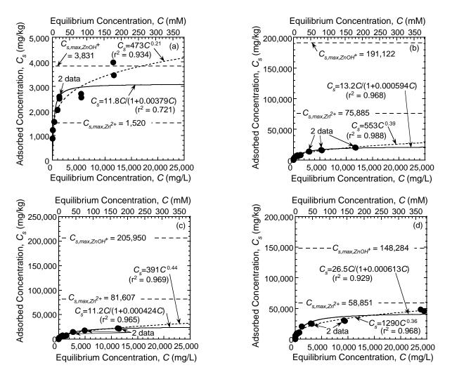
Figure 3.3. Fitted Freundlich (dashed line) and Langmuir (solid line) adsorption models for zinc (Zn) adsorption: (a) unamended backfill sorbent; (b) 100 % chabazite-LB; (c) 100 % chabazite-UB; (d) 100 % clinoptilolite.
