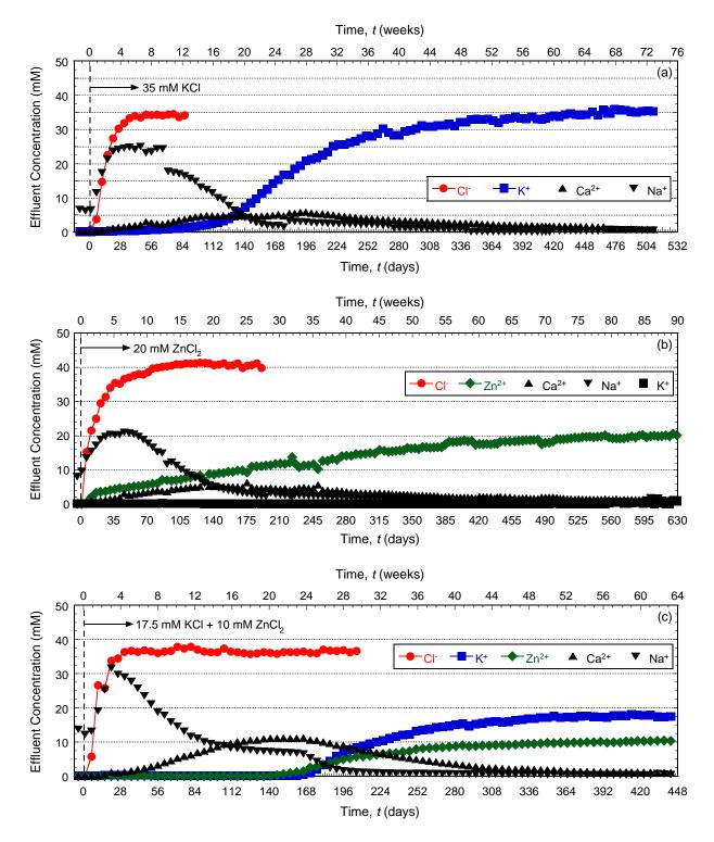
Figure 5.16. Temporal trends in effluent solute concentrations for columns of backfills amended with 5 % chabazite-UB and permeated with different salt solutions: (a) 35 mM KCl (Test No. 3); (b) 20 mM ZnCl<sub>2</sub> (Test No. 4); (c) 17.5 mM KCl plus 10 mM ZnCl<sub>2</sub> (Test No. 5).
