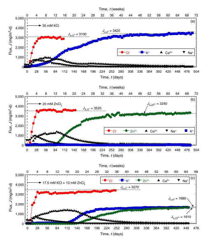
Figure 5.21. Temporal trends in effluent solute flux from for columns of backfills amended with 5 % clinoptilolite and permeated with different salt solutions: (a) 35 mM KCl (Test No. 6); (b) 20 mM ZnCl<sub>2</sub> (Test No. 7); (c) 17.5 mM KCl plus 10 mM ZnCl<sub>2</sub> (Test No. 8).
