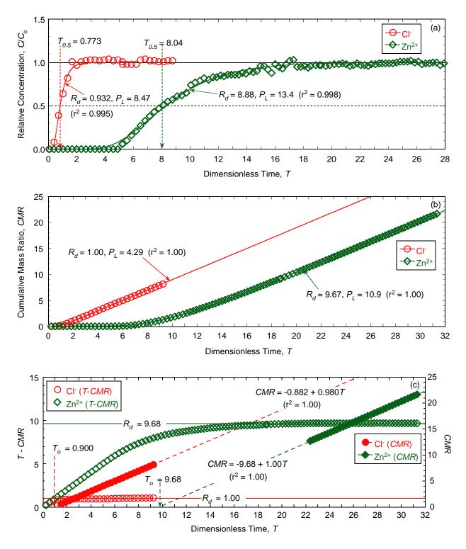
Figure 5.42. Chemical transport analyses for determination of column Péclet number ( $P_L$ ) and/or retardation factor ( $R_d$ ) for backfill amended with 5 % clinoptilolite and permeated with 20 mM ZnCl<sub>2</sub> (Test No. 7): (a) regression of relative concentration (RC) data; (b) regression of cumulative mass ratio (CMR) data; (c)  $T_o$  (=  $R_d$ ) and T - CMR analyses for  $R_d$ .
