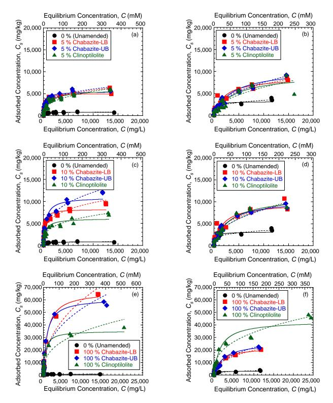
Figure 3.12. Adsorption test results fitted to the Freundlich (dashed line) and Langmuir (solid line) adsorption models for different amounts and types of zeolite: (a) K with 5 % zeolite; (b) Zn with 5 % zeolite; (c) K with 10 % zeolite; (d) Zn with 10 % zeolite; (e) K with 100 % zeolite K; (f) Zn with 100 % zeolite.
