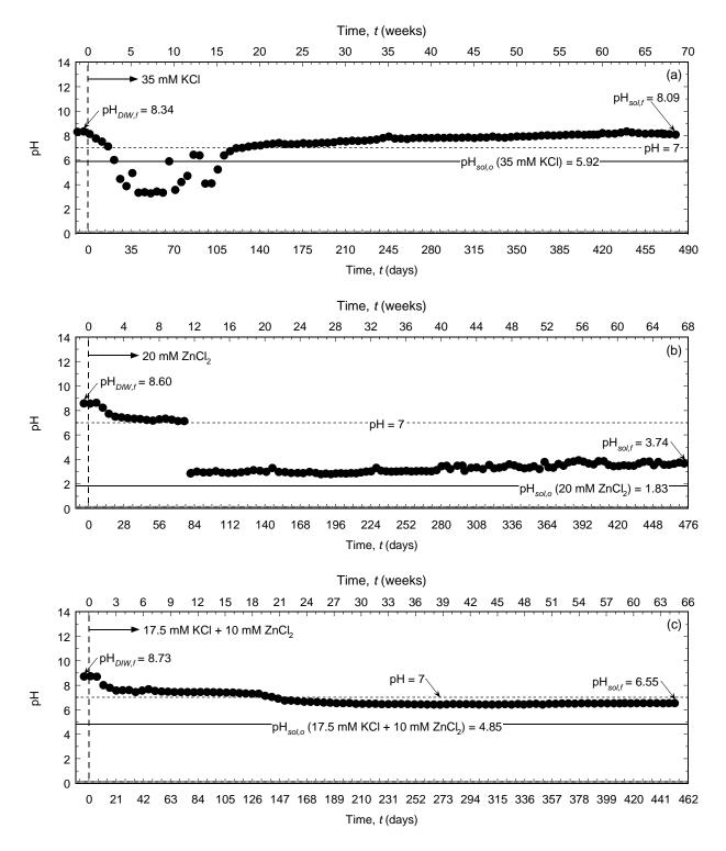
Figure 5.33. Temporal trends in the pH of the effluent for columns of backfills amended with 5 % clinoptilolite permeated with different salt solutions: (a) 35 mM KCl (Test No. 6); (b) 20 mM ZnCl<sub>2</sub> (Test No. 7); (c) 17.5 mM KCl plus 10 mM ZnCl<sub>2</sub> (Test No. 8).
