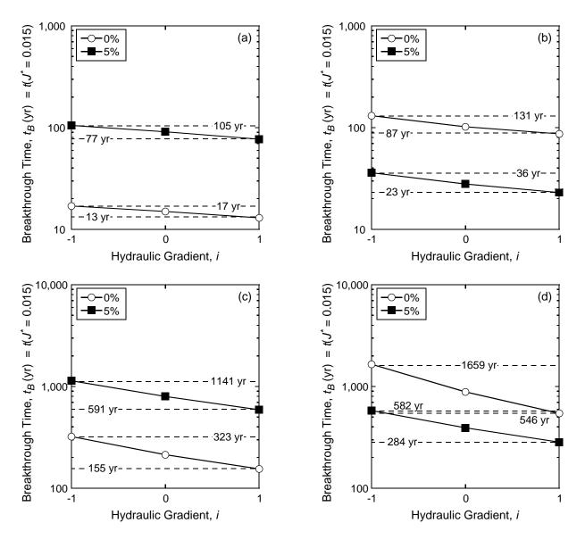
Figure E.22. Relationship between Péclet number,  $P_L$ , and predicted flux breakthrough times corresponding to  $J^*(x = L) = 0.015$  with a constant source concentration ( $C_o$ ) of 100 mg/L for the unamended and zeolite-amended cutoff wall with 5 % chabazite-UB: (a) potassium (K), Langmuir; (b) zinc (Zn), Langmuir; (c) potassium (K), Freundlich; (d) zinc (Zn), Freundlich.
