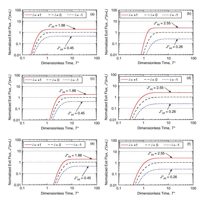
Figure E.11. Effect of Péclet number,  $P_L$ , on flux breakthrough curves with a constant source concentration,  $C_o = 1,000$  mg/L for: (a) unamended with potassium (K); (b) unamended with zinc (Zn); (c) amended with 5 % chabazite-UB with potassium (K); (d) amended with 5 % chabazite-UB with zinc (Zn); (e) amended with 10 % chabazite-UB with potassium (K); (f) amended with 10 % chabazite-UB with zinc (Zn), all based on the Langmuir adsorption model.
