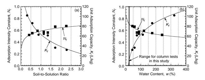
Figure 5.48. The Freundlich sorption parameters as a function of (a) soil-to-solution ratio and (b) the gravimetric water content (data from Manassero *et al.* 1998).
