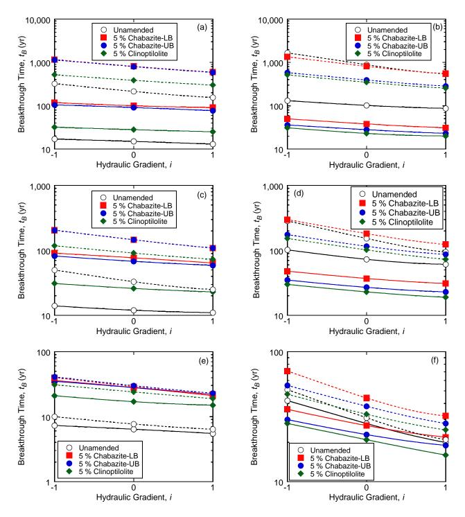
Figure 4.14. Relationship between direction and magnitude of hydraulic gradient (*i*) and barrier flux breakthrough time based  $J^*(L,t)$  of 0.015 for unamended and 5 % zeolite-amended backfills: (a), (c), (e) potassium source concentration ( $C_o$ ) of 100, 1,000, and 10,000 mg/L, respectively; (b), (d), (f) zinc  $C_o$  of 100, 1,000, and 10,000 mg/L respectively. Note: dashed line = Freundlich adsorption model; solid line = Langmuir adsorption model.
