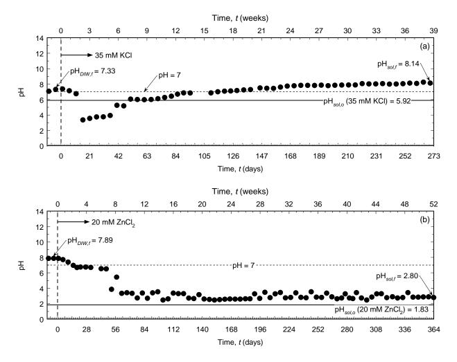
Figure 5.31. Temporal trends in the pH of the effluent for columns with unamended backfills permeated with different salt solutions: (a) 35 mM KCl (Test No. 1); (b) 20 mM  $ZnCl_2$  (Test No. 2).
