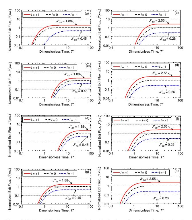
Figure 4.6. Effect of direction and magnitude of hydraulic gradient (*i*) on flux breakthrough curves for unamended and zeolite-amended backfills based on the Langmuir adsorption model for a constant source concentration ( $C_o$ ) of 100 mg/L: (a) potassium (K), unamended; (b) zinc (Zn), unamended; (c) K, 5 % chabazite-LB-amended; (d) Zn, 5 % chabazite-LB-amended; (e) K, 10 % chabazite-LB-amended; (f) Zn, 10 % chabazite-LB-amended; (g) K, 5 % clinoptilolite-amended.
