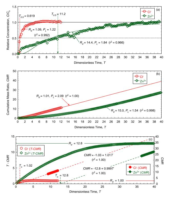
Figure 5.39. Chemical transport analyses for determination of column Péclet number ( $P_L$ ) and/or retardation factor ( $R_d$ ) for backfill amended with 5 % chabazite-UB and permeated with 20 mM ZnCl<sub>2</sub> (Test No. 4): (a) regression of relative concentration (RC) data; (b) regression of cumulative mass ratio (CMR) data; (c)  $T_o$  (=  $R_d$ ) and T - CMR analyses for  $R_d$ .
