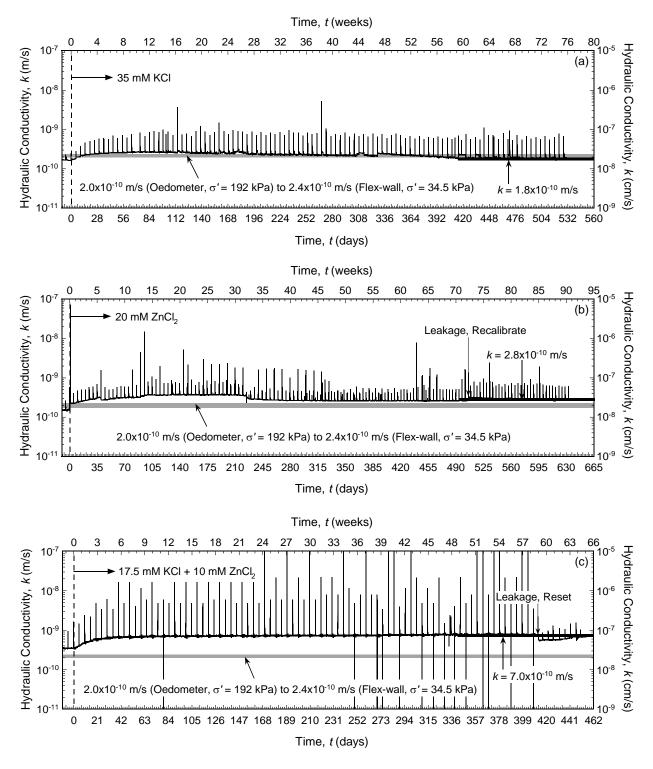
Figure 5.11. Temporal trends in hydraulic conductivity for columns of backfills amended with 5 % chabazite-UB and permeated with different salt solutions: (a) 35 mM KCl (Test No. 3); (b) 20 mM ZnCl<sub>2</sub> (Test No. 4); (c) 17.5 mM KCl plus 10 mM ZnCl<sub>2</sub> (Test No. 5).
