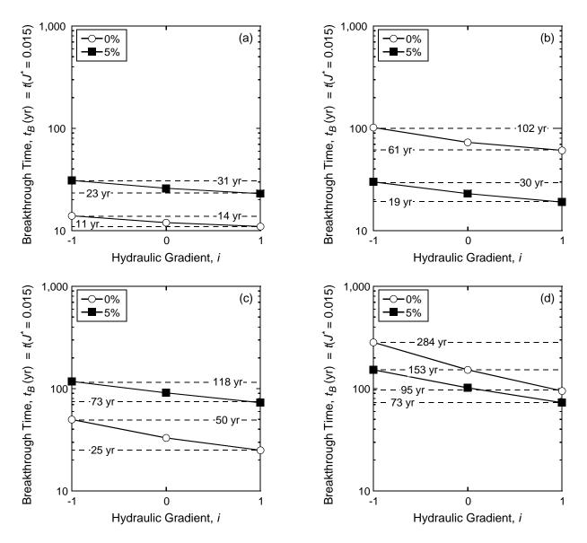
Figure E.26. Relationship between Péclet number,  $P_L$ , and predicted flux breakthrough times corresponding to  $J^*(x = L) = 0.015$  with a constant source concentration ( $C_o$ ) of 1,000 mg/L for the unamended and zeolite-amended cutoff wall with 5 % clinoptilolite: (a) potassium (K), Langmuir; (b) zinc (Zn), Langmuir; (c) potassium (K), Freundlich; (d) zinc (Zn), Freundlich.
