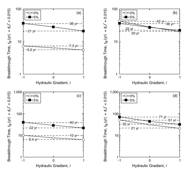
Figure E.21. Relationship between Péclet number,  $P_L$ , and predicted flux breakthrough times corresponding to  $J^*(x = L) = 0.015$  with a constant source concentration ( $C_o$ ) of 10,000 mg/L for the unamended and zeolite-amended cutoff wall with 5 % chabazite-LB: (a) potassium (K), Langmuir; (b) zinc (Zn), Langmuir; (c) potassium (K), Freundlich; (d) zinc (Zn), Freundlich.
