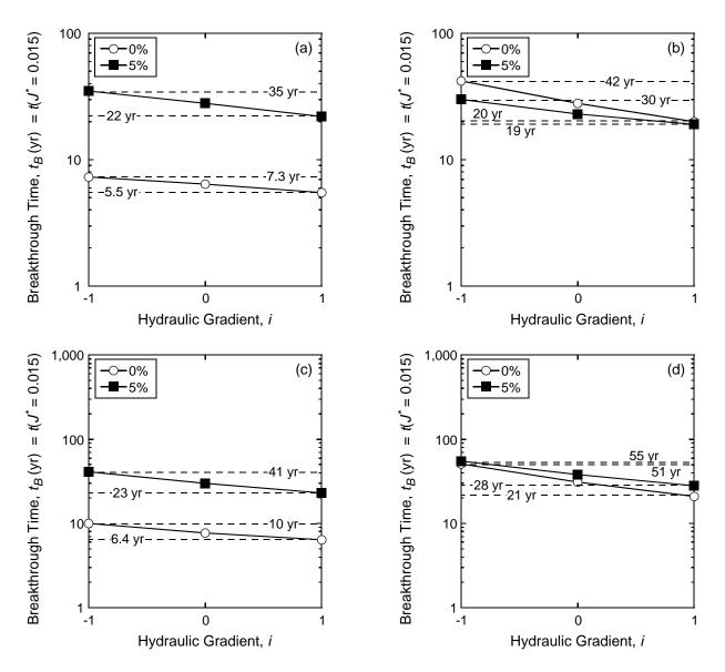
Figure E.24. Relationship between Péclet number,  $P_L$ , and predicted flux breakthrough times corresponding to  $J^*(x = L) = 0.015$  with a constant source concentration ( $C_o$ ) of 10,000 mg/L for the unamended and zeolite-amended cutoff wall with 5 % chabazite-UB: (a) potassium (K), Langmuir; (b) zinc (Zn), Langmuir; (c) potassium (K), Freundlich; (d) zinc (Zn), Freundlich.
