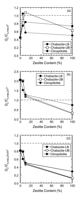
Figure 3.7. Ratio of the maximum adsorption capacity,  $Q_L$  (mg/kg) to the theoretical maximum solid-phase concentration,  $C_{s,max}$  (mg/kg) for different types and amounts of zeolite: (a) K<sup>+</sup>; (b) Zn<sup>2+</sup>; (c) ZnOH<sup>+</sup>.
