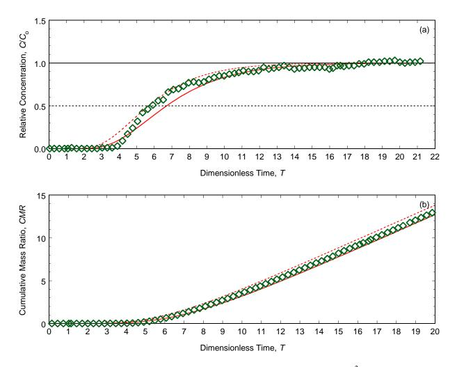
Figure F.2. Comparison of the measured column effluent data for zinc  $(Zn^{2+})$  versus the model simulation using  $R_d$  based on the BEAT results and  $P_L$  from regression of the measured column effluent data for the unamended backfill permeated with 20 mM ZnCl<sub>2</sub> (Test No. 2): (a) relative concentration (*RC*) data; (b) cumulative mass ratio (*CMR*) data. Note: dashed line =  $R_d$  based on Freundlich adsorption model; solid line =  $R_d$  based on Langmuir adsorption model.
