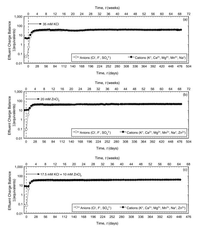
Figure 5.25. Temporal trends in effluent charge balance for columns of backfills amended with 5 % clinoptilolite and permeated with different salt solutions: (a) 35 mM KCl (Test No. 6); (b) 20 mM ZnCl<sub>2</sub> (Test No. 7); (c) 17.5 mM KCl plus 10 mM ZnCl<sub>2</sub> (Test No. 8). [Note: absolute values for the  $\Sigma$ anion equivalents are shown].
