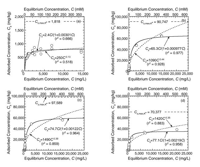
Figure 3.2. Fitted Freundlich (dashed line) and Langmuir (solid line) adsorption models for potassium (K) adsorption: (a) unamended backfill sorbent; (b) 100 % chabazite-LB; (c) 100 % chabazite-UB; (d) 100 % clinoptilolite.
