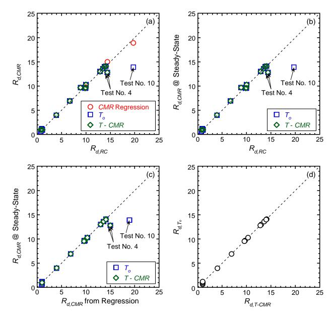
Figure 5.46. Comparison of the retardation factor  $(R_d)$ : (a)  $R_d$  from relative concentration (RC) versus  $R_d$  from cumulative mass ratio (CMR); (b)  $R_d$  from RC versus  $R_d$  from steady–state CMR; (c)  $R_d$  from CMR versus  $R_d$  from steady–state CMR; (d)  $R_d$  from (T-CMR) versus  $T_o$ .
