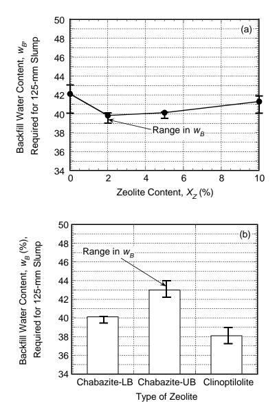
Figure 2.7. Backfill water content required to achieve a 125-mm (5-in) slump: (a) effect of different amounts of the same zeolite (chabazite-LB); (b) effect of the same amount (5 %) of different types of zeolite.
