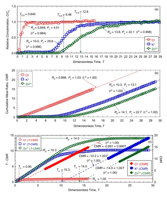
Figure 5.43. Chemical transport analyses for determination of column Péclet number ( $P_L$ ) and/or retardation factor ( $R_d$ ) for backfill amended with 5 % clinoptilolite and permeated with 17.5 mM KCl plus 10 mM ZnCl<sub>2</sub> (Test No. 8): (a) regression of relative concentration (RC) data; (b) regression of cumulative mass ratio (CMR) data; (c)  $T_o$  (=  $R_d$ ) and T - CMR analyses for  $R_d$ .
