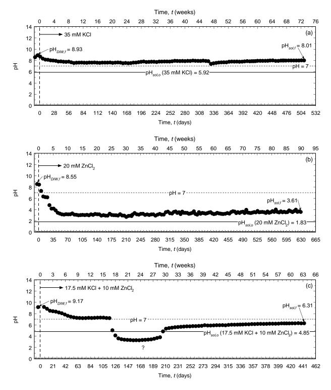
Figure 5.32. Temporal trends in the pH of the effluent from columns of backfills amended with 5 % chabazite-UB permeated with different salt solutions: (a) 35 mM KCl (Test No. 3); (b) 20 mM ZnCl<sub>2</sub> (Test No. 4); (c) 17.5 mM KCl plus 10 mM ZnCl<sub>2</sub> (Test No. 5).
