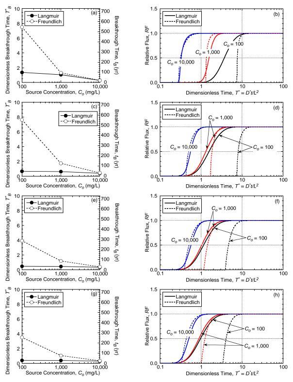
Figure 4.18. Effect of constant zinc source concentration ( $C_o$ ) on the dimensionless barrier breakthrough times,  $T_B^*$  (a, c, e) for f = 0.05 and flux breakthrough curves (b, d, f) for unamended and zeolite-amended backfills: (a) & (b) unamended; (c) & (d) 5 % chabazite-LB-amended; (e) & (f) 5 % chabazite-UB-amended; (g) & (h) 5 % clinoptilolite-amended.
