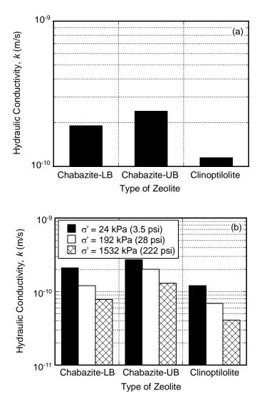
Figure 2.12. Effect of the same amount (5 %) of different zeolites on the hydraulic conductivity, k, of zeolite-amended backfills: (a) geometric mean of k values measured using flexible-wall cells at an average consolidation effective stress,  $\sigma'$ , of 34.5 kPa (5.0 psi); (b) k values measured in fixed-ring oedometer cells at different values of  $\sigma'$ .
