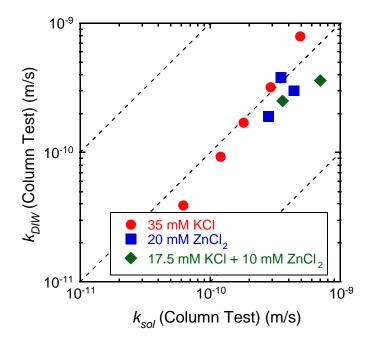
Figure 5.14. Comparison of the measured hydraulic conductivity based on column test,  $k_{DIW}$  versus  $k_{sol}$ .
