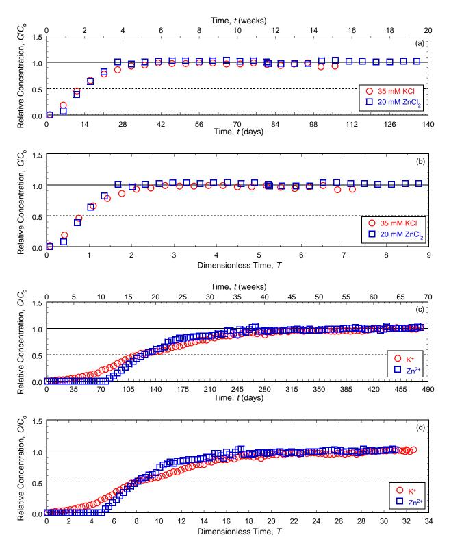
Figure 5.66. Breakthrough curves for backfill amended with 5 % clinoptilolite and permeated with 35 mM KCl or 20 mM ZnCl<sub>2</sub>: (a) chloride (Cl<sup>-</sup>) versus time (*t*); (b) Cl<sup>-</sup> versus dimensionless time (*T*); (c) potassium (K<sup>+</sup>) and zinc (Zn<sup>2+</sup>) versus *t*; (d) K<sup>+</sup> and Zn<sup>2+</sup> versus *T*.
