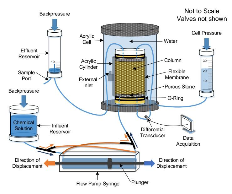
Figure 5.1. Schematic of testing apparatus.
