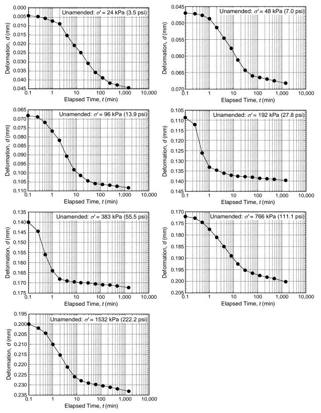
Figure A.5. Results of settlement as a function of log elapsed time for the unamended SB backfill.
