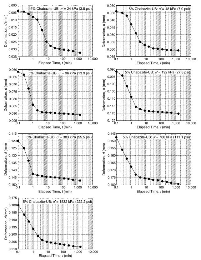
Figure A.13. Results of settlement as a function of log time for SB backfill amended with 5 % chabazite-UB.
