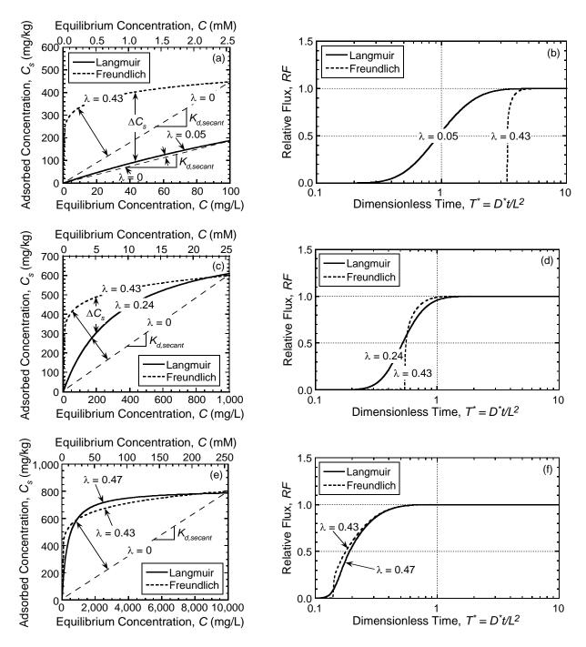
Figure 4.3. Effect of adsorption behavior on potassium flux breakthrough curves for unamended backfill based on different adsorption models (Langmuir and Freundlich): (a), (c), (e) adsorption behaviors for concentration ranges of 100, 1,000, and 10,000 mg/L, respectively; (b), (d), (f) flux breakthrough curves for a source concentration ( $C_o$ ) of 100, 1,000, and 10,000 mg/L, respectively.
