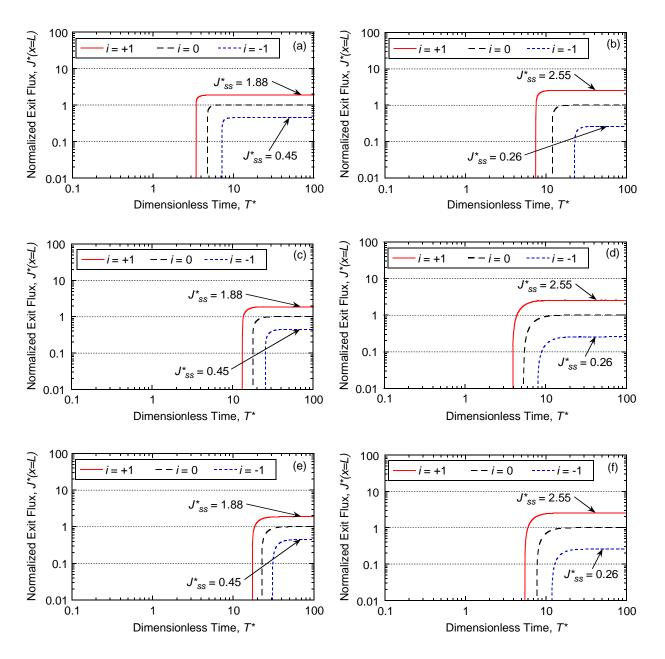
Figure E.7. Effect of Péclet number,  $P_L$ , on flux breakthrough curves with a constant source concentration,  $C_o = 100 \text{ mg/L}$  for: (a) unamended with potassium (K); (b) unamended with zinc (Zn); (c) amended with 5 % chabazite-UB with potassium (K); (d) amended with 5 % chabazite-UB with zinc (Zn); (e) amended with 10 % chabazite-UB with potassium (K); (f) amended with 10 % chabazite-UB with zinc (Zn), all based on the Freundlich adsorption model.
