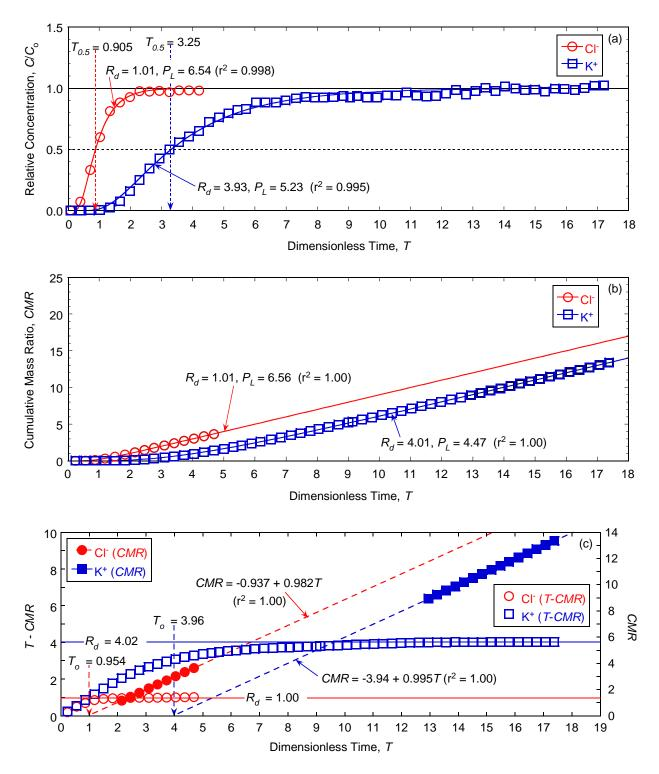
Figure 5.35. Chemical transport analyses for determination of column Péclet number ( $P_L$ ) and/or retardation factor ( $R_d$ ) for unamended backfill permeated with 35 mM KCl (Test No. 1): (a) regression of relative concentration (RC) data; (b) regression of cumulative mass ratio (CMR) data; (c)  $T_o$  (=  $R_d$ ) and T - CMR analyses for  $R_d$ .
