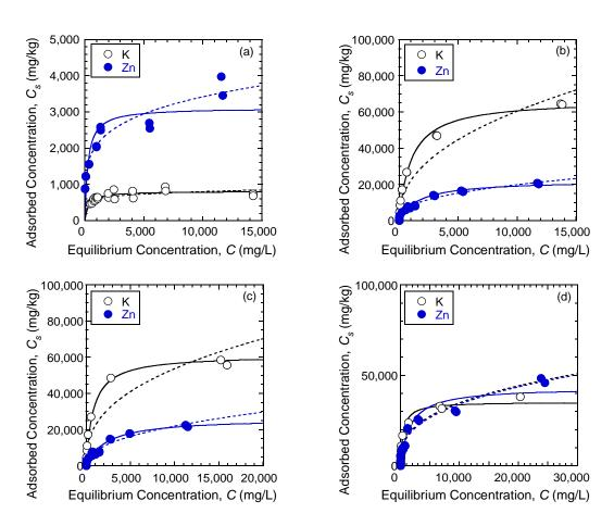
Figure 3.14. Comparison of potassium (K) versus zinc (Zn) adsorption including fitted Freundlich (dash lines) and Langmuir (solid lines) adsorption models: (a) unamended backfill sorbent; (b) 100 % chabazite-LB; (c) 100 % chabazite-UB; (d) 100 % clinoptilolite.
