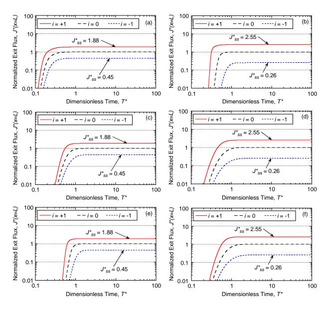
Figure E.18. Effect of Péclet number,  $P_L$ , on flux breakthrough curves with a constant source concentration,  $C_o = 10,000 \text{ mg/L}$  for: (a) unamended with potassium (K); (b) unamended with zinc (Zn); (c) amended with 5 % clinoptilolite with potassium (K); (d) amended with 5 % clinoptilolite with zinc (Zn); (e) amended with 10 % clinoptilolite with potassium (K); (f) amended with 10 % clinoptilolite with zinc (Zn), all based on the Langmuir adsorption model.
