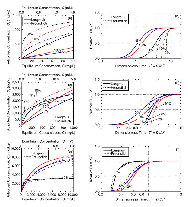
Figure 4.5. Effect of adsorption behavior on flux breakthrough curves for zinc based on different contents (0, 5, 10 %) of chabazite-UB and adsorption models (Langmuir and Freundlich): (a), (c), (e) adsorption behaviors over concentration ranges of 100, 1,000, and 10,000 mg/L, respectively; (b), (d), (f) flux breakthrough curves for a source concentration ( $C_o$ ) of 100, 1,000, and 10,000 mg/L, respectively.
