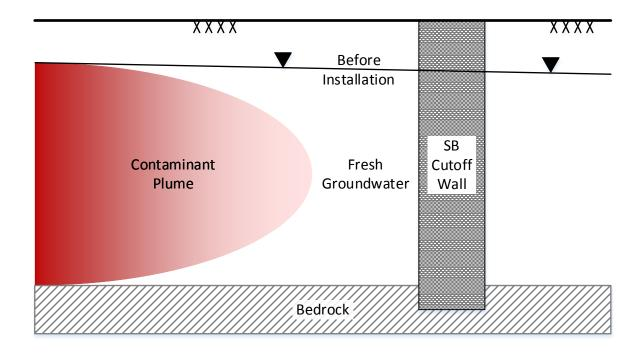
Figure 5.3. Schematic scenario for placement of soil-bentonite (SB) vertical cutoff wall down gradient from a migrating contaminant plume.
