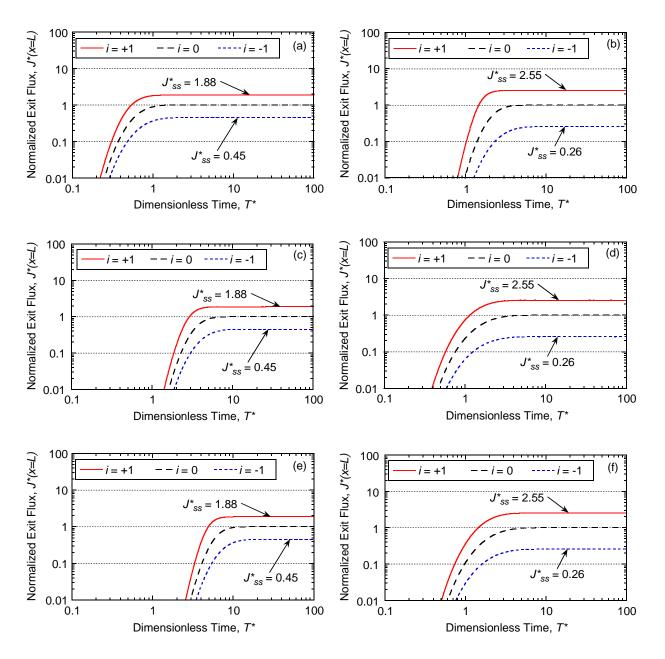
Figure E.5. Effect of Péclet number,  $P_L$ , on flux breakthrough curves with a constant source concentration,  $C_o = 1,000$  mg/L for: (a) unamended with potassium (K); (b) unamended with zinc (Zn); (c) amended with 5 % chabazite-LB with potassium (K); (d) amended with 5 % chabazite-LB with zinc (Zn); (e) amended with 10 % chabazite-LB with potassium (K); (f) amended with 10 % chabazite-LB with zinc (Zn), all based on the Langmuir adsorption model.
