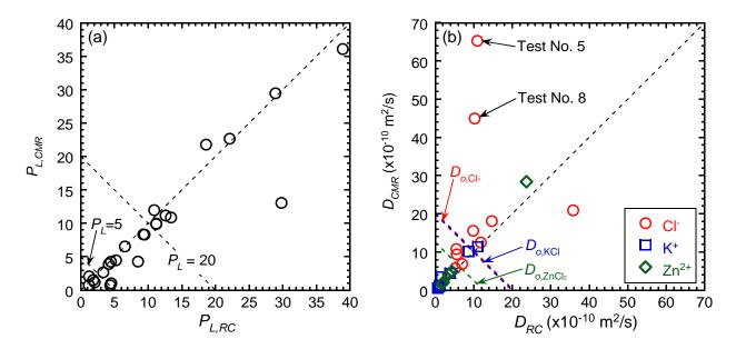
Figure 5.47. Comparison of the Péclet Number  $(P_L)$ , and dispersion coefficient (D) from relative concentration (RC) and cumulative mass ratio (CMR): (a)  $P_L$  from RC versus CMR; (b)  $R_d$  from RC versus steady-state CMR; (b) D from RC versus CMR.
