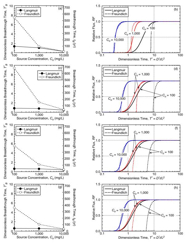
Figure 4.19. Effect of constant zinc source concentration ( $C_o$ ) on the dimensionless barrier breakthrough times,  $T_B^*$  (a, c, e) for f = 0.05 and flux breakthrough curves (b, d, f) for unamended and zeolite-amended backfills: (a) & (b) unamended; (c) & (d) 10 % chabazite-LB-amended; (e) & (f) 10 % chabazite-UB-amended; (g) & (h) 10 % clinoptilolite-amended.
