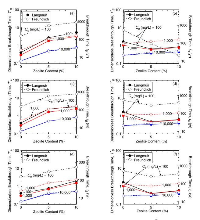
Figure 4.8. Effect of the zeolite content on barrier flux breakthrough times,  $T_B^*$  and  $t_B$ , based on f of 0.05 and source concentration ( $C_o$ ) of 100, 1,000, 10,000 mg/L for potassium (a, c, e) or zinc (b, d, f): (a) & (b) chabazite-LB; (c) & (d) chabazite-UB; (e) & (f) clinoptilolite.
