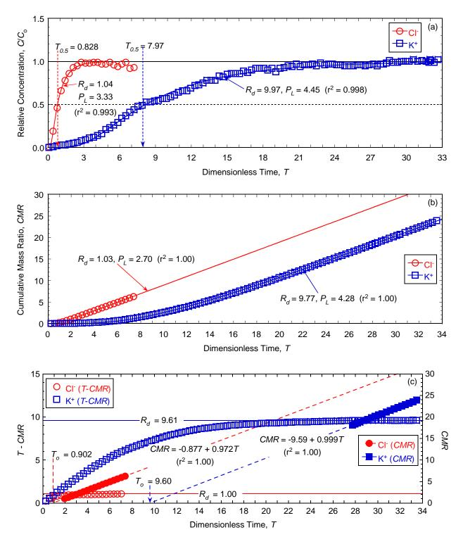
Figure 5.41. Chemical transport analyses for determination of column Péclet number ( $P_L$ ) and/or retardation factor ( $R_d$ ) for backfill amended with 5 % clinoptilolite and permeated with 35 mM KCl (Test No. 6): (a) regression of relative concentration (RC) data; (b) regression of cumulative mass ratio (*CMR*) data; (c)  $T_o$  (=  $R_d$ ) and T - CMR analyses for  $R_d$ .
