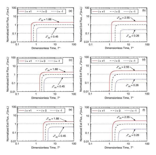
Figure E.14. Effect of Péclet number,  $P_L$ , on flux breakthrough curves with a constant source concentration,  $C_o = 1,000$  mg/L for: (a) unamended with potassium (K); (b) unamended with zinc (Zn); (c) amended with 5 % clinoptilolite with potassium (K); (d) amended with 5 % clinoptilolite with zinc (Zn); (e) amended with 10 % clinoptilolite with potassium (K); (f) amended with 10 % clinoptilolite with zinc (Zn), all based on the Freundlich adsorption model.
