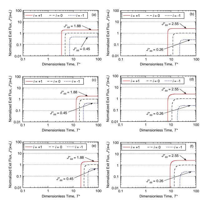
Figure E.1. Effect of Péclet number,  $P_L$ , on flux breakthrough curves with a constant source concentration,  $C_o = 100 \text{ mg/L}$  for: (a) unamended with potassium (K); (b) unamended with zinc (Zn); (c) amended with 5 % chabazite-LB with potassium (K); (d) amended with 5 % chabazite-LB with zinc (Zn); (e) amended with 10 % chabazite-LB with potassium (K); (f) amended with 10 % chabazite-LB with zinc (Zn), all based on the Freundlich adsorption model.
