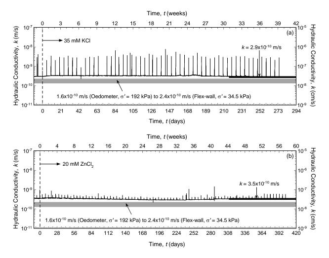
Figure 5.10. Temporal trends in hydraulic conductivity for columns of unamended backfills permeated with different salt solutions: (a) 35 mM KCl (Test No. 1); (b) 20 mM ZnCl<sub>2</sub> (Test No. 2).
