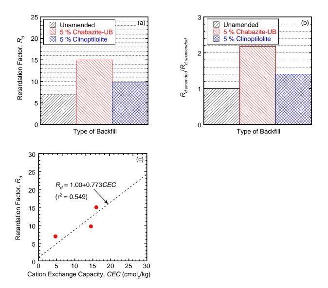
Figure 5.57. Effect of type of zeolite on retardation of zinc  $(Zn^{2+})$  for columns of unamended and zeolite-amended backfills permeated with 20 mM ZnCl<sub>2</sub>: (a) retardation factor  $(R_d)$ ; (b) ratio of  $R_d$  for the zeolite-amended backfill relative to  $R_d$  for the unamended backfill  $(R_{d,amended}/R_{d,unamended})$ ; (c) cation exchange capacity (*CEC*) of backfill and  $R_d$  of Zn<sup>2+</sup>.
