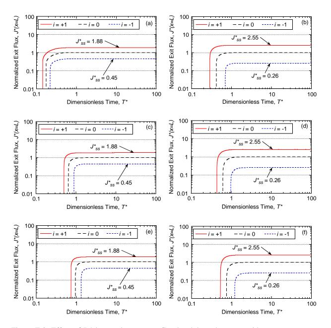
Figure E.3. Effect of Péclet number,  $P_L$ , on flux breakthrough curves with a constant source concentration,  $C_o = 10,000 \text{ mg/L}$  for: (a) unamended with potassium (K); (b) unamended with zinc (Zn); (c) amended with 5 % chabazite-LB with potassium (K); (d) amended with 5 % chabazite-LB with zinc (Zn); (e) amended with 10 % chabazite-LB with potassium (K); (f) amended with 10 % chabazite-LB with zinc (Zn), all based on the Freundlich adsorption model.
