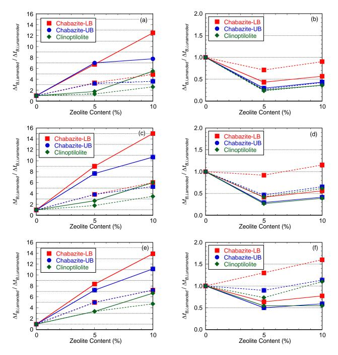
Figure 4.15. Relative effect of zeolite amendment on the incremental change in barrier flux breakthrough time due to a reversal in hydraulic gradient,  $\Delta t_{B,i,amended}/\Delta t_{B,i,unamended}$ , as a function of zeolite content: (a), (c), (e) potassium source concentration ( $C_o$ ) of 100, 1,000, and 10,000 mg/L, respectively; (b), (d), (f) zinc  $C_o$  of 100, 1,000, and 10,000 mg/L respectively. Note: solid line = Langmuir adsorption model; dashed line = Freundlich adsorption model.
