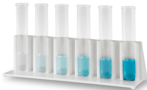
Figure 1.7. Qualitube for Microcystin Detection. Source: Envirologix
