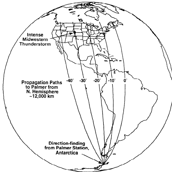
Figure 2. ELF/VLF broadband recordings are made at Palmer Station, Antarctica ( 64^{\circ}46'S , 64^{\circ}03'W ), at a range of \sim 12,000 km from the Nebraska and Iowa storms studied. Most of the Americas, the Atlantic and Pacific Oceans, Africa, and parts of Europe have smaller ranges to Palmer than the storms reported in this paper.
