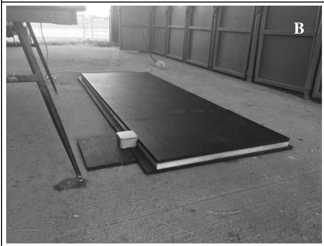
Figure 3.2 Images of the embedded-optical-base system (EOBS). Image A shows EOBS with initial column and row grid layout for first round testing. Image B shows EOBS without grid layout. The EOBS platform measured 0.914 m (width) x 2.438 m (length).
