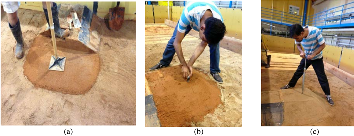
Figure 3. Preparation of model embankments for spill-through abutments: (a) compaction; (b) torsional-vane test of cohesive soil; and (c) needle penetrometer test
