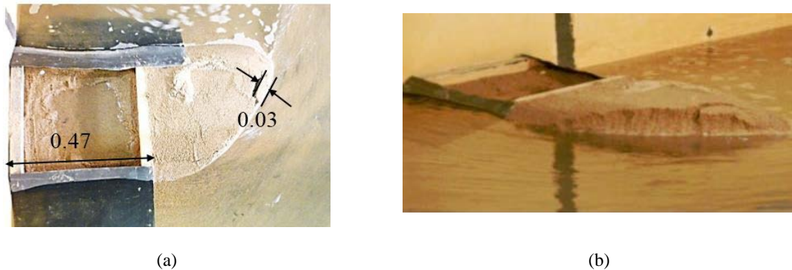
Figure 7. Erosion of a non-cohesive (sand) embankment: (a) the formation of a tension crack; and (b) eventual detachment of a block from the face of the embankment (dimensions in meters). Note that surface tension gives sand a modicum of cohesion for this small-scale experiment.
