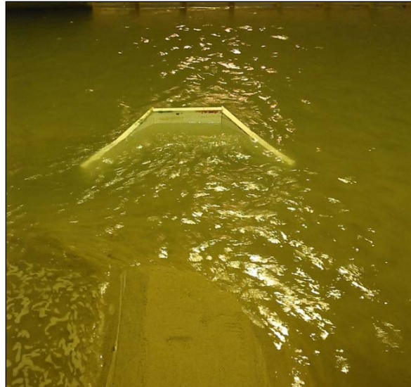
Figure 1. Breach development in a non-cohesive embankment in a lab model (1:30-scale) of a wingwall abutment (Ettema et al. 2010). Bridge abutments typically are wingwall or spill-through forms. Bridge abutments that end with vertical walls and side wings are called “wingwall abutments”; bridge abutments that end in spill-slopes (where the sideslope form extends around the abutment, are called “spill-through abutments.” Most of the experiments in this paper involved spill-through abutments.
