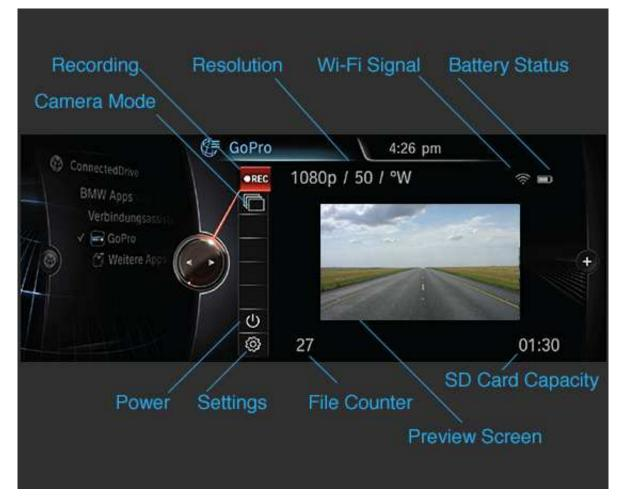
FIGURE 2.11. GoPro Remote User Interface-2 (reprinted from [7])
