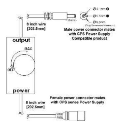
FIGURE 2.24. LDP 2-A LED dimmer (reprinted from [10])
