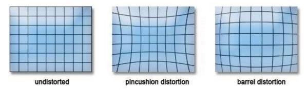
FIGURE 2.12. Types of Image Distortions (reprinted from [8])
