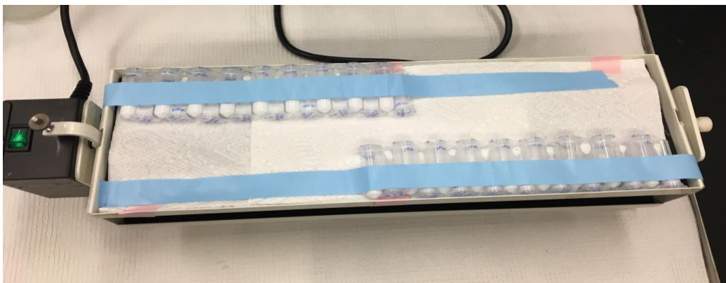
Figure 12. Samples agitated using using a Thermo Scientific Labquake shaker with a fixed speed.
