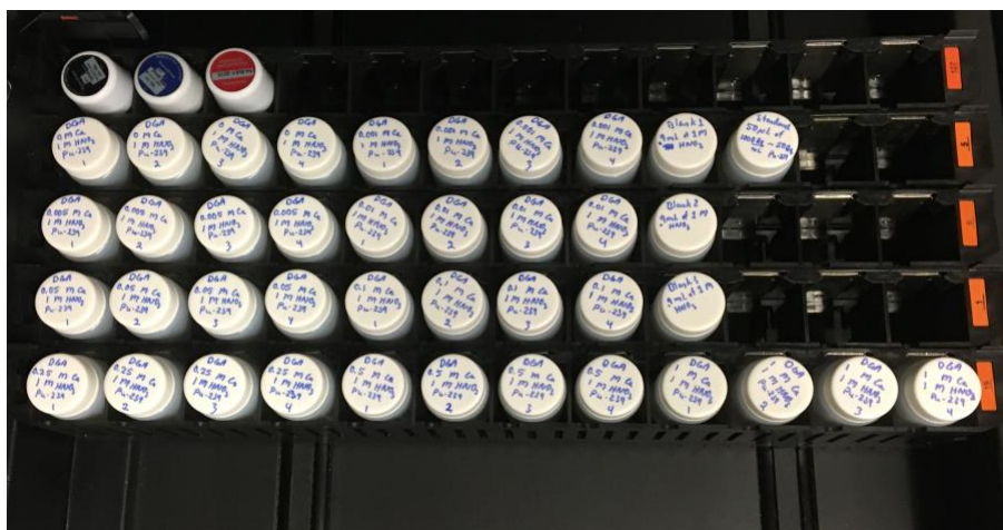
Figure 14. Samples counted with Perkin Elmer Model Tri-Carb 5110TR liquid scintillation counter and analyzed using QuantaSmart™ Software.
