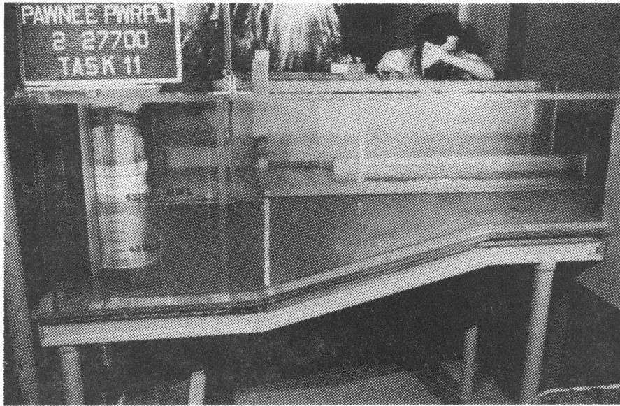
Figure 8. Pump Operation in a Modified Sump with Baffle Plates, Curtain Walls and Divider Wall in Place
