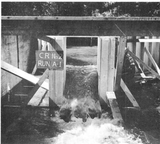
C. Upstream view of Run A-1 Discharge 11.7 cfs
