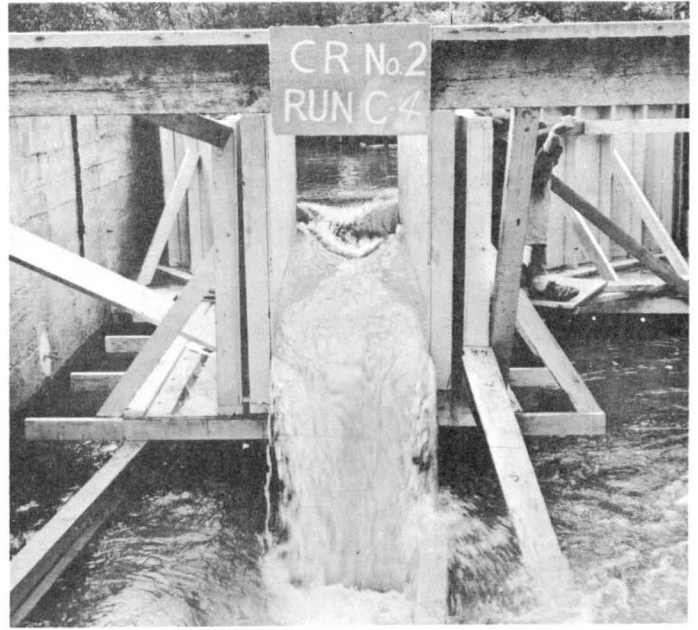
B. Upstream view of Run C-4 Discharge 9.42 cfs
