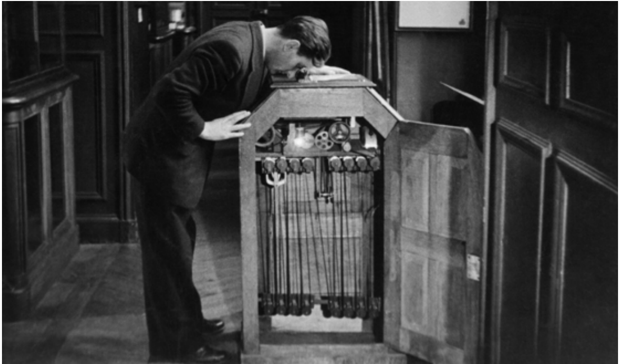
Figure 11. Kinetoscope with open side door revealing the film and mechanisms. 37
