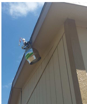
Figure 2.2: Canister affixed to the roof line of a mobile classroom on the elementary school campus.
