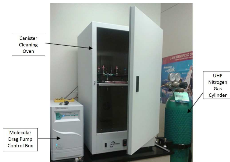
Figure 2.9: Photo of the Entech Instruments 3100D Canister Cleaning System used to clean and evacuate the 6L Silonite ® -coated canisters.
