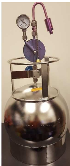
Figure 2.8: Photo of the Flow Controller attached to the 6L Silonite ® -coated canister, prepared for field deployment.
