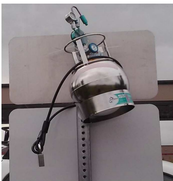
Figure 2.4: Canister affixed to an exit sign north of the gas station pumps.
