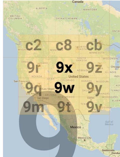
Figure 3.7. Determining intersecting Geohash values to direct the spatial query to the destination nodes
