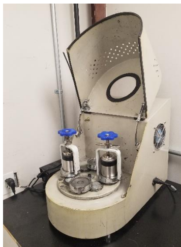
Figure 2.3: Planetary ball mill and milling jars used for mechanical milling of stainless steel chips.
