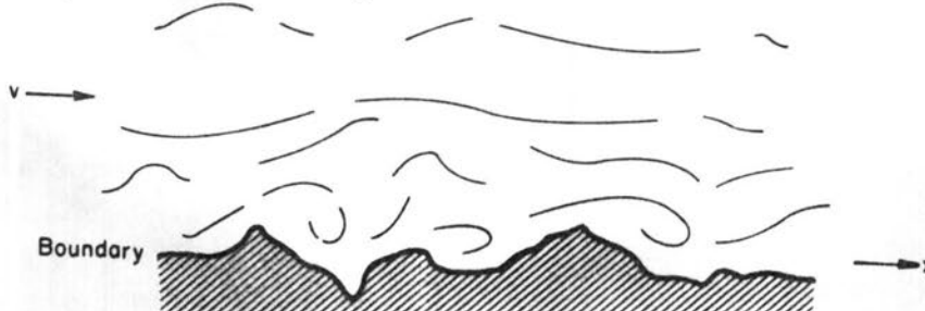
Fig. 2.3.3 Hydraulically rough boundary
