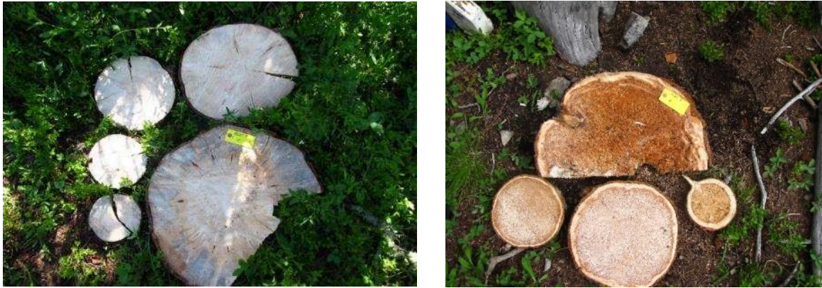
Figure 2.5- Seasoning checks (left) and heart rot (right). Photo Credit: Jim Webb
