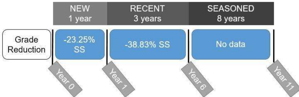
Figure 5.2 - Percent Select Structural reduction with increasing TSD class. Changes indicated use year zero as a base.
