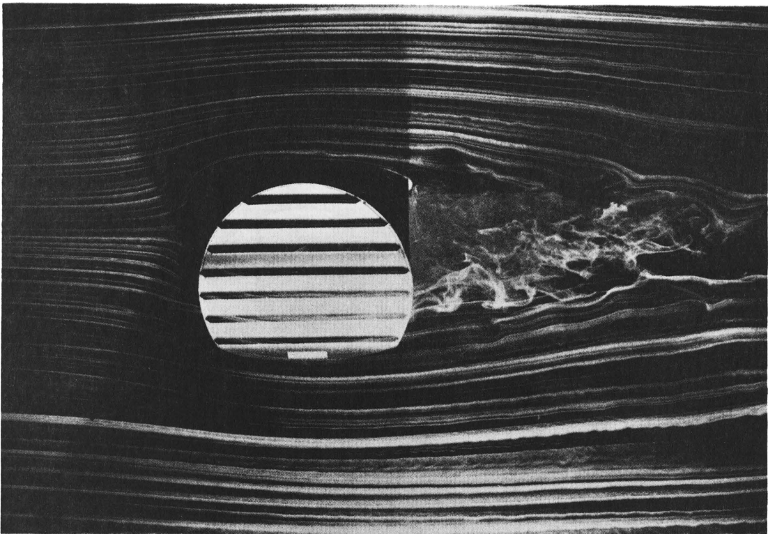
Figure 44a. Flow Around the Conical Horn Antenna - GABRIEL UHR10 D
