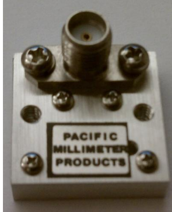
Figure 3.6: 130 GHz zero bias waveguide detector with negative voltage output.
