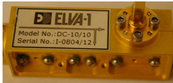
Figure 2.4: W-band ELVA 10 dB directional coupler.
