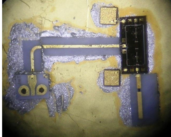
Figure 2.7: Measurement test configuration for M/A-COM PIN-diode switch.
