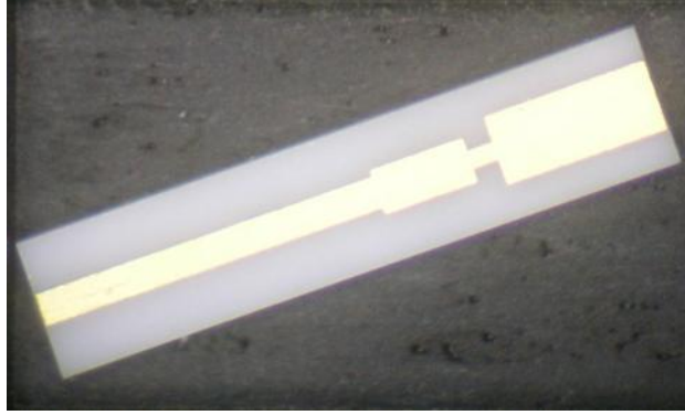
Figure 2.12: 92 GHz waveguide-to-microstrip transition.
