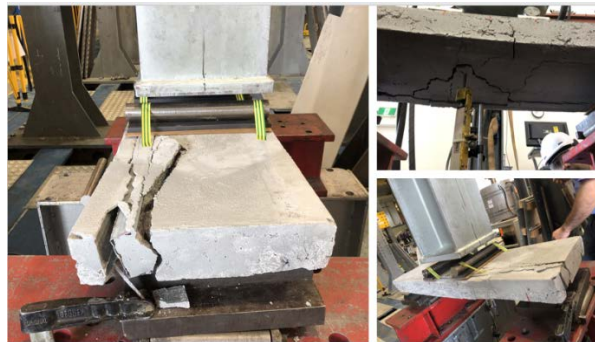
Fig. 10. Failure modes of prefabricated wall panels with cold-form steel studs
