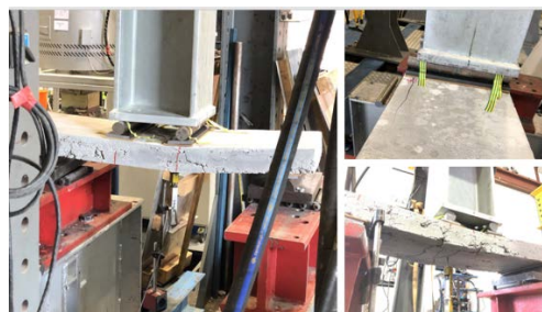
Fig. 12. Failure modes of prefabricated wall panels with two slotted steel angles
