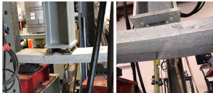
Fig. 14. Failure modes of prefabricated wall panels with three slotted steel angles
