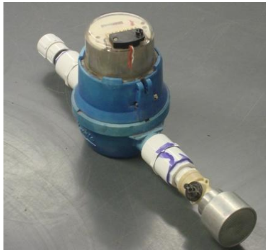
Figure 1.2: Watering breaker with attached flow meter
