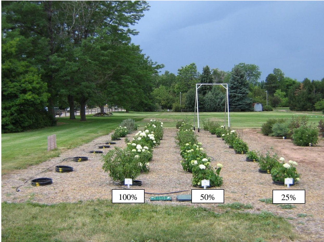
Figure 2.7: Lysimeter component of the study containing the three watering treatments based on ET_o looking west (July 21, 2010)
