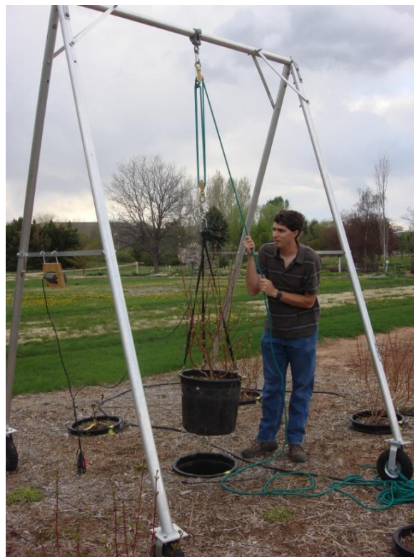
Figure 2.2: Lysimeter A-frame used for weighing each pot in the study
