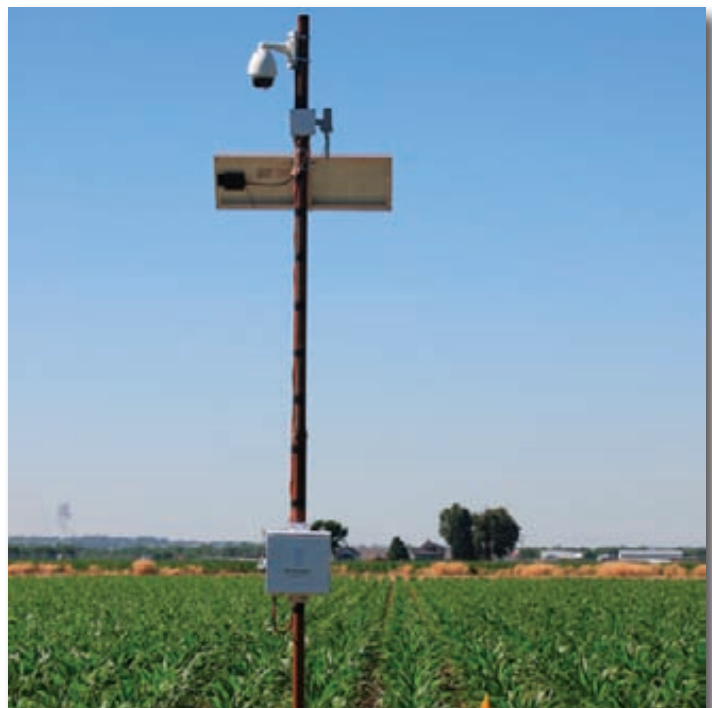
Part of the instrumentation on the Regenesys research farm includes an internet-accessed camera that records plantwater stress at multiple times during the day.
