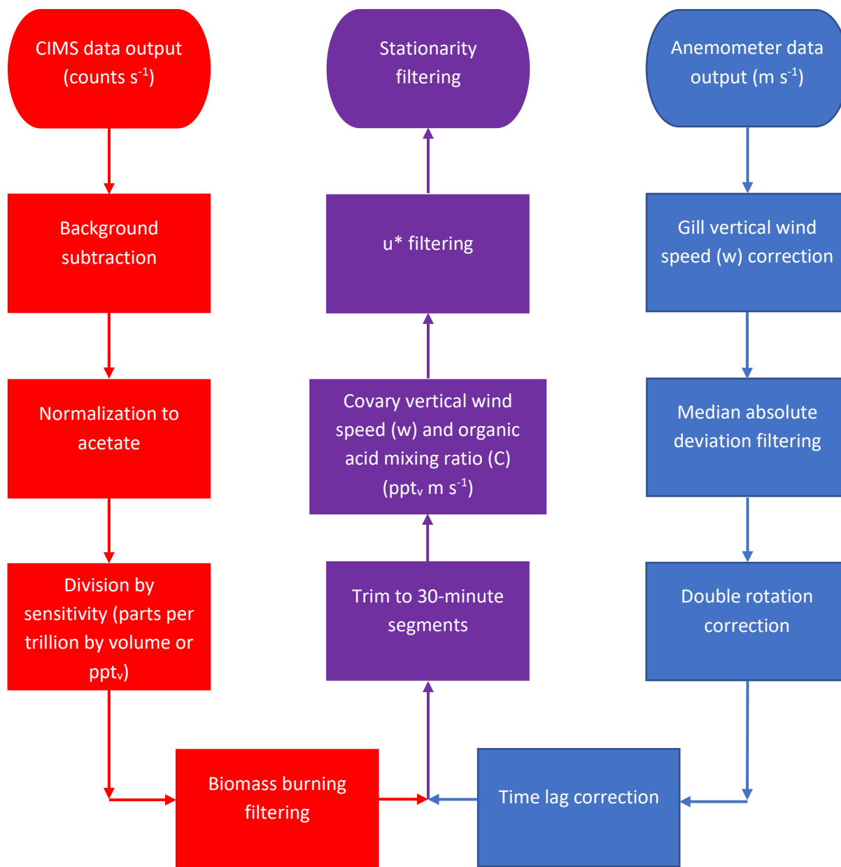
Figure A1.15. Flow chart lists the data processing steps taken to transform chemical ionization mass spectrometer (CIMS) data (red) for organic acids and three-dimensional sonic anemometer data (blue) for vertical wind speed ( w ) into vertical flux data (purple) by the eddy covariance technique ( \overline{w'C'} ).
