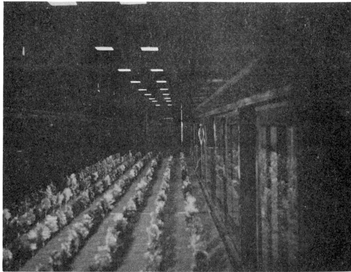
Figure 3.21 The arrangement of artificial trees in the model forest, 0.254 m tree spacing
