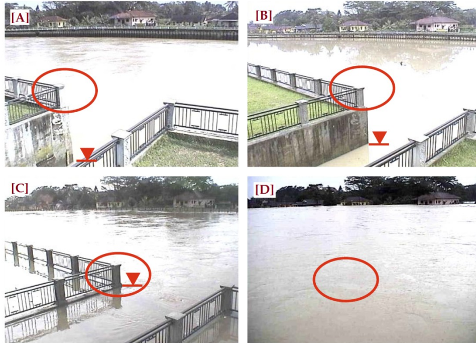
Figure 6.4 Water level indicators [A] On Dec. 18, 2006 - 14:56, [B] On Dec. 19, 2006 - 08:01 [C] On Dec. 20, 2006 - 08:01 and [D] On Dec. 21, 2006 - 08:16 (after Shafie 2009)
