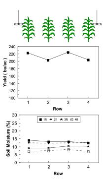
Figure 5a. Corn yield and soil water content for sprinkler devices spaced 9 ft. apart at 7 ft height.
