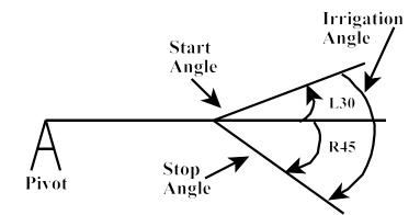
Figure 3. Part circle sprinklers angles. Angles are between 0 -180 degrees with an L or R prefix.
