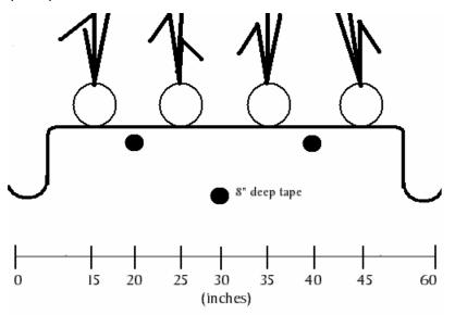
**Figure 1:** Comparison of drip line placement for onion production; the standard single line placed 8 inches deep in the center of the bed and the more efficient configuration of two lines placed at a shallower depth.
