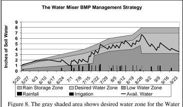
Figure 8. The gray shaded area shows desired water zone for the Water Miser BMP strategy. The black line showing available water should stay in the gray shaded area to indicate planned moisture level for the crop. Rain may push the line into the rain storage zone.
