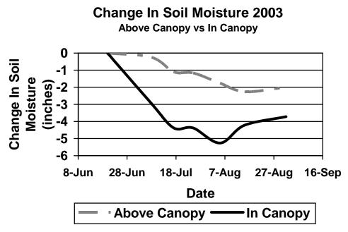
Figure 1. Change in soil moisture (from initial values) during the 2003 growing season for above canopy and in-canopy placement of sprinklers.
