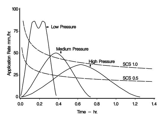
Figure 2 Example application rate curve versus 0.5 and 1.0 SCS intake curve.
