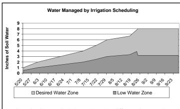
Figure 3. The gray shaded area shows the difference between the soils water holding capacity in the root zone and the maximum allowed soil moisture deficit.
