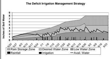
Figure 9. The gray shaded area shows desired water zone for the Deficit Irrigation strategy. The black line showing available water should stay in the gray shaded area to indicate planned moisture level for the crop. Rain may push the line into the rain storage zone.
