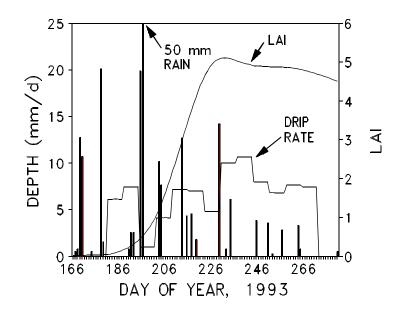
**Figure 1.** Depth of rainfall (25 mm is 1 inch) and drip irrigation for each day of the corn growing season. Also plotted is the crop leaf area index, which peaked in mid August. A 2-inch (50-mm) rain goes off the plot scale.
