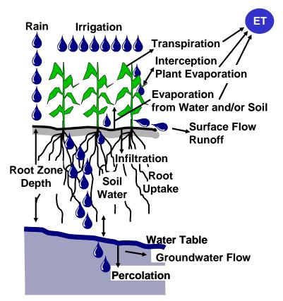
Figure 2. Illustration of various water transport components needed to characterize irrigation efficiency.
