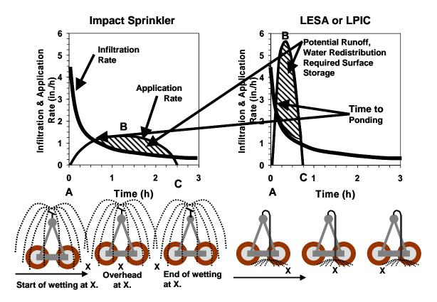
Figure 3. Illustration of runoff or surface water redistribution potential for impact sprinkler and spray (LESA or LPIC) center application packages for an example soil. (A) represents the start of the irrigation, (B) is the peak application rate (usually when the system is directly overhead), and (C) is the completion of the irrigation. The first intersection point of the infiltration curve and the application rate curve represents the first ponding on the soil surface.
