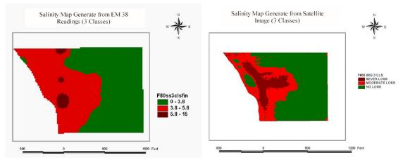
Figure 4. Soil salinity map generated from field data vs. map generated from satellite image.
