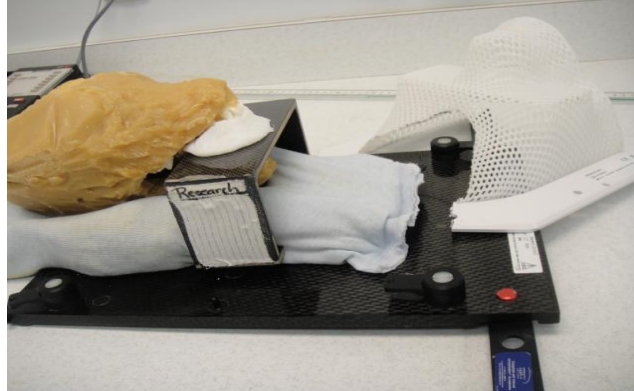
Fig 2.3A Cranial immobilization system used for the phantom composed of (mask, bite block, bridge, cushion, and baseplate)
