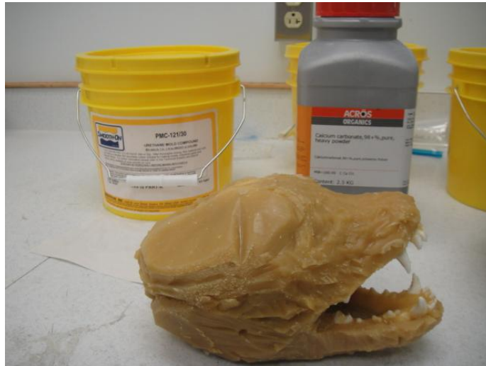
Figure 2.1 Canine head phantom constructed from canine skull and STES (rubber, urethane and calcium carbonate)
