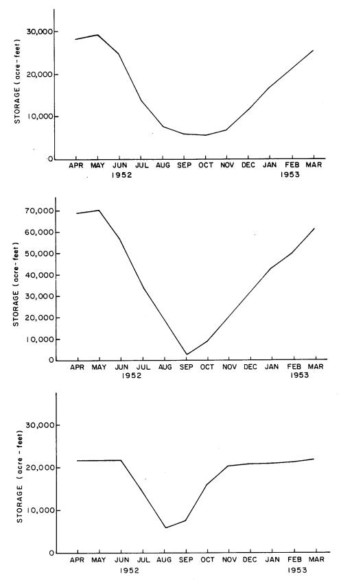
Figure 3-5. Typical cycles of filling and drawing water over and annual cycle for three reservoirs: (a) Prewitt, (b) North Sterling, and (c) Julesburg. Adapted from Labadie, et al. (1983).
