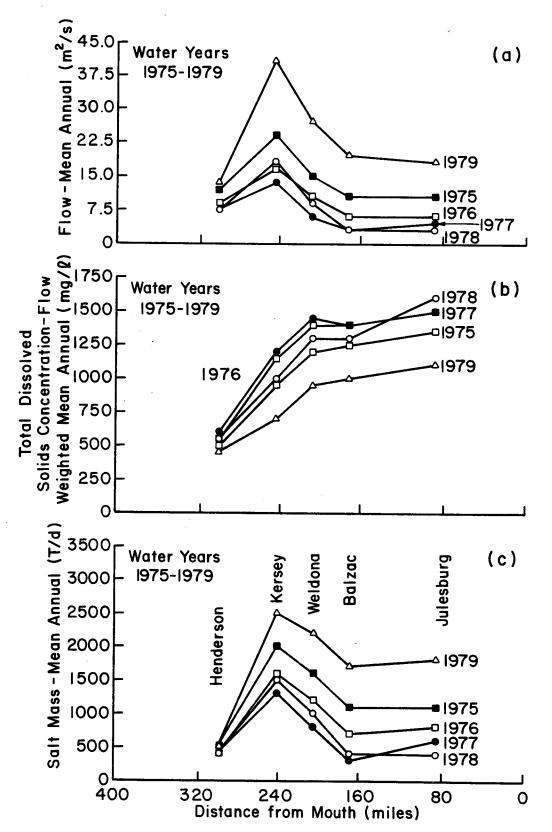
Figure 3-9. Distance profiles of flow, total dissolved solids, and salt mass flow from Henderson to Julesburg, 1975-79 (from Gomez-Ferrer and Hendricks, 1982).
