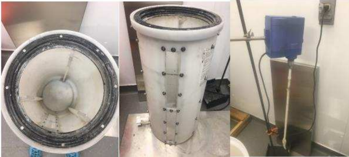
Figure 25- 20-gallon baffled Nalgene tank and standing mixer used for optimized phosphorus recovery process
