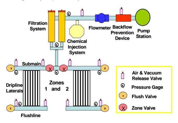
Figure 1. Schematic of Subsurface Drip Irrigation (SDI) System. (Components are not to scale) K-State Research and Extension Bulletin MF-2576, Subsurface Drip Irrigation (SDI) Component: Minimum Requirements
