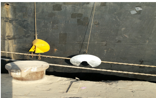
Figure 3. Improper use of rat guard at seaport
