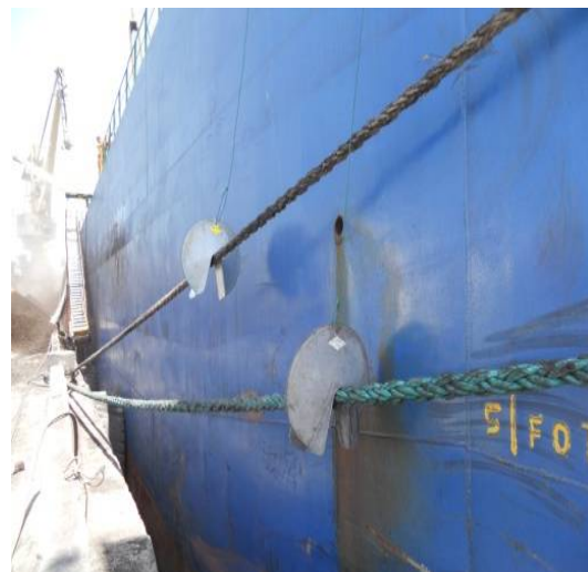
Figure 6. Rodent guard without locking system
