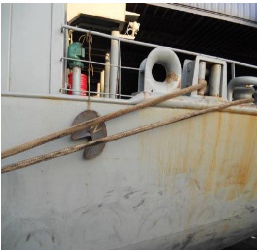
Figure 5. Rodent guard not in position
