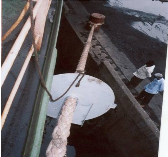
Figure 3. Rodent guard in mooring rope
