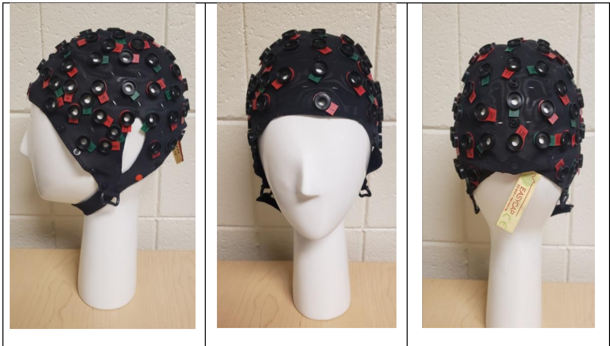
Figure 1. Side view, frontal view, and posterior view of EasyCap (cap montage M15) specialized recording cap (Easycap GmbH, Germany) without NIRx spring-loaded grommets
