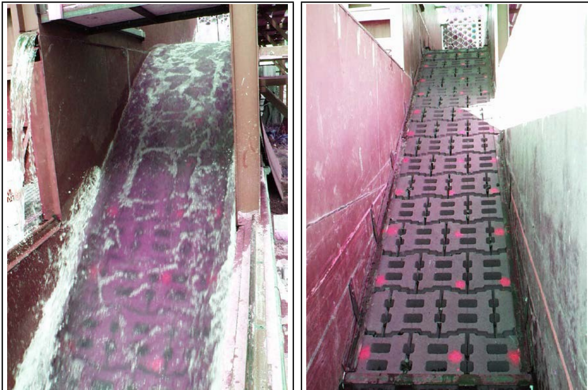
Figure 1. Full-Scale Laboratory Testing of ACB Systems at Colorado State University (Photos by Armortec)
