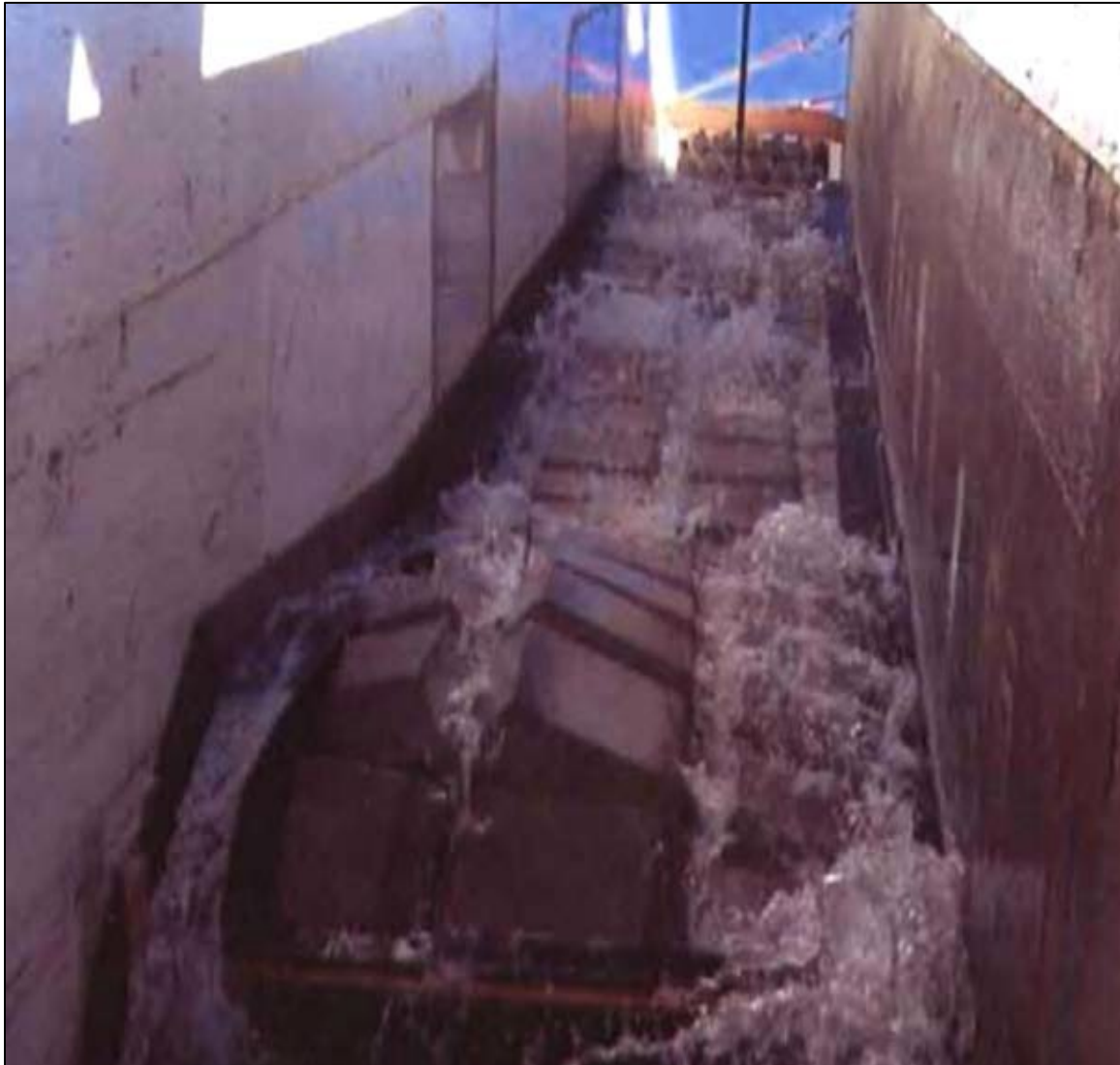
Figure 13. Photograph Showing Laboratory Testing of an ACB System that Failed after 8 Minutes of Testing Under 1-foot of Overtopping (Photo looking upstream).
