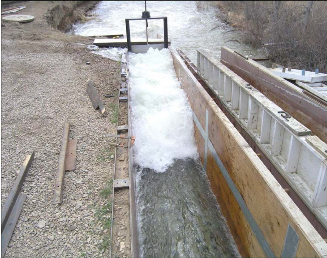
Figure 2. Full-Scale Test of Hydraulic Jump on ACBs in CSU Flume (Photo Courtesy of Chris Thornton)
