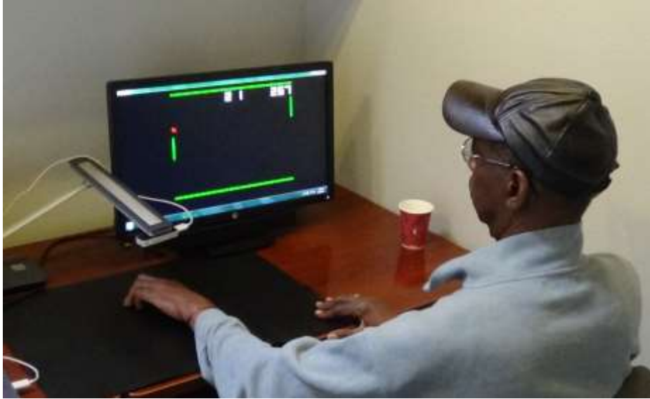
Fig. 9 Picture of system setup for participants who used their affected, left upper extremity (R4, R5, R7, R8). A 23" monitor was placed at subject's midline. The Leap Motion Controller ©2015 was affixed to the pictured stand, positioned approximately 8" above the table, and directed to capture hand movement on the black table mat pictured. The black table mat was positioned at the same height for all subjects as all desks used were of the same height.
