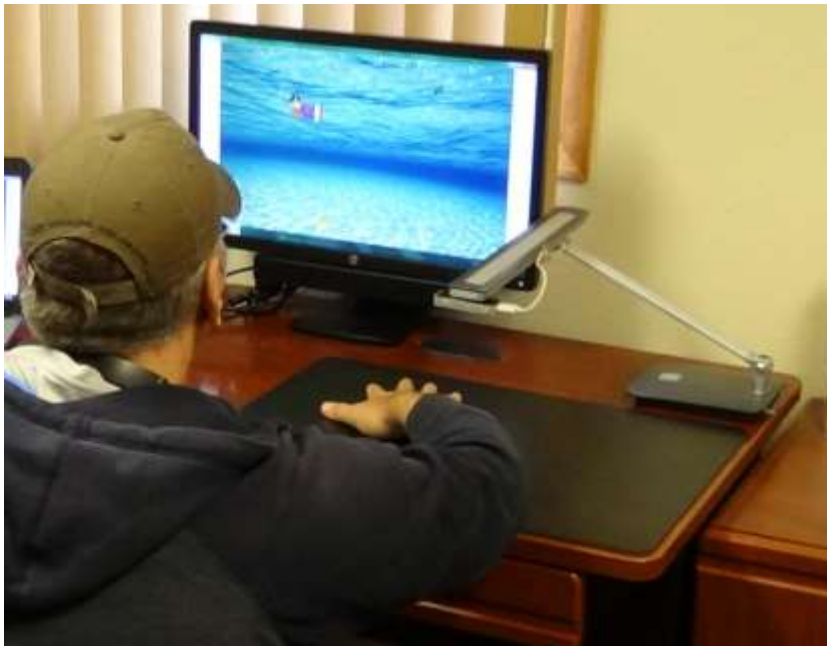
Fig. 10 Picture of system setup for participants who used their non-affected, right upper extremity (R1, R2, R3, R6). A 23" monitor was placed at subject's midline. The Leap Motion Controller ©2015 was affixed to the pictured stand, positioned approximately 8" above the table, and directed to capture hand movement on the black table mat pictured. The black table mat was positioned at the same height for all subjects as all desks used were of the same height.
