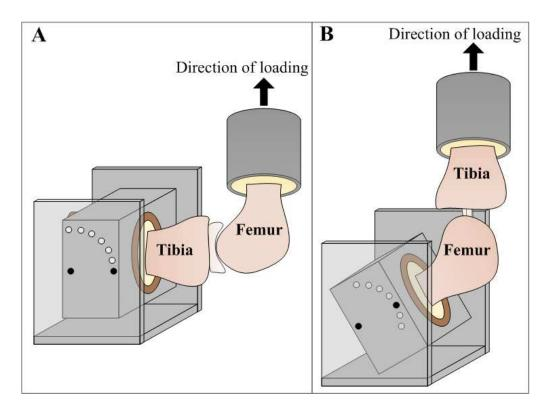
Figure 4.2: Mechanical testing setup for simulated anterior drawer test (A), and stress relaxation and pull to failure tests (B).
