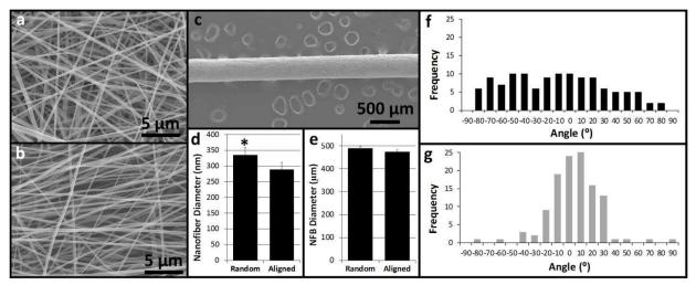
Figure 2.1: Nanofiber sheets with random (a) and aligned (b) nanofibers were used to fabricate nanofiber bundles (c). The diameters of nanofibers which compose random and aligned nanofiber sheets are significantly different (d, \* indicates p < 0.05) however the diameter of random and aligned nanofiber bundles (NFB) are not significantly different e). Randomly oriented nanofiber sheets have a wider spread of nanofiber angles (f) compared to aligned nanofiber sheets (g).
