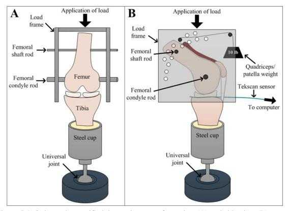
Figure 5.4: Ovine cadaver stifle joint testing setup front view (A) and side view (B).
