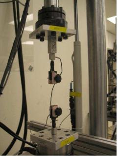
7. Setup the camera stand on the MTS and attach the Flea3 camera. The camera should be ~1ft away from the thin film grips. Adjust the height of the camera stand so that the top of the lower thin film grip is just visible at the bottom of the camera image. Note that if the camera is positioned as shown in figure X the recording will be upside down.
