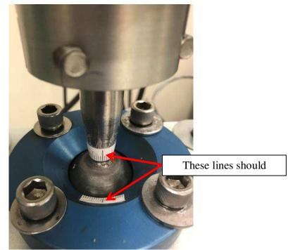
iii. On the cardboard potting tube make a vertical mark with a marker. Note the position of the mark at each angle using the ruler on the cup. This position should be the same any other testing with the joint (such as in the destabilized condition).
