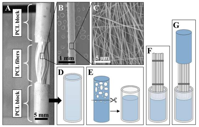
Figure 4.1: Electrospun scaffold (A), individual nanofiber bundle (B) and electrospun nanofibers (C). Silicone tubing with solvent cast PCL (D), solidified PCL with voids cut off and remainder inserted into silicone tubing (E), nanofiber bundles inserted into solvent cast PCL (F), and PCL block technique repeated on other end of nanofiber bundles (G).
