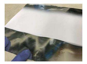
3. When the nanofiber bundle is  $\sim 0.5$  mm in diameter use a scalpel to slice close to the rolled edge.
