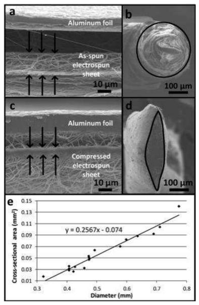
Figure 2.2: Transverse section of as-spun nanofiber sheet (a) nanofiber bundle (b). Transverse section of compressed nanofiber sheet (c) and nanofiber bundle (d). Linear relationship between measured nanofiber bundle diameter and compressed cross-sectional area (e).
