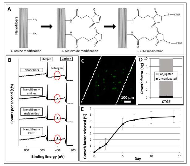
Figure 3.2: Chemical conjugation procedure (A), XPS survey spectra showing increasing nitrogen peak (B), immunofluorescence staining of conjugated CTGF (C), amount of CTGF conjugated (D), and CTGF release over a 14 day period (E).
