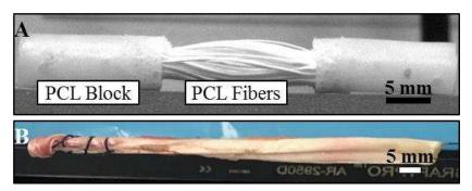
Figure 5.1: Electrospun scaffold (A) and LDE tendon soft tissue graft (B) prior to
