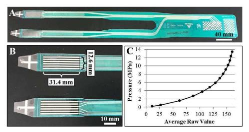
Figure 5.2: Tekscan 4041 sensor (A) and sensing area (B). Calibration curve (C).
