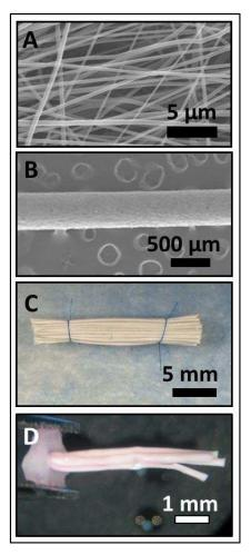
Figure 3.1: Aligned nanofibers (A), nanofiber bundle (B), scaffold composed of ~20 nanofiber bundles (C), and small scaffold composed of 4 nanofiber bundles (D).
